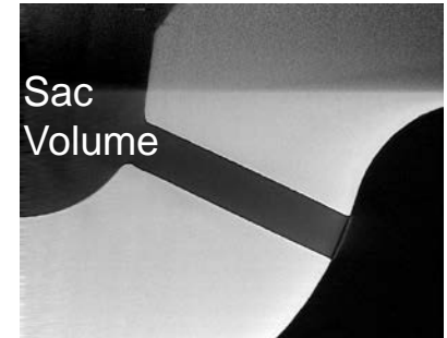
*X-ray image of new CAT injector tip (Powell et al.)
