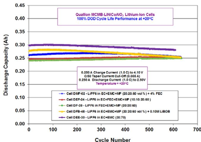
**Figure IV - 171:** Cycle life performance of 0.25Ah MCMB-LiNiCoAlO<sub>2</sub> cells (Quallion, LCC) containing various electrolytes at 20°C, using C rate charge and discharge over a voltage range of 2.50V to 4.10V.
