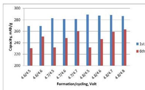
**Figure IV - 9:** Discharge capacity after 1st and 6th cycles under various testing conditions.
