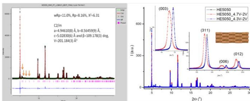
**Figure IV - 20:** (left) HR-SXRD pattern of HE5050 shows the super-reflections (020), (110), (11-1), (021), etc. due to the presence of Li/M ordering and associated monoclinic phase (C2/m). (right) HR-SXRD patterns of HE5050, HE5050\_4.3V-2V\_1 cycle, and HE5050\_4.7V-2V\_1 cycle. The inset drawing shows a possible interconnected layered structure for the heterogeneous structure after the activation.
