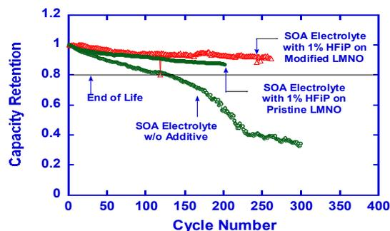
**Figure IV - 158:** Capacity as a function of cycle number plots at room temperature LMNO half cells in 1 m LiPF<sub>6</sub>/EC:EMC (30:70) with HFiP. Baseline electrolyte was also used as benchmark.
