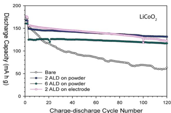
Figure IV - 59: Cycling performance for ALD alumina coated samples of LiCoO<sub>2</sub> cycled between 3.3V and 4.5V.
