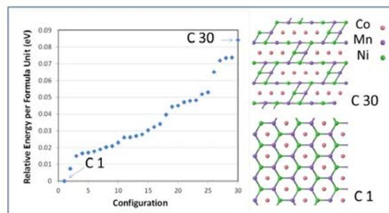
Figure IV - 13: DFT results for relative energies of thirty configurations of  $\text{Li}(\text{Ni}_{1/3}\text{Mn}_{1/3}\text{Co}_{1/3})\text{O}_2$ . The lowest energy configuration is the ordered arrangement C1. The partially segregated arrangement of C30, with NiMn zigzags interrupted by lines of Co, is still low enough in energy to be present at elevated temperatures.
