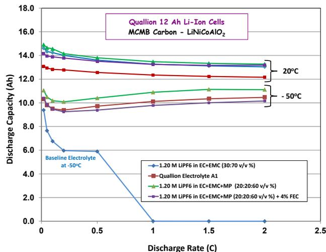
**Figure IV - 166:** Discharge rate capability of 12 Ah MCMB-LiNiCoAlO<sub>2</sub> cells (Quallion, LCC) containing various electrolytes at  $+20^{\circ}\text{C}$  and  $-50^{\circ}\text{C}$  (See first figure, A).
