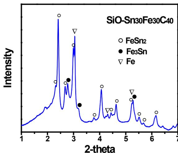
Figure IV - 100: XRD pattern of SiO-Sn<sub>30</sub>Fe<sub>30</sub>C<sub>40</sub>.
