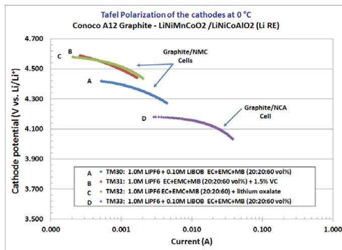
Figure IV - 173: Tafel polarization measurements at 0°C of three electrode cells consisting of Cononco A12 graphite/Toda HE 5050 LiNiCoMnO<sub>2</sub> or LiNiCoAlO<sub>2</sub> and containing various MB-based electrolytes.
