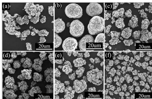
**Figure IV - 36:** SEM images of  $\text{Ni}_{0.25}\text{Mn}_{0.75}(\text{OH})_2$  secondary particles synthesized with different  $M_S/M_A$  in the base solutions (a) 0.667, (b) 1.5, (c) 1.8, (d) 2, (e) 2.5, (f) 4.
