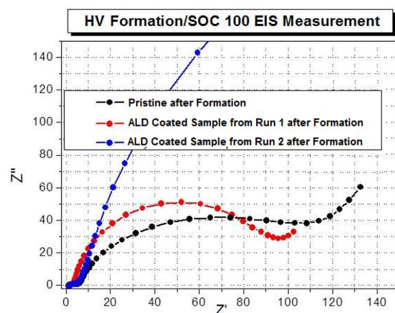
**Figure IV - 73:** EIS measurements on Mn-rich cathode material coated with different ALD layers of  $\text{Al}_2\text{O}_3$ : the powders coated in Run 2 show larger impedance build up compared to the baseline.
