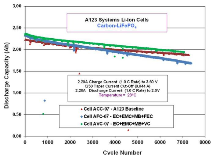
Figure IV - 164: Cycle life performance of LiFePO<sub>4</sub>-based A123 cells containing various electrolytes at +23°C.
