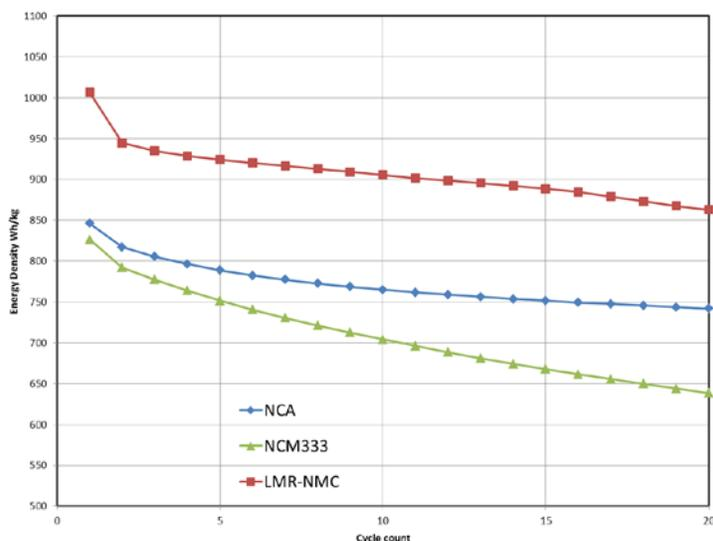
**Figure IV - 7:** Gravimetric energy densities during discharge plotted versus cycle number for LMR-NMC, NCA, and NCM. Voltage fade, along with capacity loss and cell resistance increase, lead to an overall loss in deliverable energy for a given amount of active oxide.
