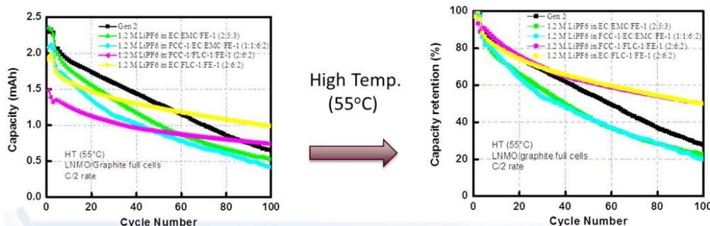
**Figure IV - 156:** LNMO/Graphite cell cycling profiles at 55°C(a) and the cycling performance using fluorinated electrolytes (b) Normalized capacity retention of fluorinated electrolyte and Gen2. Cycling rate is C/10, cutoff voltage is 3.5-4.9 V.
