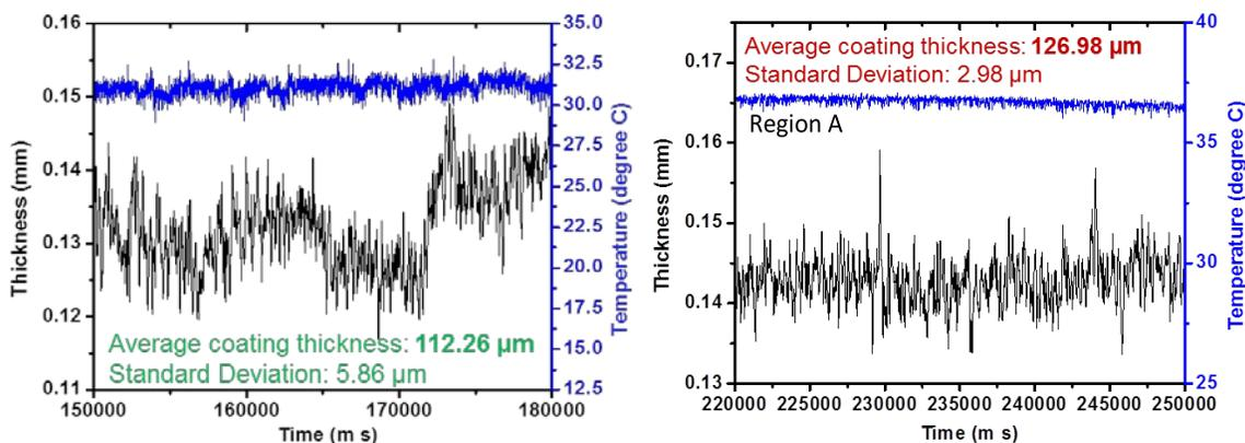
**Figure IV - 85:** In line thickness measurement of  $\text{LiNi}_{0.5}\text{Co}_{0.2}\text{Mn}_{0.3}\text{O}_2$  (NCM 523) electrode at different regions; the y-axis represents the temperature at which data were collected.
