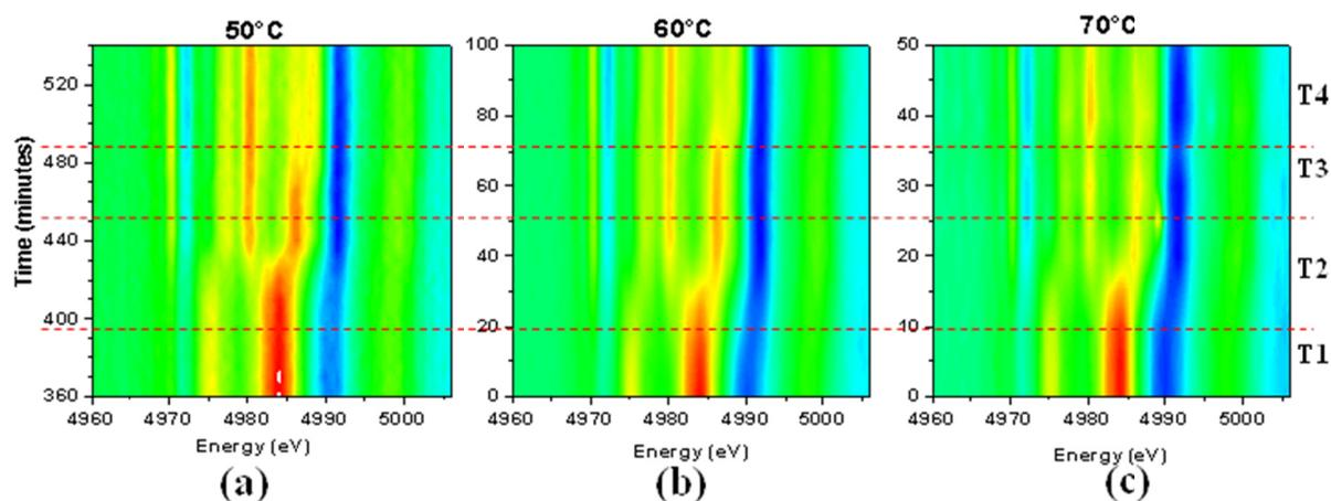
Figure IV - 107: Contour plots of the derivatives of the normalized energy for three temperature settings, (a) 50°C, (b) 60°C and (c) 70°C.
