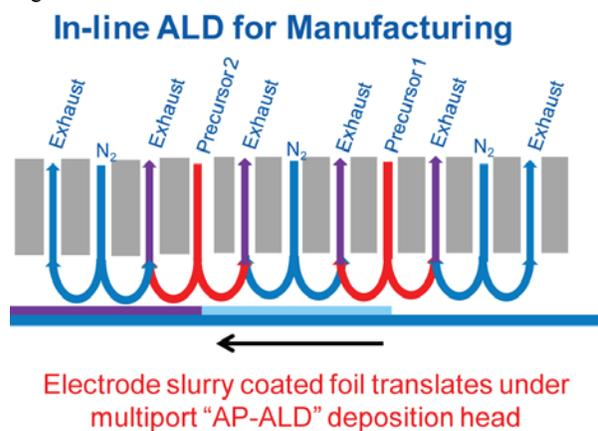
**Figure IV - 61:** A simplified schematic demonstrating the in-line spatial ALD concept.
