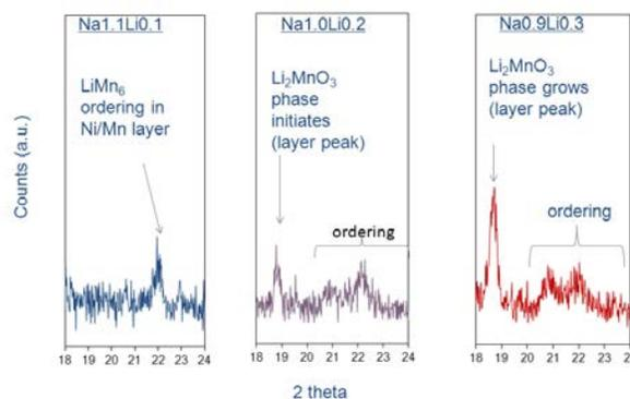
**Figure IV - 126:** X-ray powder diffraction patterns magnified between 18 and 24 degrees  $\text{CuK}\alpha$  2-theta of  $\text{Na}_a\text{Li}_b\text{Ni}_{0.25}\text{Mn}_{0.75}\text{O}_6$  precursor.
