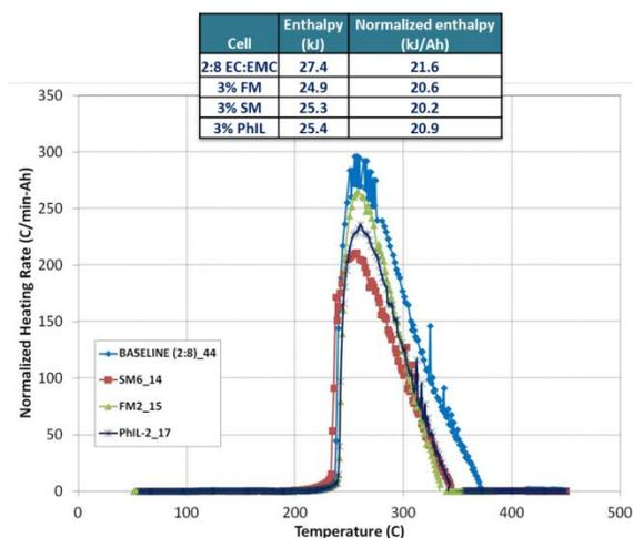
Figure IV - 225: ARC performance of INL synthesized phosphazene electrolytes.
