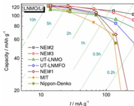
**Figure IV - 40:** Rate performance of  $\text{LiNi}_{1/2}\text{Mn}_{3/2}\text{O}_4$  materials.
