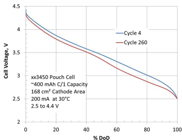
**Figure IV - 272:** Voltage profile change of ConocoPhillips A12 Graphite vs. Toda HE5050 (4<sup>th</sup> Cell Build).
