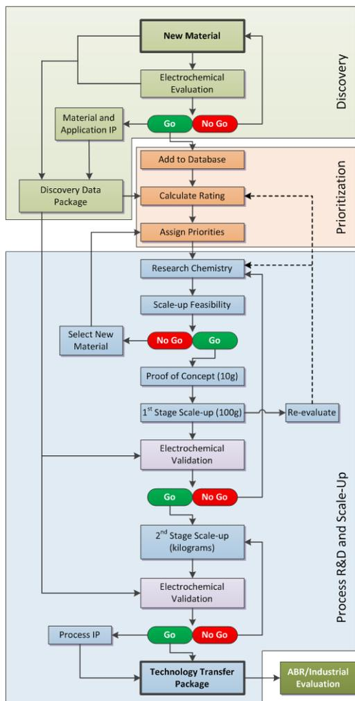
Figure IV - 249: Electrolyte Materials Process R&D Flowchart
