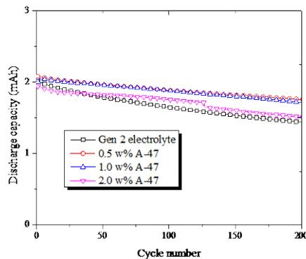
**Figure IV - 147:** Capacity retention of MCMB/NCM coin cells in 3E7EMC/PF12 with none or various amount of TPP (A-47). The cells were cycled at 55 °C. The charge rate was 1C. The cut-off voltages were 3~4 V.
