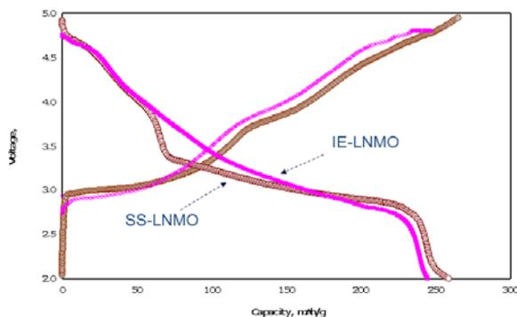
**Figure IV - 136:** Voltage profiles of direct synthesized  $\text{Li}_{1.2}\text{Ni}_{0.25}\text{Mn}_{0.75}\text{O}_y$  (SS-LNMO) and ion-exchange sample  $\text{Li}_{1.26}\text{Na}_{0.02}\text{Ni}_{0.25}\text{Mn}_{0.75}\text{O}_2$  (IE-LNMO). Current rate for both is  $15 \text{ mA g}^{-1}$
