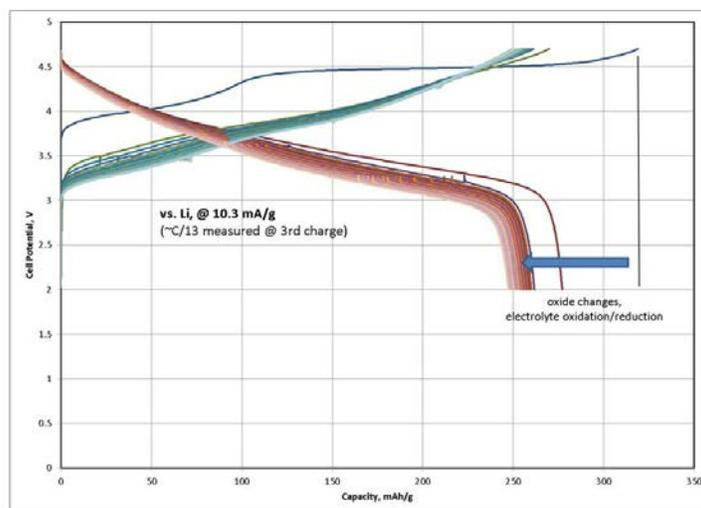
**Figure IV - 1:** Charge and discharge voltage profiles of the LMR-NMC 0.5Li<sub>2</sub>MnO<sub>3</sub>\*0.5LiMn<sub>0.375</sub>Ni<sub>0.375</sub>Co<sub>0.25</sub>O<sub>2</sub> cycled against metallic Li for 20 cycles. Various mechanisms have been identified to cause the apparent capacity fade.
