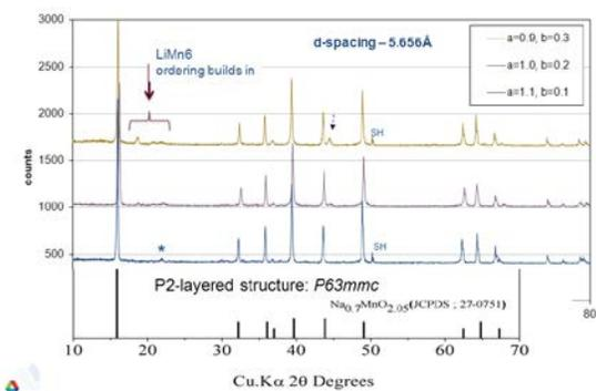
**Figure IV - 125:** X-ray powder diffraction patterns of  $\text{Na}_a\text{Li}_b\text{Ni}_{0.25}\text{Mn}_{0.75}\text{O}_6$  precursor. The asterisk indicates a superlattice peak, and the additional peaks in the top pattern indicate the formation of  $\text{LiMn}_6$  sites within the  $\text{Na}(\text{Li},\text{M})\text{O}_2$  structure.
