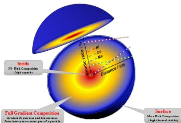
**Figure IV - 120:** Schematic diagram of the full concentration gradient lithium transition metal oxide particle with the nickel concentration decreasing from the center toward outer layer and the concentration of manganese increasing accordingly.
