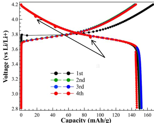
**Figure IV - 71:** Initial evaluation of Sample 2 coated with  $\text{Al}_2\text{O}_3$  in Run 1 using coin cells at NREL: Charge and Discharge at C/5 (25°C) with 1C-discharge pulses for 20s after every 10% discharge.
