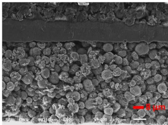
Figure IV - 243: Fractured cathode particles from calendaring from lot#2012-07-09&11.
