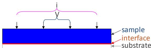
Figure IV - 55: Four point probe electrode conductivity geometry.
