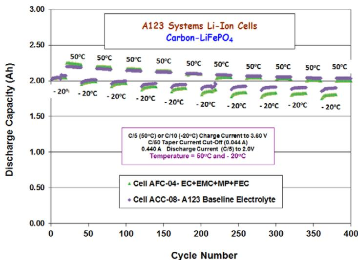
Figure IV - 165: Cycle life performance of LiFePO<sub>4</sub>-based A123 cells containing various electrolytes subjected to variable temperature cycling between +50°C and -20°C.
