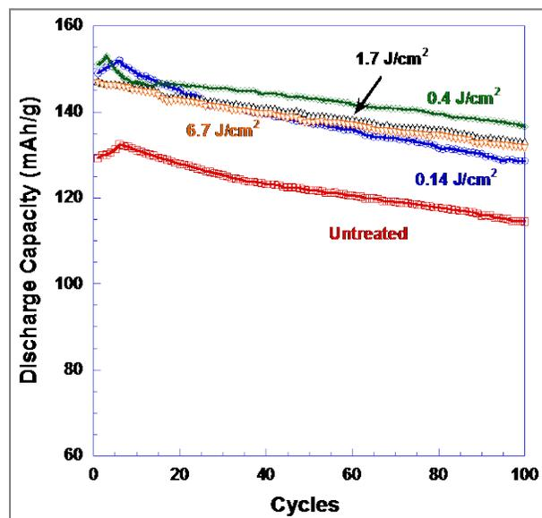
Figure IV - 75: Cycling of  $\text{LiFePO}_4$  cathodes at 0.5C/0.5C ( $0.34 \text{ mA/cm}^2$ ) confirming  $0.4 \text{ J/cm}^2$  as the best corona treatment energy density for long term performance.
