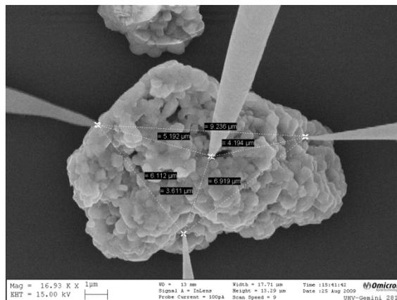
Figure IV - 52: Conductivity measurement using nano probe SEM.
