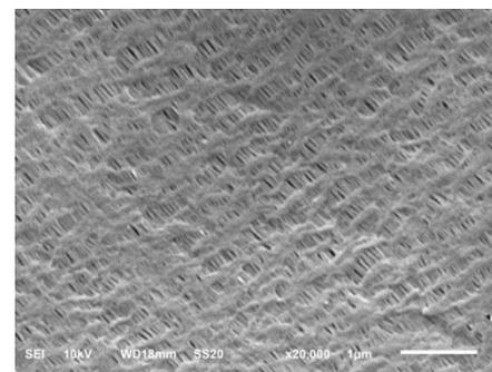
**Figure IV - 255:** SEM micrograph of Celgard separator before cycling.
