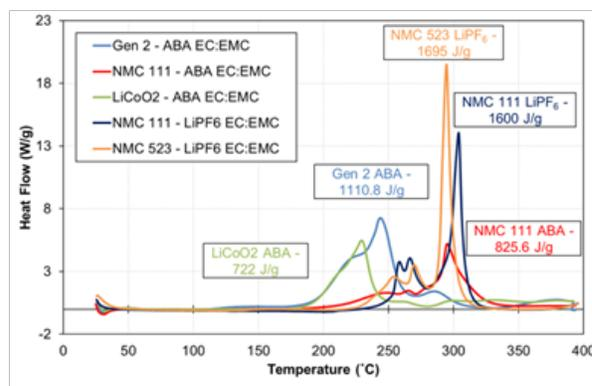
**Figure IV - 229:** Differential scanning calorimetry results for a variety of cathode materials with 1M ABA: 1M LiF electrolyte in EC:EMC solvent. For comparison, the DSC result for the same electrode material using 1.2 M LiPF<sub>6</sub> is also shown (dark blue).
