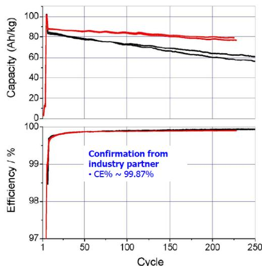
**Figure IV - 159:** Capacity as a function of cycle number plots at room temperature LMNO/A12 full Li ion cells in 1 m LiPF<sub>6</sub>/EC:EMC (30:70) with 5 mM HFiP. Baseline electrolyte was also used as benchmark.
