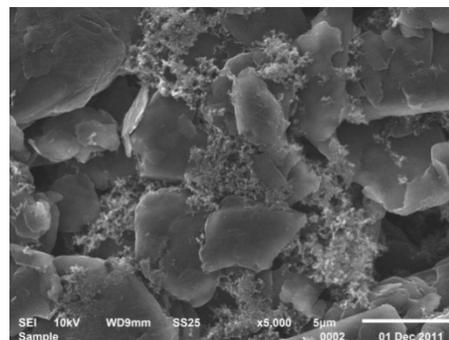
**Figure IV - 253:** SEM micrograph of a section of a pristine anode.
