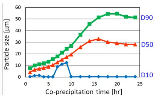
**Figure IV - 238:** Particle size distribution without growth control technology.
