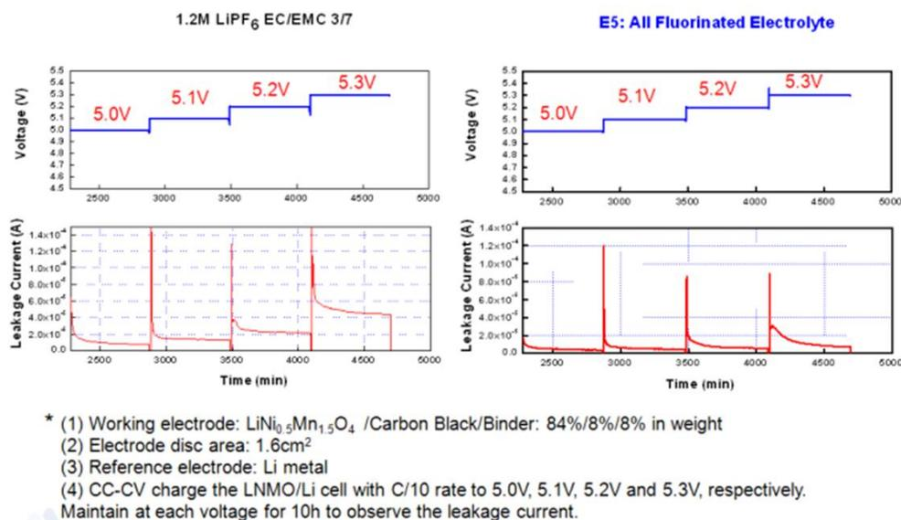
Figure IV - 153: Gen2 electrolyte and fluorinated electrolyte leakage currents at various potentials with LNMO/Li cell.
