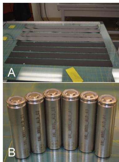
**Figure IV - 66:** (A) Samples of NMC 111 and A10 Graphite provided by Sandia NL and coated with ALD alumina by NREL/CU (B) 18650 cells fabricated from coated ALD foils for testing at Sandia.
