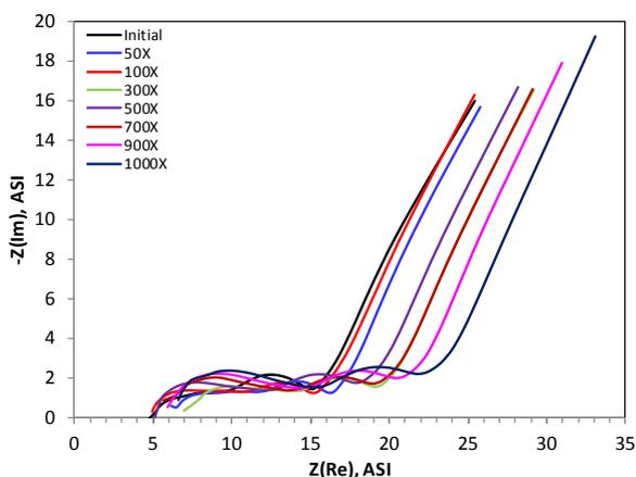
**Figure IV - 197:** EIS data from a  $\text{Li}_{1.2}\text{Ni}_{0.15}\text{Mn}_{0.55}\text{Co}_{0.1}\text{O}_2//\text{Graphite}$  cells containing the LiDFOB electrolyte additive.
