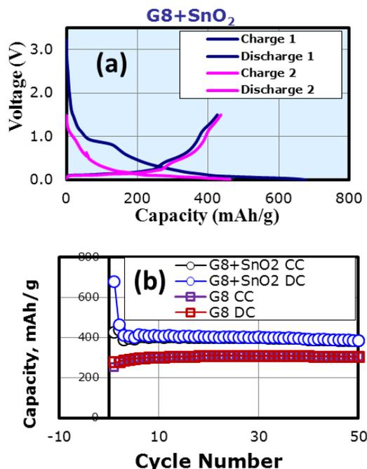
**Figure IV - 104:** (a) First and second discharge-charge-profiles of a lithium cell with a G8 graphite/25wt.% SnO<sub>2</sub> electrode, and (b) capacity vs. cycle number plot of a lithium half-cell with a SnO<sub>2</sub>-graphite electrode, cycled between 1.5 and 0.01 V at a C/4 rate (top), relative to a cell with a standard G8 graphite electrode (bottom).
