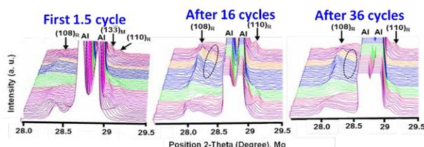
**Figure IV - 92:** (108), (110), (133) reflection during first 1.5 cycles, after 16 cycles, and after 36 cycles. The R and M subscripts designate the rhombohedral (trigonal) phase and monoclinic phase, respectively. The color stacks represents the different charge/discharge voltages. The appearance of new peaks is highlighted in the dotted regions.
