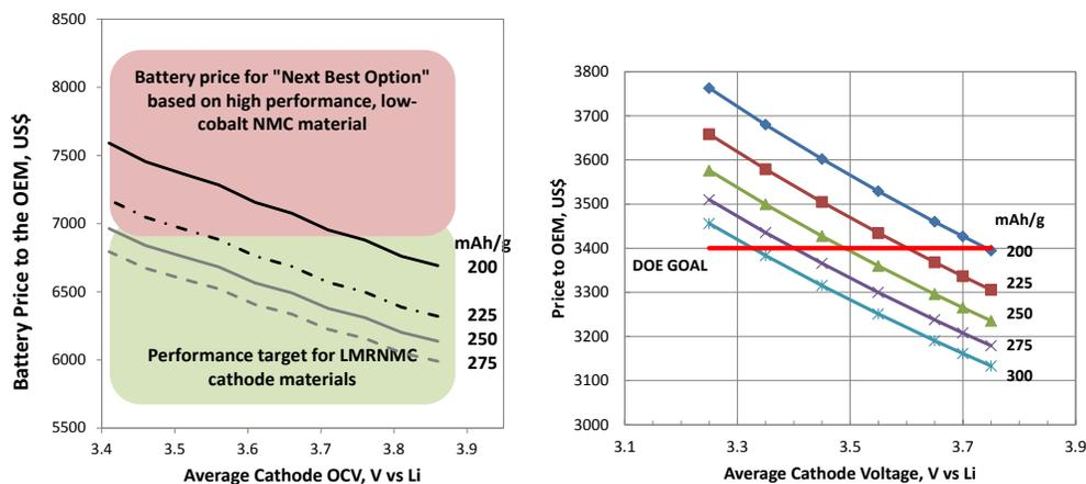
**Figure IV - 8:** Battery Price to OEM for an advanced Li-ion anode with LMR-NMC cathodes with varying capacities as a function of cathode OCV for (left) an EV150 compared against the next best Li-ion cathode option and (right) a PHEV40 compared against DOE goals.
