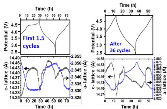
**Figure IV - 91:** Change in lattice parameter (with error bars) in Toda HE5050 cathode material at different points in the electrochemical charge/discharge profile; these plots were collected from the freshly prepared cell (first 1.5 cycles) and after 36 cycles.
