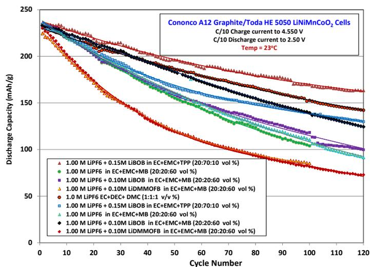
Figure IV - 172: Cycle life performance of Cononco A12 graphite/Toda HE 5050 LiNiCoMnO<sub>2</sub> cells containing containing various electrolytes (Fig. 2B).
