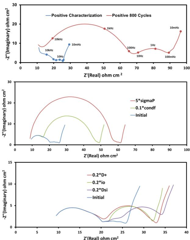
**Figure IV - 183:** (top) Experimental EIS measurements on Toda HE5050 LMR-NMC material before and after aging taken at an electrode voltage of 3.75 V and 30 °C (100 kHz-10 mHz). (middle) model parameter sensitivity analysis showing sensitivity to contact resistance and SEI film conductivity (bottom) model parameter sensitivity analysis for mid-frequency arc.
