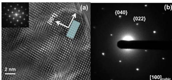
**Figure IV - 97:** High-resolution TEM image from the AH90 particle showing spinel like lattice fringes (see the simulated image of cubic spinel phase along [100] direction; the FFT and SAED shows spinel phase reflections).
