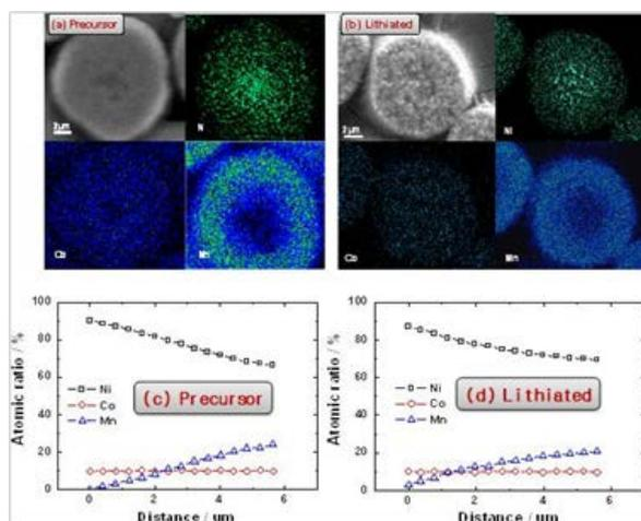
**Figure IV - 121:** Scanning electron microscopy images and electron-probe X-ray micro-analyzer mapping of (a) a precursor particle and (b) a lithiated particle; and integrated atomic ratio of transition metals as a function of the distance from the center of the particle for (c) the precursor and (d) the lithiated material.
