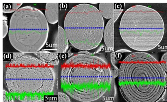
**Figure IV - 46:** EDXS curves superimposed on SEM images of bisected precursors with particle sizes of (a) <20  $\mu\text{m}$  (b) 20-38  $\mu\text{m}$ , and (c) 38-75  $\mu\text{m}$  and cathode materials with particle sizes of (d) <20  $\mu\text{m}$  (e) 20-38  $\mu\text{m}$ , and (f) 38-75  $\mu\text{m}$ .
