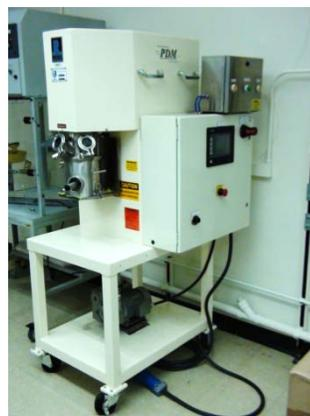
**Figure IV - 265:** High energy/shear planetary mixer from Ross with a 2 liter chamber capacity.
