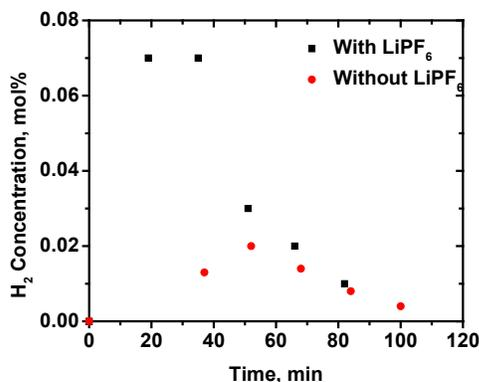
**Figure IV - 105:** Hydrogen concentration change with reaction time measured by *in situ* GC. The supporting Ar flow rate is 14 mL/min. Black squares represent condition with LiPF<sub>6</sub> in the electrolyte; red circles, no LiPF<sub>6</sub> in the electrolyte.
