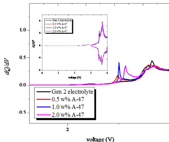
**Figure IV - 146:** Diff. Capacity vs voltage MCMB/NCM coin cells in 3E7EMC/PF12 with none or various amount of TPP (A-47). The cells were cycled at 55 °C. The charge rate was C/10. The cut-off voltages were 3 ~ 4V.
