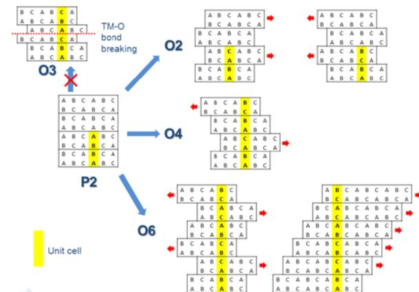
**Figure IV - 130:** This is a schematic model showing the layer gliding process of P2 to O2, O4 or O6 stacking. O stacking occurs when Li enters the alkali metal layer for Na. Li prefers octahedral coordination instead of prismatic coordination so a shear occurs leaving the stacking faults in the material.
