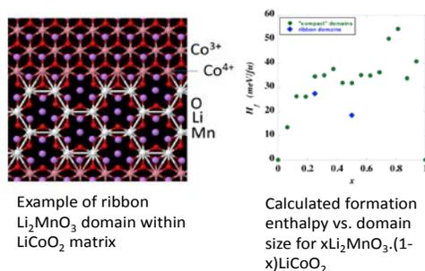
Figure IV - 12: Example  $\text{Li}_2\text{MnO}_3$  Domain within  $\text{LiCoO}_2$  Matrix.
