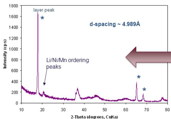
**Figure IV - 128:** XRD pattern of IE product, made by refluxing  $\text{Na}_{1.0}\text{Li}_{0.2}\text{Ni}_{0.25}\text{Mn}_{0.75}\text{O}_y$  in hexanol with 2 fold LiCl for 4 hours, followed by washing with methanol, and vacuum drying.
