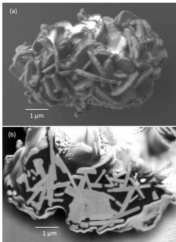
**Figure IV - 26:** Scanning electron micrographs of the  $\text{Li}_{1-x}(\text{Mn},\text{TM})\text{O}_2$  particle from the previous figure (a) in the pristine condition before cycling and (b) after 26 complete charge/discharge cycles.
