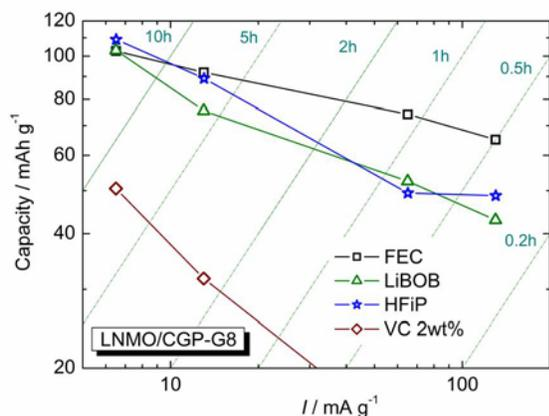
Figure IV - 41: The effect of electrolyte additives on full-cell rate performance.
