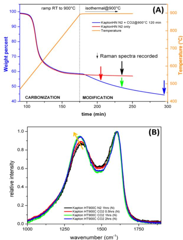
**Figure IV - 199:** TGA analysis (a) and Raman spectra (b) of pyrolyzed polyimide sample with and without heat treatments. (Arrows in the TGA curve mark with corresponding colors the points where Raman spectra were obtained).
