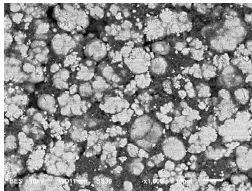
**Figure IV - 240:** Fractured cathode particles from calendaring from lot#2012-02-22.
