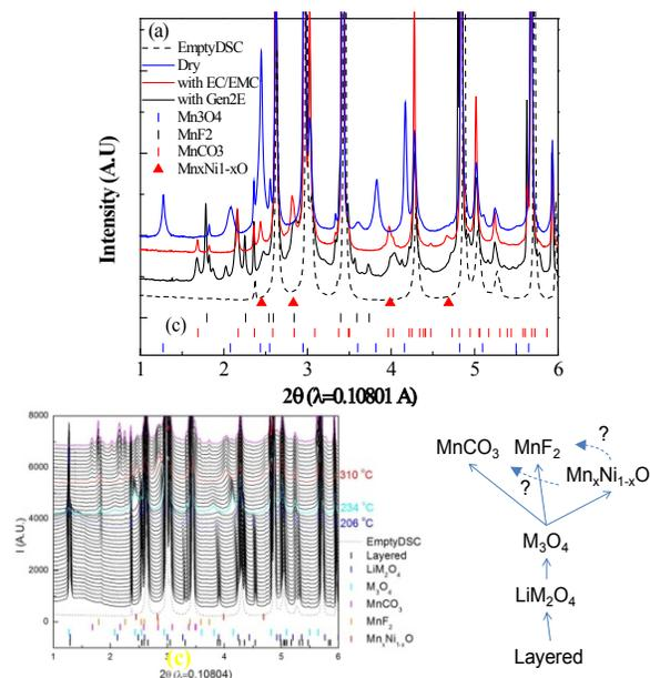
**Figure IV - 220:** (a) Comparison of HEXDRD patterns of abused delithiated HE5050 (charged to 4.6 V vs.  $Li^+/Li$ ) showing that the decomposition pathway strongly depended on the chemical environmental it was exposed to, (b) *in situ* HEXRD pattern of deliithiated HE5050 with the presence of electrolyte, and (c) proposed decomposition pathway for delithiated HE5050 with the presence of electrolyte.
