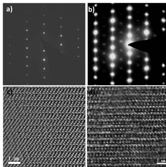
**Figure IV - 22:** Electron diffraction patterns from (a) fresh and (b) 1500 times cycled  $\text{Li}_{1.2}\text{Ni}_{0.15}\text{Mn}_{0.55}\text{CO}_{0.1}\text{O}_2$  showing the transformation from layered to spinel-like structure. Corresponding high resolution images are presented in (c) and (d).
