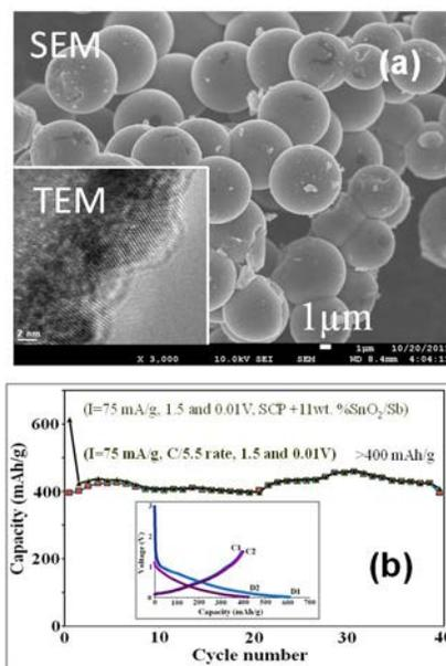
**Figure IV - 103:** (a) SEM and TEM (inset) images of SnO<sub>2</sub>/Sb-coated carbon spheres, (b) First and second discharge-charge-profiles (inset) and capacity vs. cycle number plot of a lithium half-cell with a SnO<sub>2</sub>/Sb-carbon sphere electrode cycled between 1.5 and 0.01 V at a C/5.5 rate.
