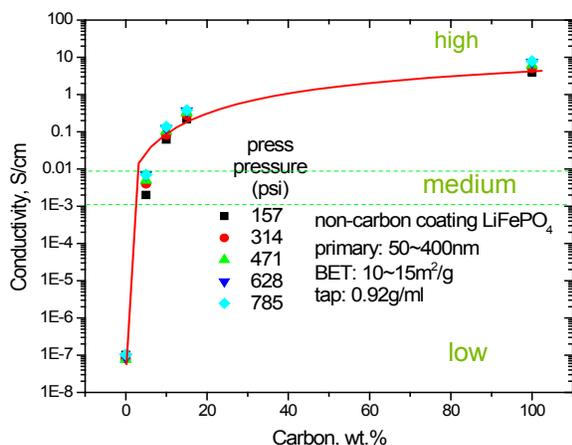
Figure IV - 53: Carbon Additive Effect on Conductivity of LiFePO<sub>4</sub>/Carbon Blend.
