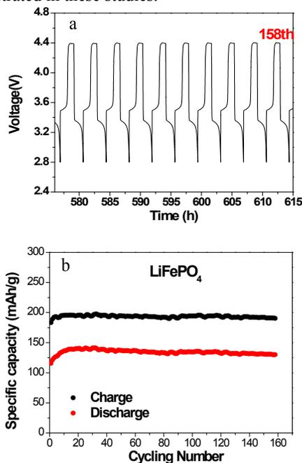
Figure IV - 233: (a) Voltage profile and b) cycling capacities of the polymer-protected cell with a  $\text{LiFePO}_4$  cathode.
