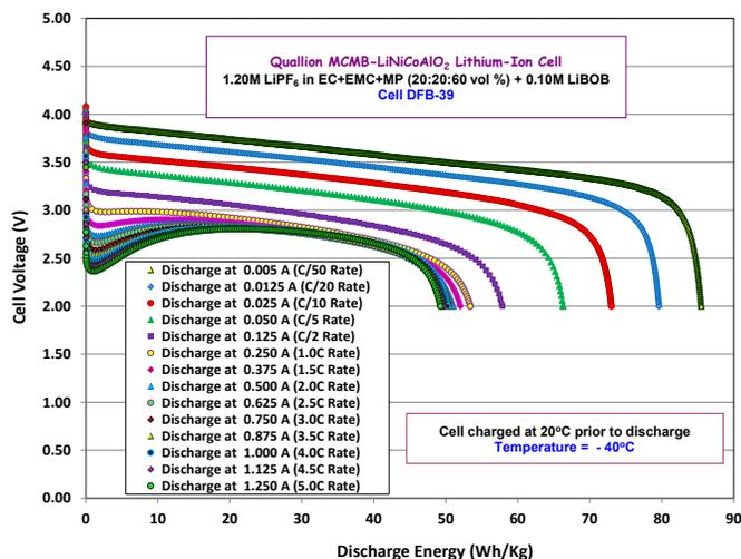
Figure IV - 169: Discharge performance of a 0.25Ah MCMB-LiNiCoAlO<sub>2</sub> cell containing a methyl propionate-based electrolyte with LiBOB at -40°C
