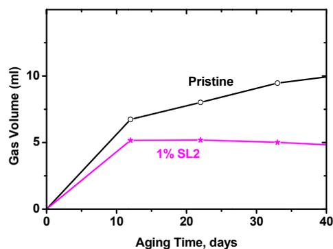
Figure IV - 108: Gas evolution in pouch cells LTO/LMO with /without 1% SL2 as the additive in the electrolyte of 1.2M  $\text{LiPF}_6$  in EC/EMC in 3:7 in weight.
