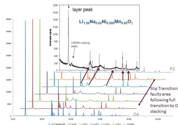
**Figure IV - 129:** P2 to O4 transition showing the DIFFAX results which models the XRD patterns. Note the middle area is the transition whereby stacking faults are present, and the likelihood of mixed O2, O4 and O6 is possible.
