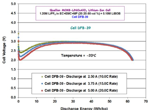
Figure IV - 170: Discharge performance of a 0.25Ah MCMB-LiNiCoAlO<sub>2</sub> cell containing a methyl propionate-based electrolyte with LiBOB at -20°C.
