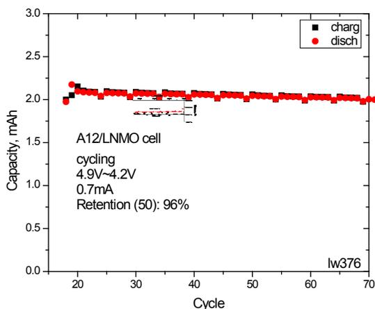
Figure IV - 261: Cycle performance of graphite/LNMO cell.
