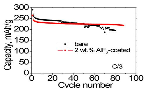
**Figure IV - 112:** Cycling performance of  $\text{AlF}_3$  coated and uncoated (bare) high energy cathode at 55°C.
