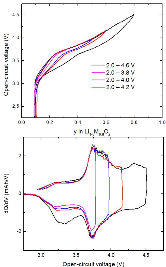
**Figure IV - 184:** OCV curves from GITT measurements to examine hysteresis in LMR-NMC cathode materials. An approximately 1 V hysteresis in site energy is observed between lithium removed at 4.3 V and that re-entered at 3.3 V.
