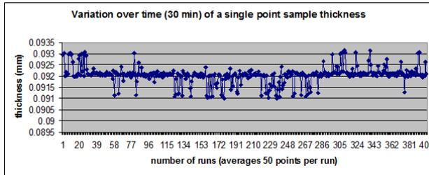
Figure IV - 83: Baseline noise determination from using calibration shim.
