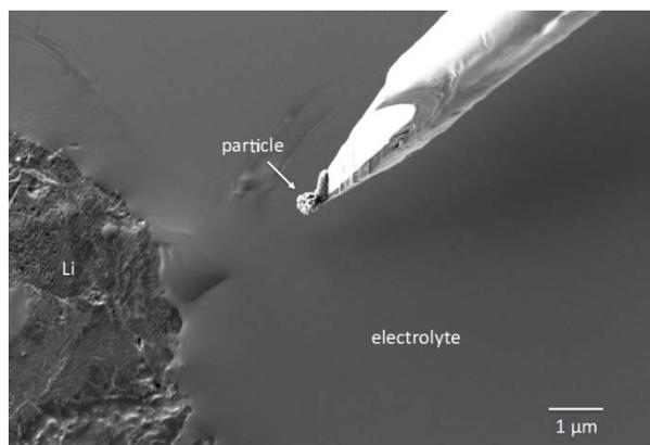
**Figure IV - 24:** Scanning electron microscope image of our microscale battery set up. A single  $\text{Li}_{1+x}(\text{Mn},\text{TM})\text{O}_2$  particle is attached to a probe tip which serves as one electrode and is used to place the particle in the electrolyte covering the anode (Li metal in this case). In this image, the particle is just above the electrolyte.
