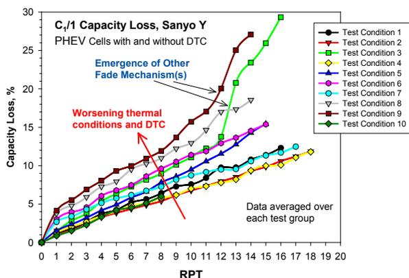
Figure IV - 203: C/1 Capacity Loss, Sanyo Y.
