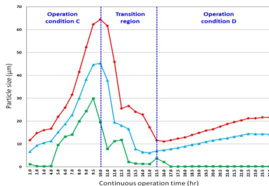
**Figure IV - 239:** Particle size distribution with growth control technology.
