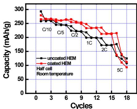
Figure IV - 114: Rate capability of cells based on coated and uncoated high energy cathode material.
