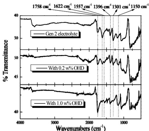
**Figure IV - 144:** FTIR spectra of MCMB electrodes obtained from MCMB/NCM coin cells containing different amounts of OHD in electrolyte of 1.2M LiPF<sub>6</sub> with EC/DEC (3:7 weight ratio) after formation cycles.
