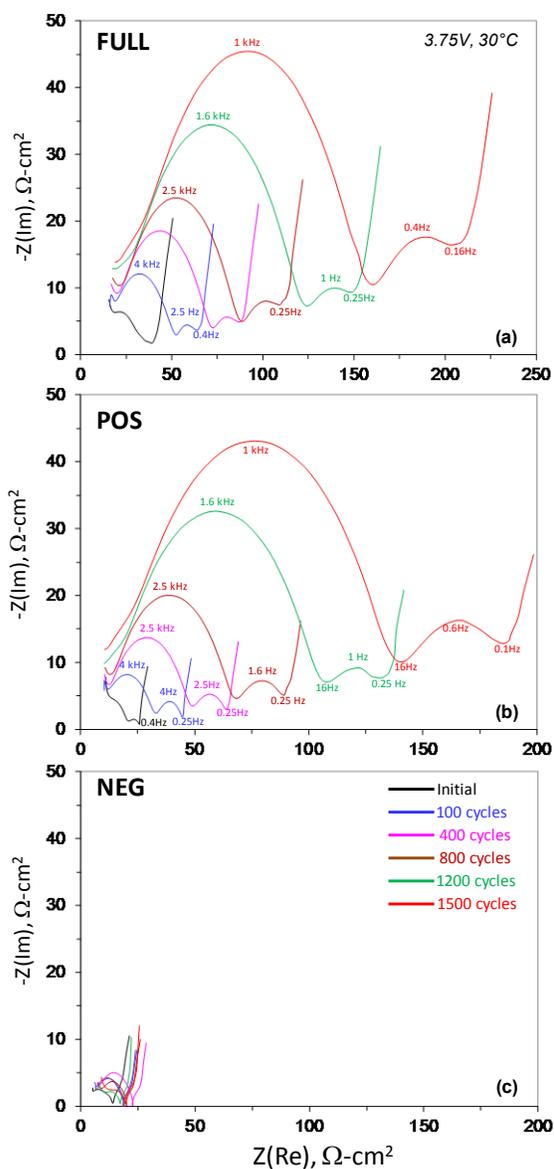
**Figure IV - 191:** AC impedance data from (a) the full cell, and from the (b), (c) positive and negative electrodes showing changes that result from cell cycling. The data were obtained at  $30\text{ }^{\circ}\text{C}$ , at a full cell voltage of  $3.75\text{V}$ , in the  $100\text{kHz}$  to  $0.01\text{ Hz}$  frequency range.
