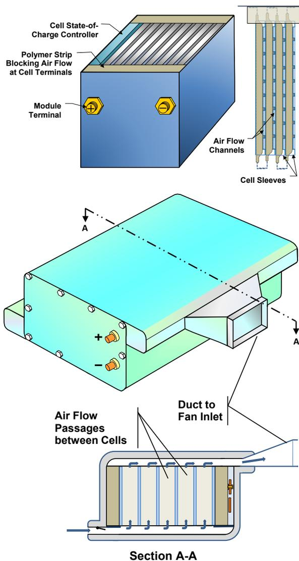
**Figure IV - 187:** New module (top) and pack (bottom) design for batteries utilizing air thermal management in BatPaC.
