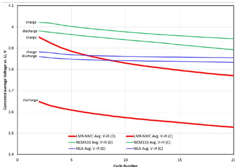
**Figure IV - 6:** Resistance corrected average charge and discharge voltages for the LMR-NMC, NCA and the NCM333 oxides. All three materials show voltage fade, however fade is strongest for the baseline material.
