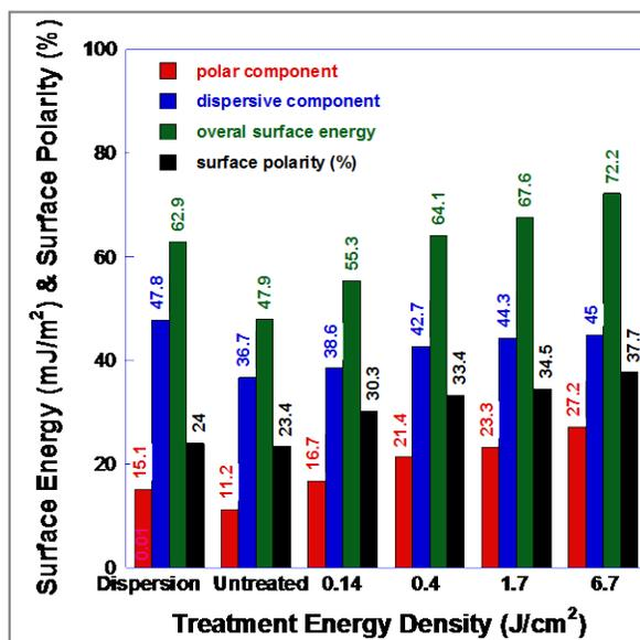
Figure IV - 74: Surface energy of treated and untreated Al foils and LiFePO<sub>4</sub> aqueous dispersion; the surface energy and polarity of Al foils increased with increasing corona treatment energy density.
