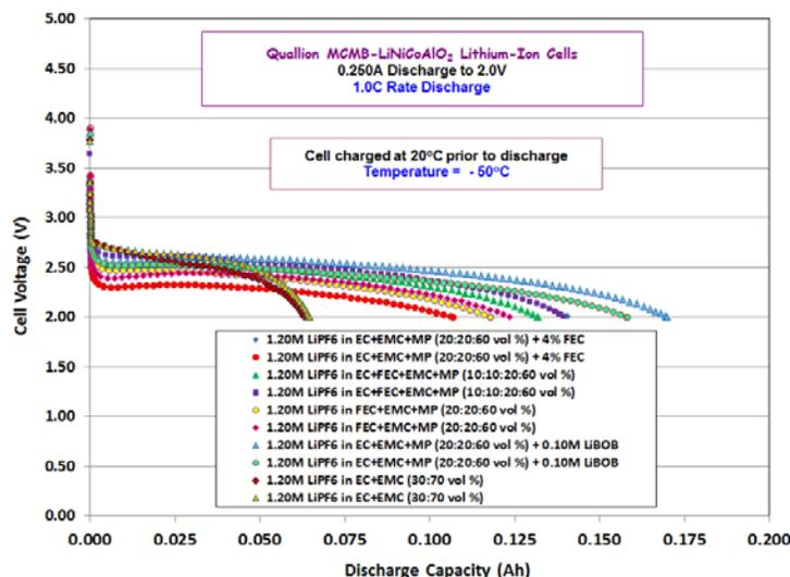
**Figure IV - 168:** Discharge performance of 0.25Ah MCMB-LiNiCoAlO<sub>2</sub> cells (Quallion, LCC) containing various electrolytes  $-50^{\circ}\text{C}$  using a C-rate discharge.
