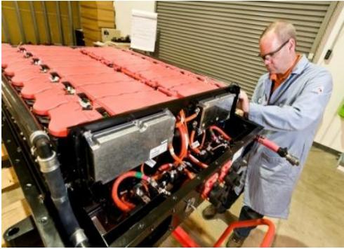
**Figure II - 9:** Complete battery packs and systems are assembled domestically prior to being sent to the customer.
