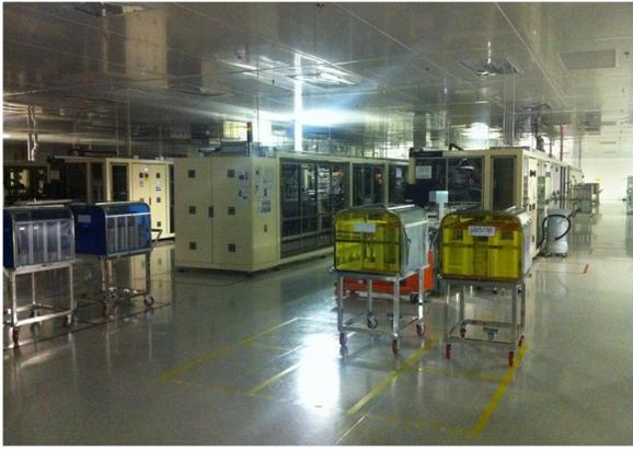
**Figure II - 31:** The folding equipment for the assembly process.
