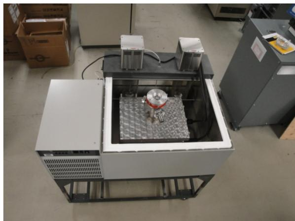
**Figure II - 118:** NREL Designed and Fabricated Cell Calorimeter in Fluke Isothermal Bath.
