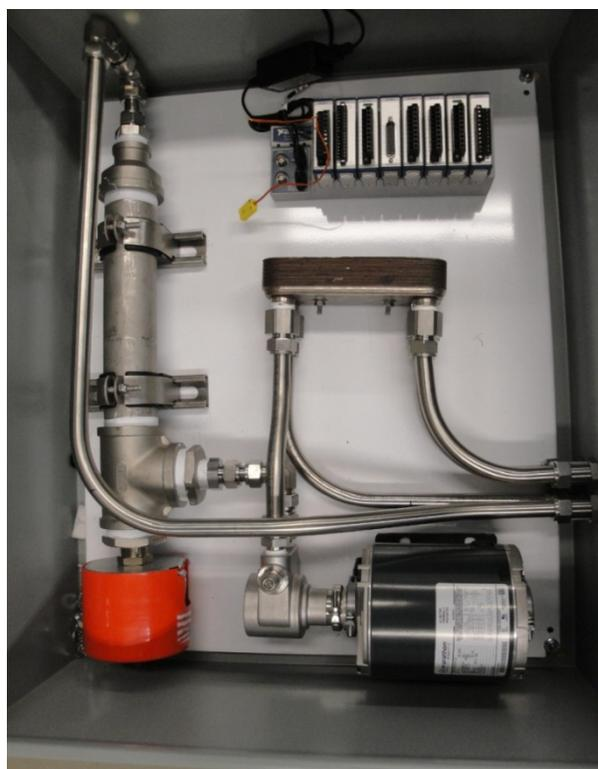
**Figure II - 119:** Liquid Handling Thermal Management In-the-Loop.
