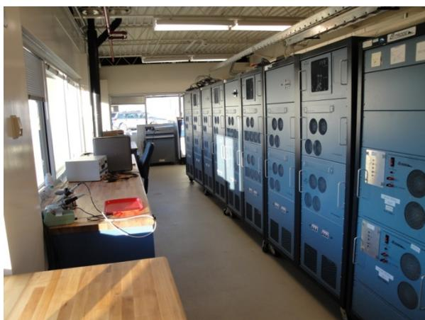
**Figure II - 117:** High and Medium Power Battery Cyclers.
