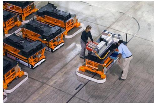
**Figure II - 49:** Battery Pack Assembly on Automated Guided Carts.
