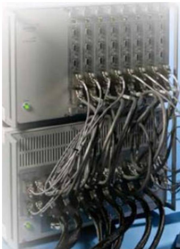
Figure II - 97: Solartron (Ametek) eight channel electrochemical test station and impedance analyzer.
