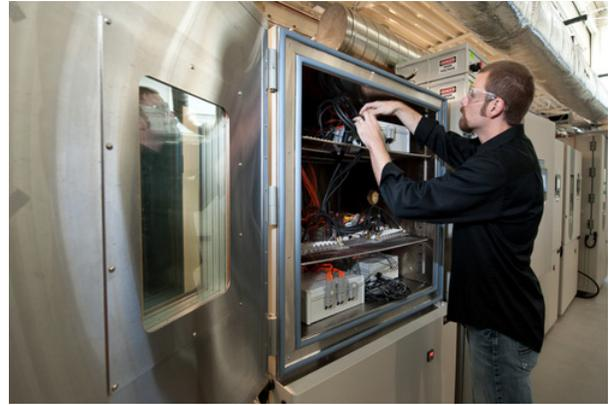
**Figure II - 123:** Life cycle testing of batteries for secondary use applications.
