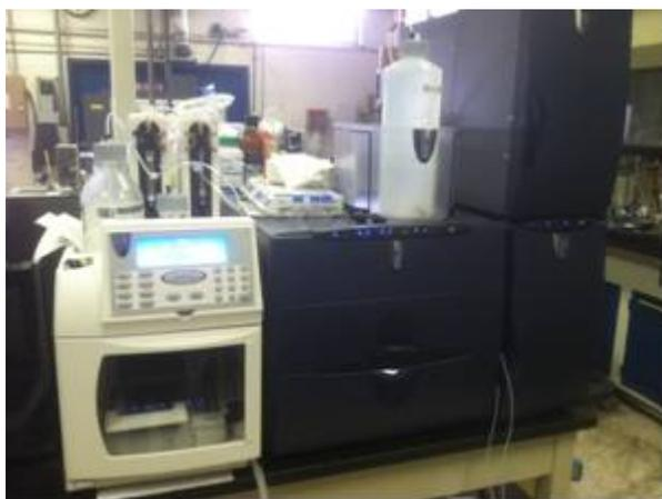
**Figure II - 75:** Ion Chromatograph (Novolyte).
