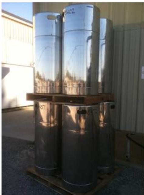
**Figure II - 74:** Several examples of the 400 215-L Electrolytes shipping vessels purchased in 2010 (Novolyte).
