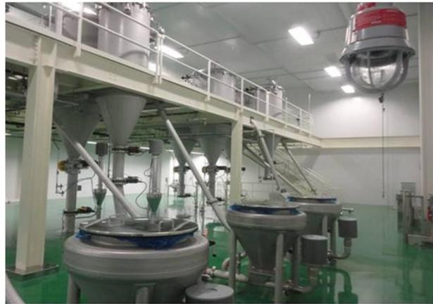
Figure II - 29: The bag filters on the 4<sup>th</sup> floor of the mixing tower of the electrode process.
