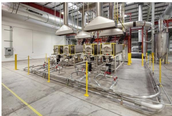
Figure II - 73: EnerG2 Pyrolysis Kilns.
