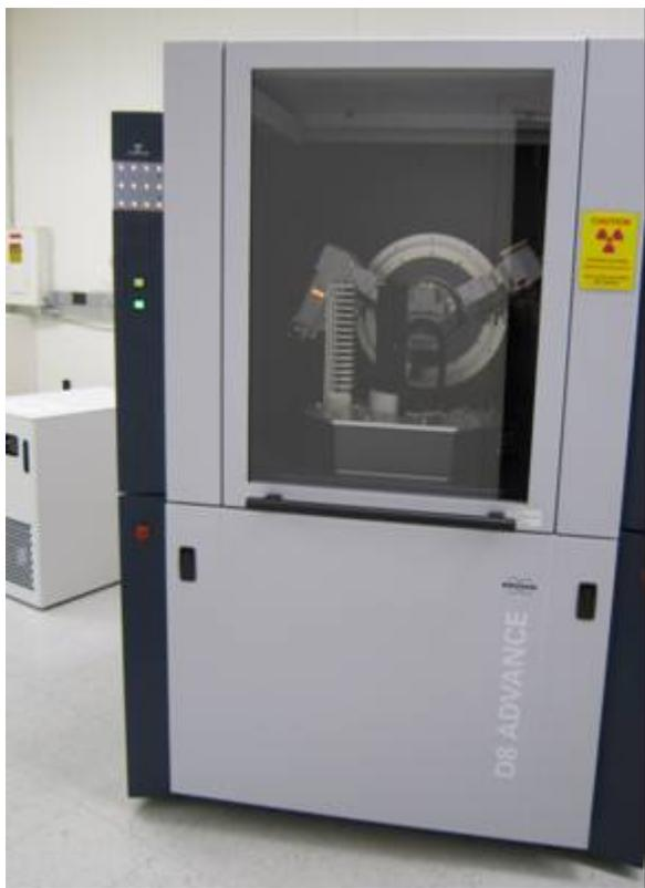
Figure II - 95: Bruker D8 advanced powder diffraction system.
