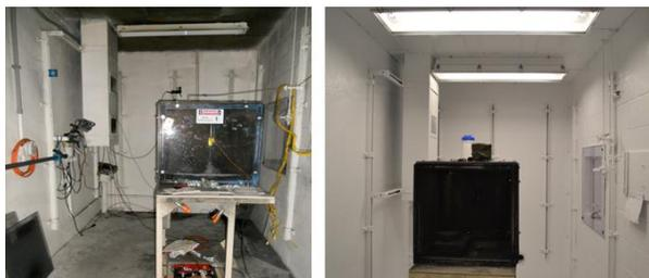
**Figure II - 124:** (right) before and (left) after photographs of a typical test cell in the Battery Abuse Laboratory.
