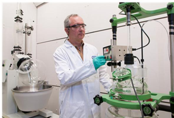
Figure II - 103: 20L Reactor and Rotavap (ANL).
