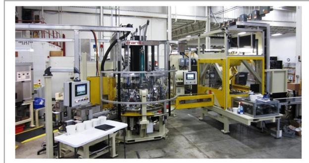
Figure II - 87: Equipment – Battery Cover Assembly Equipment (HTTM LLC, H&T, Trans-Matic).
