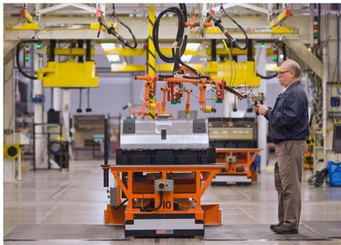
**Figure II - 48:** Battery Pack Lift Assist.
