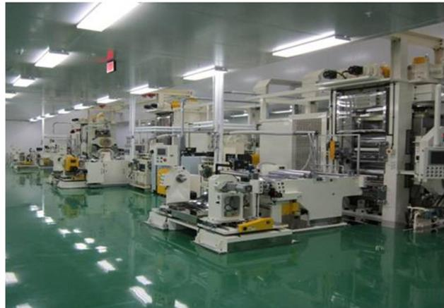
Figure II - 30: The roll press equipment for the electrode process.
