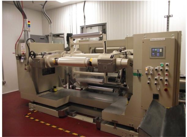
Figure II - 42: Unwinder Anode Coater – Hague Rd.
