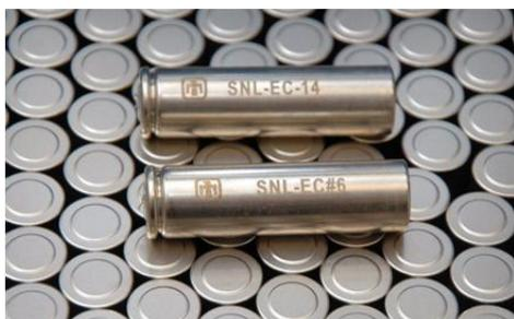
Figure IV - 183: Photograph of 18650 cells built at SNL
