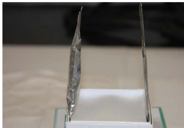
Figure IV - 30: LTO/LMO pouch cells before (right) and after (left) 80 days of aging at 63°C. The electrolyte is 1.2 M LiPF<sub>6</sub> in ethylene carbonate (EC)/ethyl methyl carbonate (EMC) at ratio of 3:7.
