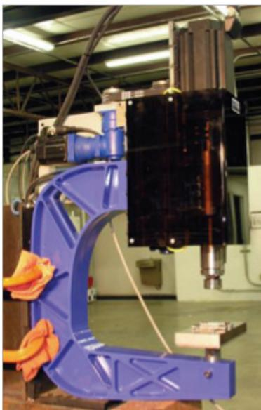
Figure 2. Prototype FBJ machine with a Cframe.
