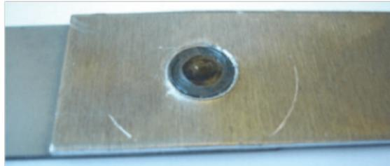
Figure 3. Appearance of FBJ between DP 980 AHSS and AA 5754 aluminum.
