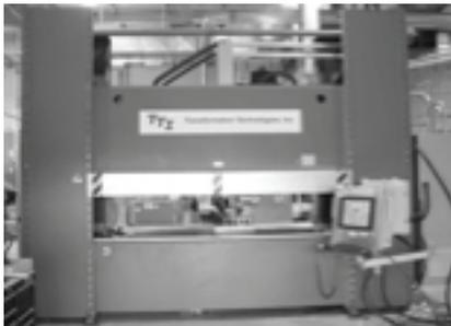
Figure 1. Precision FSW machine located at PNNL
