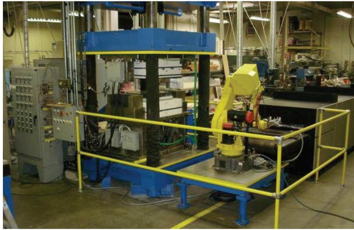
Figure 14. Photograph of the forming cell with robot and end effector.
