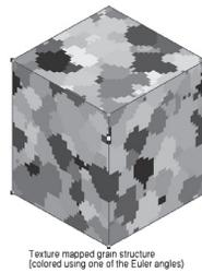
Figure 43. Three-dimensional grain structure to which the EBSD texture is mapped.
