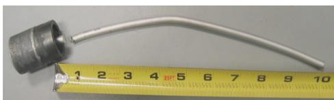
Figure 14. Magnesium alloy AZ61 extrudate obtained during preliminary extrusion experiments.
