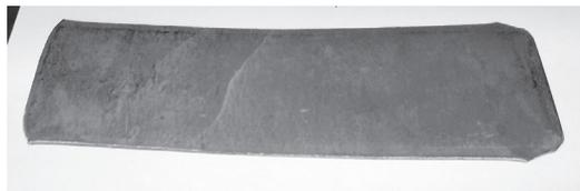
Figure 38. MEL Mg alloy #129 as hot rolled at 400°C clad to a thickness of 1.5 mm.
