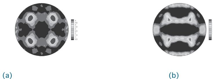
Figure 44.  $\langle 111 \rangle$  pole figures showing the texture in (a) 1/8" hot band and (b) computed texture in 1/32" sheet after plane-strain compression.
