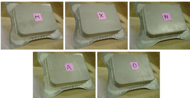
As shown above, forming windows were developed for the five different materials evaluated in this project. All five materials exhibited a robust forming window above 300C. The materials could be stamped in to a 70 mm deep pan without wrinkling or splitting. An example of a successful pan for each material is shown in Figure 8 below, for pans formed at 350C.
