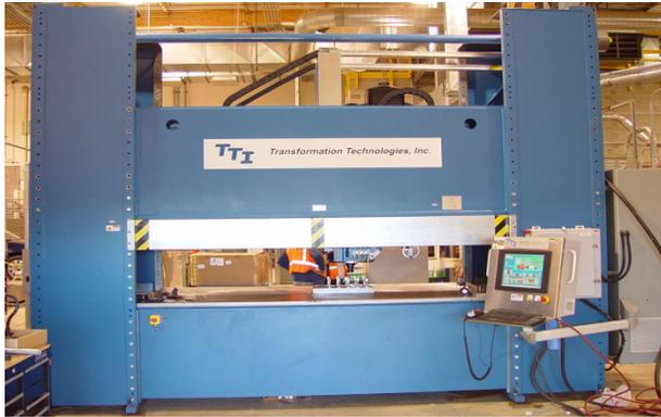
**Figure 1.** Precision FSW machine located at PNNL.
