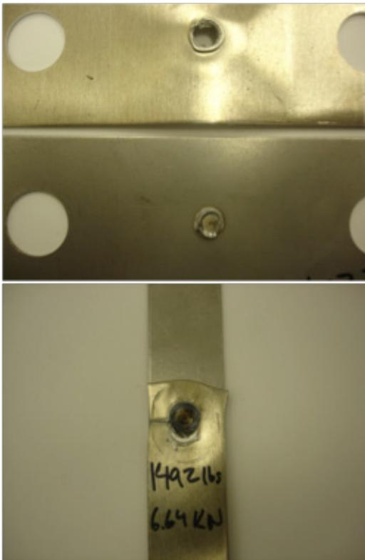
**Figure 6.** Weld button pullout failure mode observed in FBJ of AA 5754 to DP 980.
