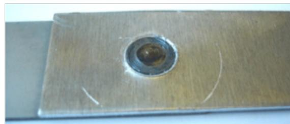
**Figure 3.** Appearance of FBJ between DP 980 and AA 5754.
