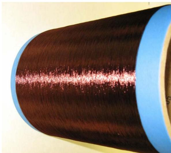
**Figure 4.** Lignin fiber tow comprising 12 filaments, each 11  $\mu\text{m}$  in diameter.
