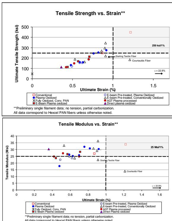
**Figure 1.** Mechanical properties of CFs stabilized and oxidized by various routes then conventionally carbonized at low temperature. There was no tensioning, controlled stretching, or tow spreading during conversion. Conventional data points are for thermally shocked and thermally ramped heating protocols.
