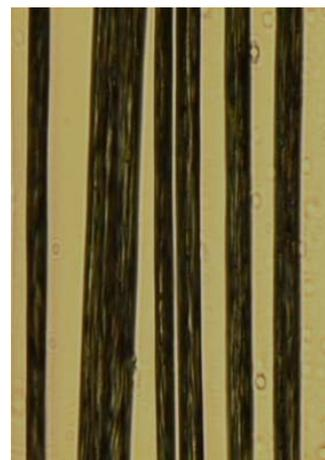
**Figure 7.** Carbon fibers produced from FISIFE precursor.
