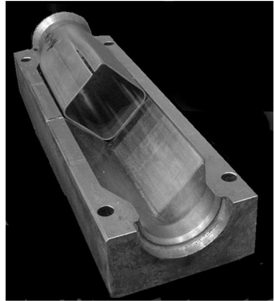
**Figure 2.** Hydroformed Tube and Die (the test was run to failure of the tube).
