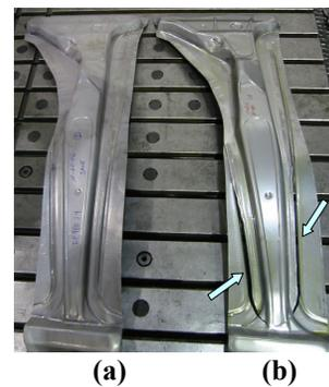
**Figure 12.** Fractured B-pillar, made of DP 980, during stamping process: (a) Type A and (b) Type B.
