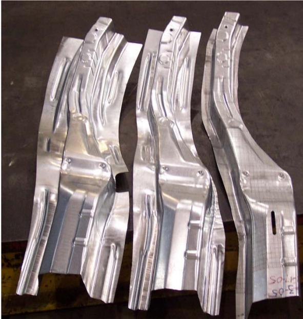
**Figure 2.** Rail stampings from three processes (from left to right: draw process– part on post; draw process–part on binder; form process).
