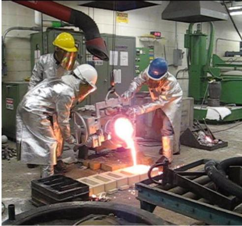
**Figure 5.** Photograph of casting steel in the Missouri University S&T foundry.
