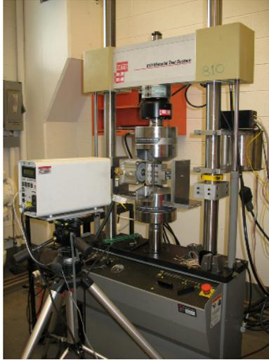
**Figure 1.** T/C and C/T test device developed by OSU.
