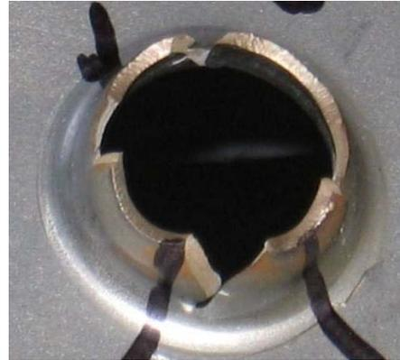
Figure 9. Example of performance of DP980 in flanging a 5 mm diameter hole.
