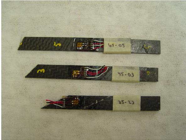
**Figure 6.** Typical failed off-axis tension specimens.
