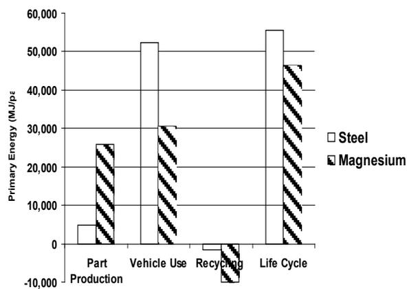
**Figure 2.** Life-cycle primary energy estimates of an automotive front end.
