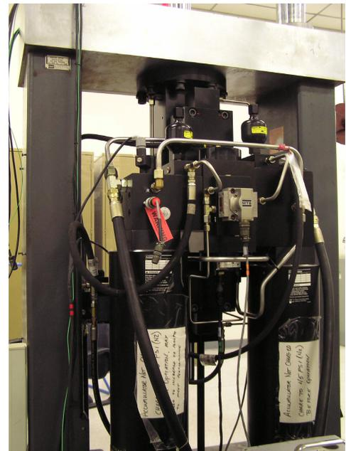
**Figure 8.** Accumulators and servovalve for high strain rate test machine.
