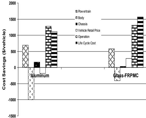
**Figure 1.** Estimated cost savings of two 25% body and chassis weight reduction vehicle scenarios.
