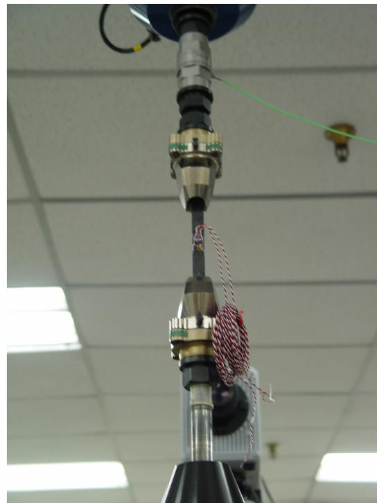
**Figure 5.** Typical coupon test setup on high strain rate tension machine.
