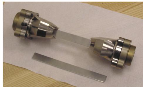
**Figure 9.** Low-mass grip used in high strain rate test machine.
