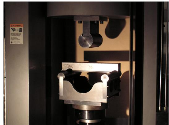
**Figure 2.** Three-point-bend test setup on TMAC.
