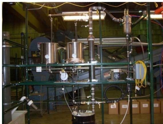
**Figure 2.** Extruder with die and vacuum knockout pot used in the devolatilization testing.
