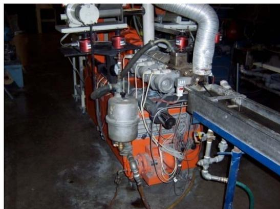
**Figure 1.** Experimental apparatus for testing the ANL two-stage process.
