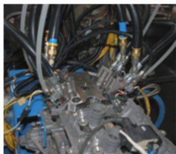
Research engine with fully flexible valve system, boosting, and EGR system.
