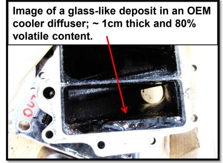
HC deposition is strongly a function of the wall temperature and volatility of the HCs; expanded use of higher-boiling HCs (such as biodiesel) in fuel is expected to increase the risk of plugging.
