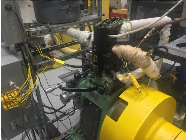
Figure 3. CFR engine with surrounding subsystems to create the PRF mapping using HCCI to determine the autoignition tendency of the reformat mixtures
