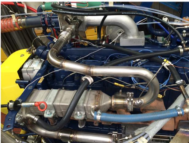
Figure 5. Initial turbocharger size and EGR system engine configuration
