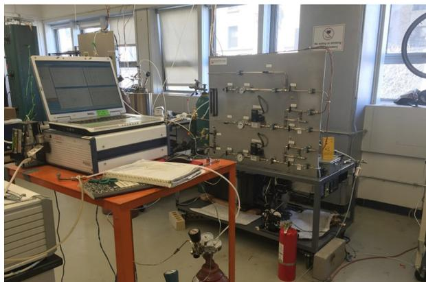
Figure 1. Test facility to reformat diesel, gasoline, and natural gas to varying level and determine their speciation using gas chromatography
