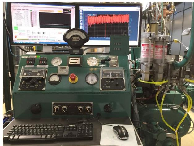
Figure 1. Instrumented and commissioned CFR F1/F2 fuels rating test engine installed at Argonne National Laboratory
