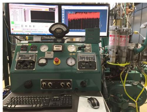
Figure 1. Instrumented and commissioned CFR F1/F2 fuels rating test engine installed at Argonne National Laboratory (Kolodziej, report II.2)
