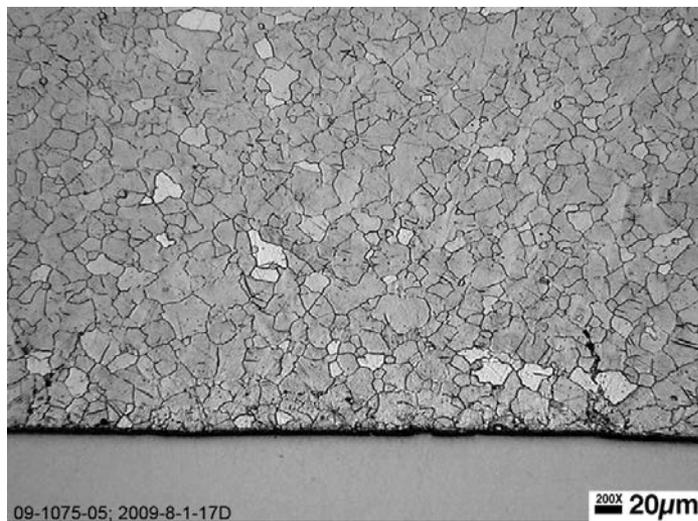
After one second the microstructure of the AZ31 has recrystallized
