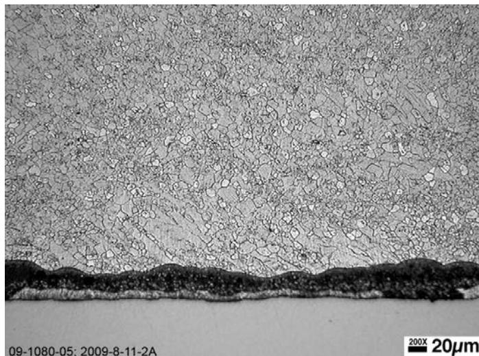
At 0.4 seconds the microstructure remains unchanged
