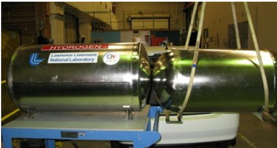
Figure 1. Generation 2 cryo-compressed hydrogen storage tank prototype (left). Generation 3 cryo-compressed hydrogen storage tank prototype (right).
