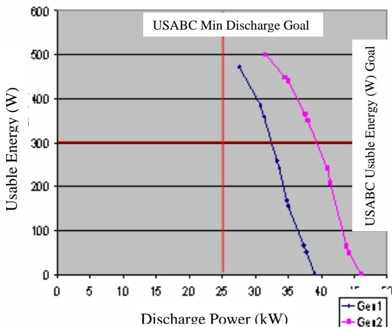
Figure 1: Usable Energy vs. Power for the Gen 1 and Gen 2 Cells.
