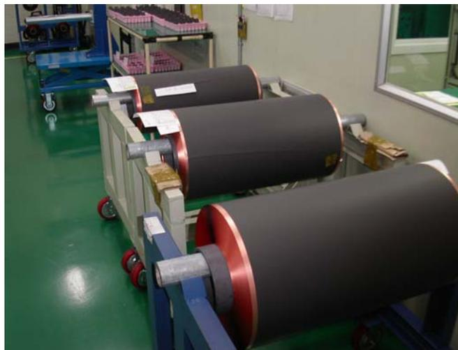
Figure1-2: Automotive cell fabrication dryer & coated rolls in A123's plant.
