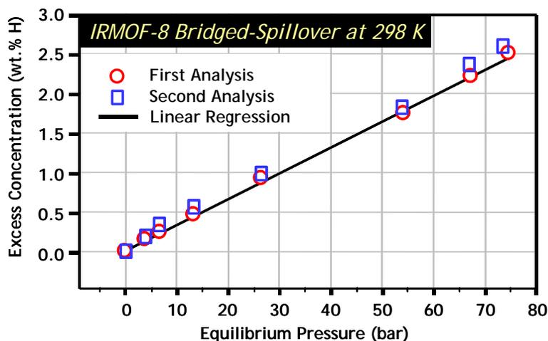
Figure 1: High-pressure hydrogen uptake (wt%) at 298 K for IRMOF-8 bridged-spillover. The first analysis (red circles), synthesized and tested at UM, was then corroborated via a second analysis (blue squares) synthesized and tested by the INER and SwRI respectively.
