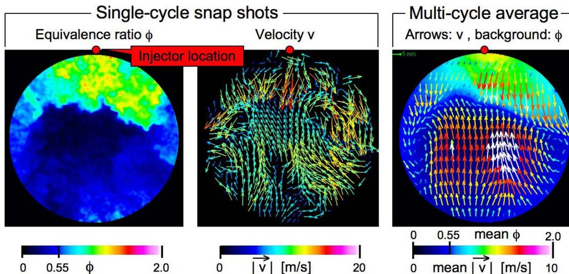
Fuel distribution and charge motion in a plane parallel to the piston top at  $32^\circ$  before top dead center after  $H_2$  injection from  $90^\circ$  to  $40^\circ$ . Left: Fuel is located near the injector just after the end of injection. Center: Instantaneous gas-flow field showing turbulent flow structures. Right: Cycle-average flow field. Flow diagrams show that highly turbulent fuel from the top encounters unmixed air from the bottom.
