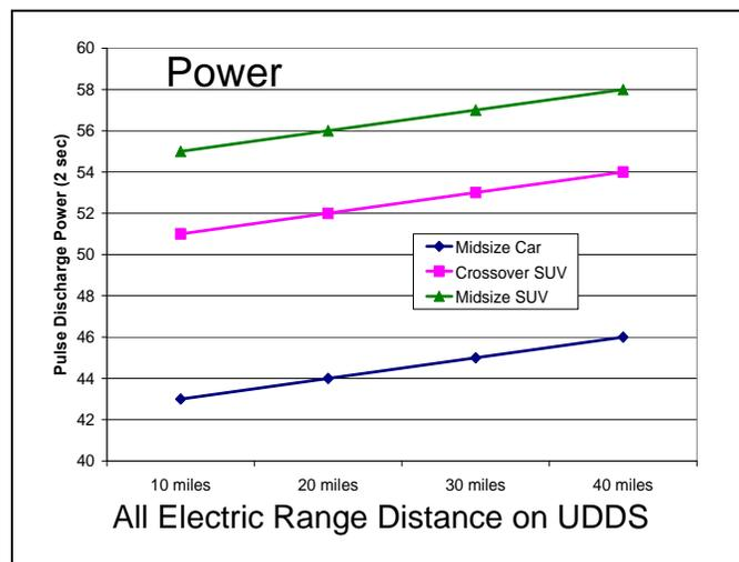
Figure 2: Battery power required during a 2 second acceleration, of max power demand, within the cycle
