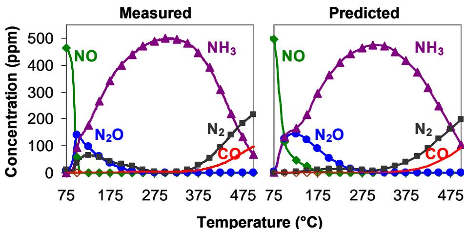
Illustration of the good correlation between experimental measurements and kinetic model predictions of the products formed in an LNT catalyst during reduction of nitric oxide (NO) by hydrogen over a wide range of temperatures.
