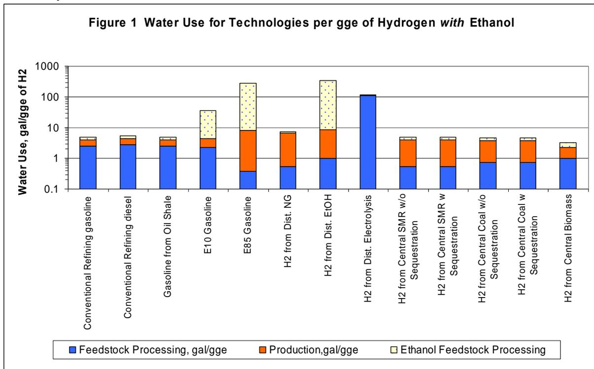
Figure 1: Water consumption for various hydrogen production pathways.
