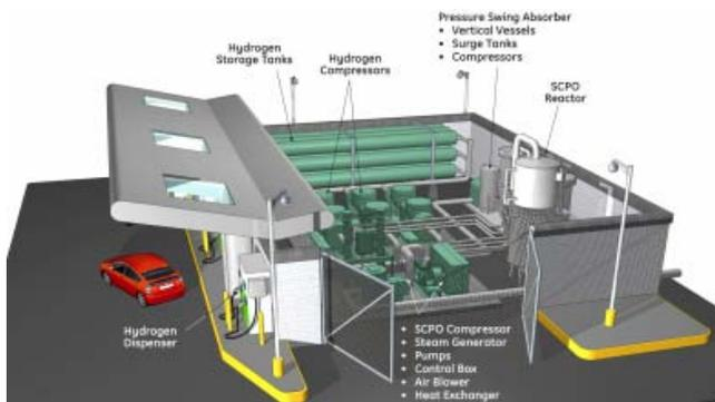
Figure 1: GE Global Research rendering of a production unit integrated into 1,500 kg/day hydrogen refueling station
