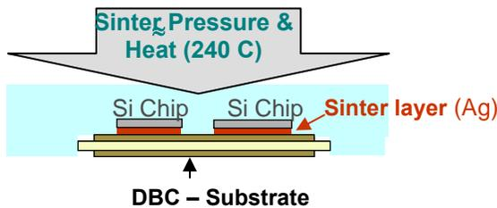
Figure 1: DBC, sintering layer and silicon chips
