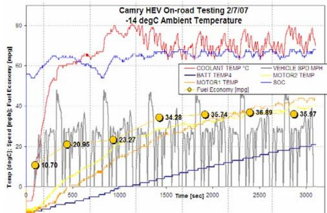
Figure 2: Fuel economy is raised to the optimum of 35 mpg after 40 minutes (2400 seconds) of driving, at ambient temp of -14 deg C.
