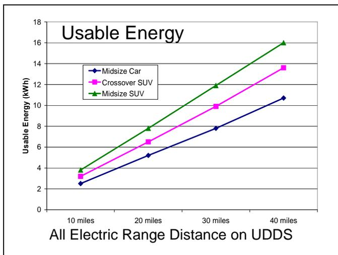
Figure 1: Battery energy required, as a function of, vehicle mass and driving distance, within the cycle
