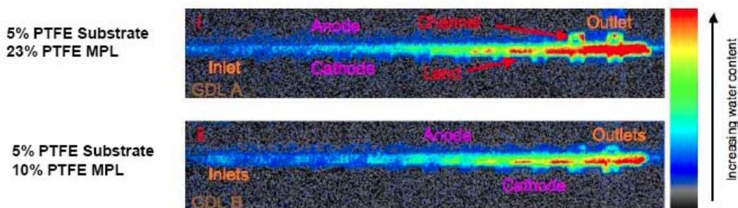
Figure 1: Water accumulation detected by neutron imaging in two cells with different microporous layer PTFE loading.
