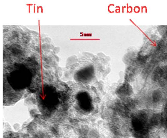
Figure 1: 1 to 8 nm sized tin particles into a matrix of carbon
