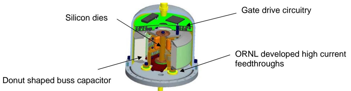
Figure 1: ORNL Floating Loop Inverter
