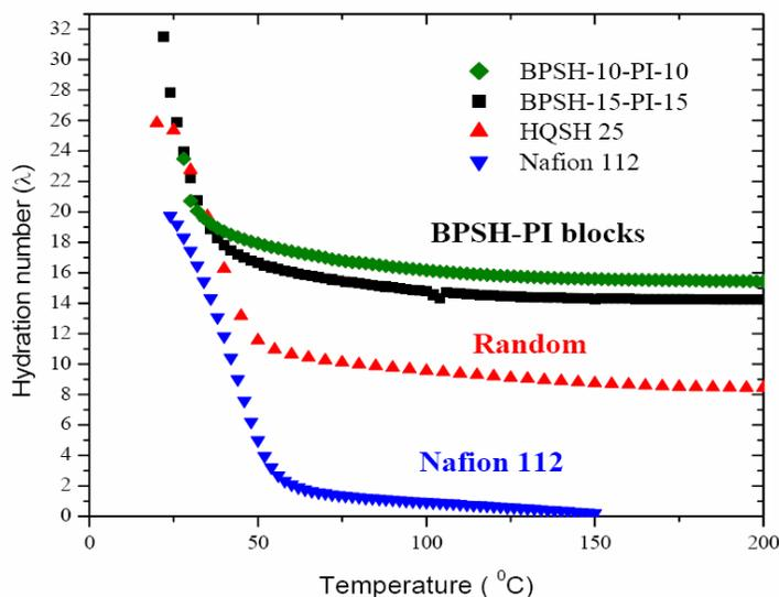
Figure 1: Water content of Virginia Tech and Nafion membranes vs. temperature
