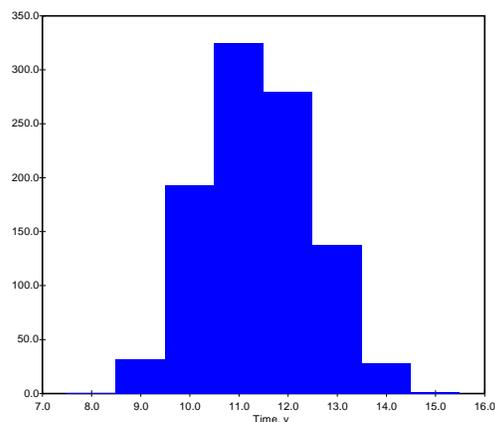
Figure 2: Shows the results of the Monte Carlo Simulation of 1000 trials from which one derives an estimate of the mean life and of the 90% confidence limit.
