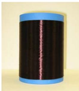
Fiber diameter was purposefully varied from 22 to 11 microns by varying take up speed, as shown in the diagram to the right. These results closely correlated to the theoretical and demonstrated that purified hardwood lignin can be continuously melt-spun into fiber form. This constitutes a significant step towards the overall objective of producing low cost carbon fibers from a renewable resource.
