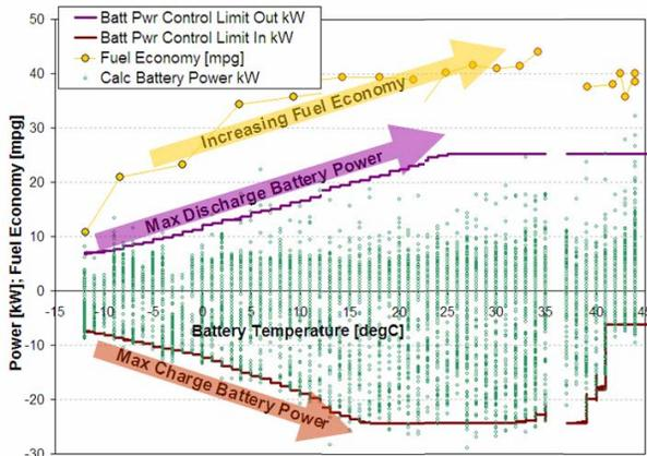
Figure 1: Hybrid battery functionality is not realized until battery reaches 15 to 25 deg. C.
