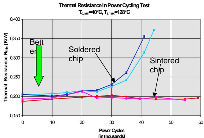
Figure 2: Effects of Power Cycling on Thermal Resistance
