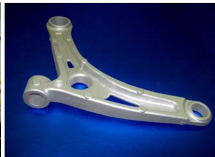
Figure 3: Magnesium Front Lower Control Arm
