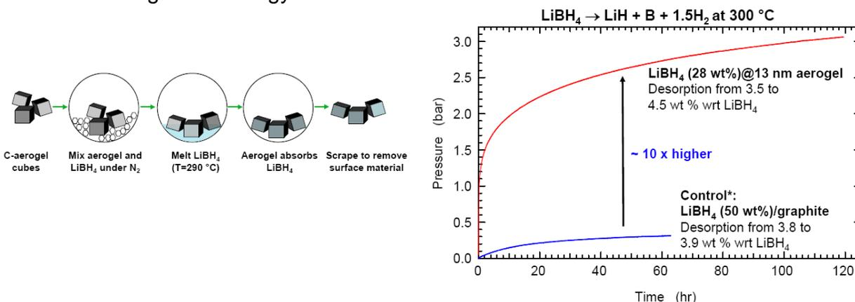
The complex hydride LiBH<sub>4</sub> can be caused to nearly fill an aerogel framework, improving its performance by lowering the temperature of hydrogen release and increasing hydrogen uptake.
