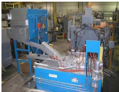
Figure 1: Contech Squeeze Casting Cell
