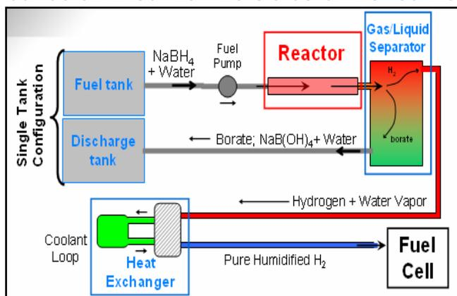
Schematic of SBH On-Board System
