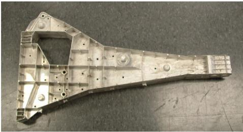
Figure 1: Thixomolded magnesium shotgun casting
