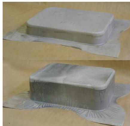
Figure 2: Deep-drawn panels warm-formed using a purpose-built warm-forming die.
