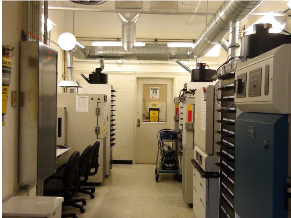
Three MACCOR cyclers with 96 multi-range channels each. Exhaust ventilation to ovens provided in case of thermal events.
