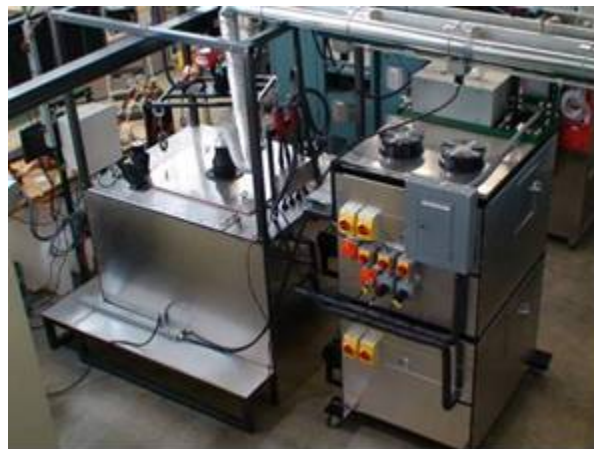
Figure III-78: NREL's battery pack calorimeter
