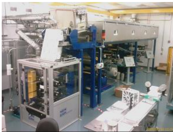
Figure III-30: New prototype production gravure Gel coater, incorporating both UV polymerization and convection drying.
