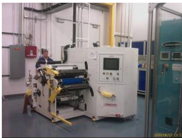
Figure III-31: New anode slitting station.
