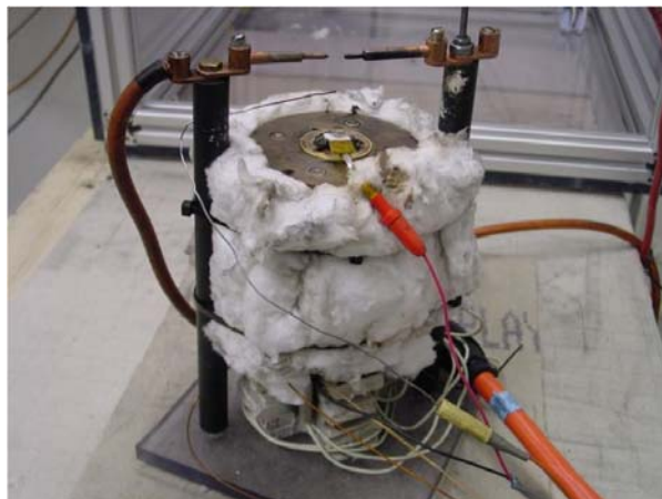
Figure IV- 132: Thermal ramp apparatus for testing thermal runaway and flammability of vent gases.
