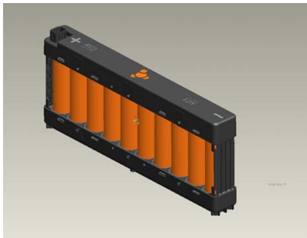
Figure III-17: A123 10-cell Module Design
