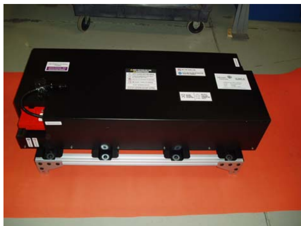
Figure III-60: JCS 344-Volt battery pack
