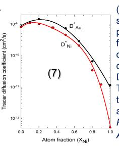
(7) Fit using suitable polynomials for functional form of isotopic diffusivity  $D_k^*(X_1, X_2, ...,$ T) (e.g. Au-Ni tracer diffusion at 900°C. Reynolds et al. Acta Met. '57)
