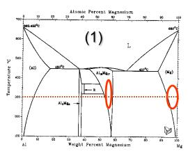
(1) Prepare single phase alloy sample (e.g., Mg-5%AI) at T<sub>o</sub>
