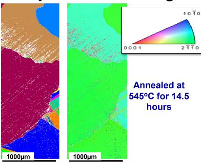
Electron Backscatter Diffraction (EBSD) map (inverse pole figure – top right) of grain orientations in a pure polycrystalline Mg rod after annealing treatment. left: Identical grain structure map with enhanced contrast.
