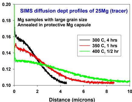
SIMS concentration depth profiles of <sup>25</sup>Mg as a function of depth in Mg polycrystalline samples with very large grain sizes (hundreds of μm)
