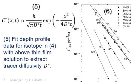
(6) Repeat for different temperatures (%) compositions to check for Arrhenius fits (e.g. Au in Au-Ni alloys, Kurtz et al., Acta Met.'55)
