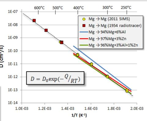
Mg tracer diffusivities as a function of reciprocal temperature for pure Mg and three Mg alloys (Wt %)
