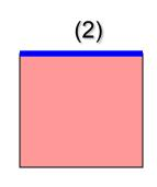
(2) Deposit thin film (100 nm) of stable isotope of an alloy element (e.g., Mg<sup>26</sup>) on annealed sample
