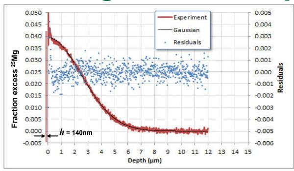
**Example of SIMS measured** excess abundance of tracer (Mg-25) as a function of depth for a magnesium sample diffused for ~1 hour at 350°C. The thin black curve shows the fit to obtain the diffusion coefficient and the blue dots are the residuals or differences between the experimental and fitted points. The fitted initial isotopic film thickness, h, is consistent with independent thickness measurements.
