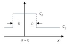
Thin-film error function solution fit (least-square) to obtain 23 Madiffusivity, background abundance and initial tracer film thickness. for the U.S. Department of Energy
