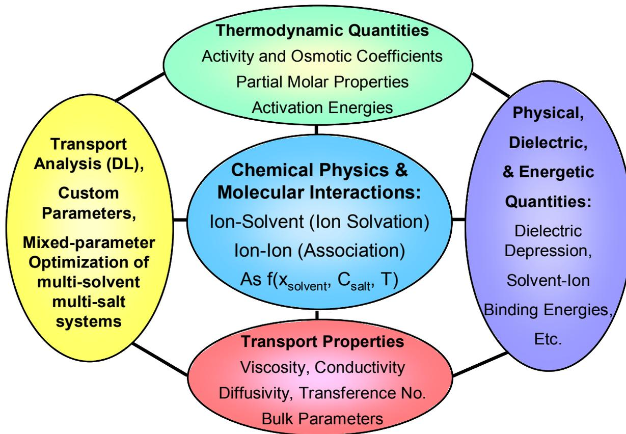
The AEM is routinely used for extensive evaluation of battery electrolyte systems in DOE-EERE and the Private Sector.
