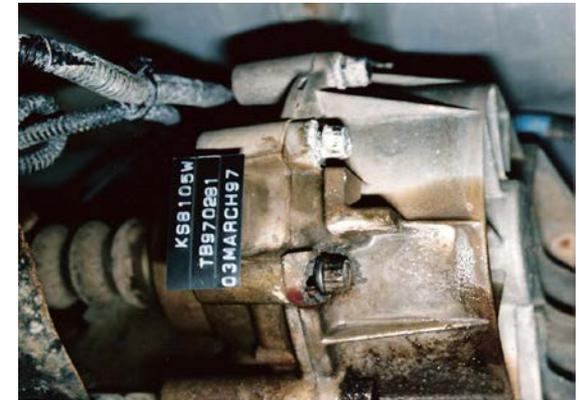
**Transfer case exhibiting perforation and oil leak without effective isolation**
