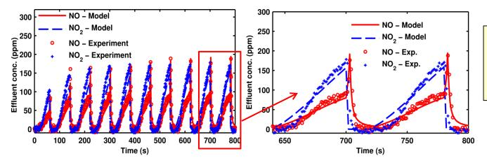
Model captures both initial and cyclic steady-state NO<sub>x</sub> profiles
