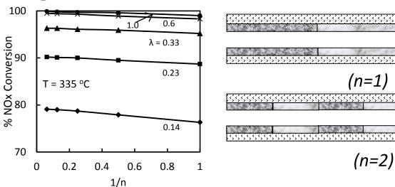
Serial design with LNT & SCR sections of equal length Catalysts: Pt/BaO (LNT) Cu/ZSM-5 (SCR) Length of each catalyst = 2cm;  $GHSV=60,000\ h^{-1}$ ; Lean inlet:  $NO=500ppm,O_2=5\%$ ; Rich inlet:  $NO=500ppm,H_2=0.875\%$ ;  $\lambda$  =  $Total\ LNT\ length/Total\ SCR\ length$  n =  $number\ of\ LNT-SCR\ bricks$
