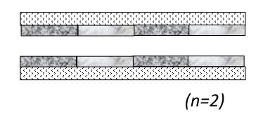
Length of each catalyst = 2cm;  $GHSV=60,000h^{-1}$ ; Lean inlet:  $NO=500ppm,O_2=5\%$ ; Rich inlet:  $NO=500ppm,H_2=0.875\%$ ;  $\lambda$  = Total LNT length/Total SCR length  $t_L = 6t_R$
