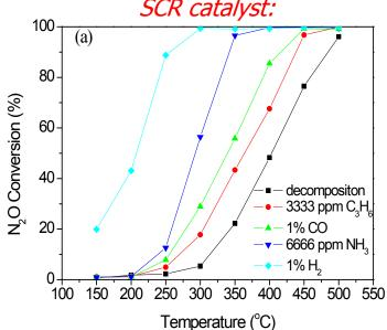
Feed: 100 ppm  $N_2O$ , 5%  $H_2O$ , 5%  $CO_2$ , reductant as shown, bal.  $N_2$ ; GHSV = 30,000  $h^{-1}$
