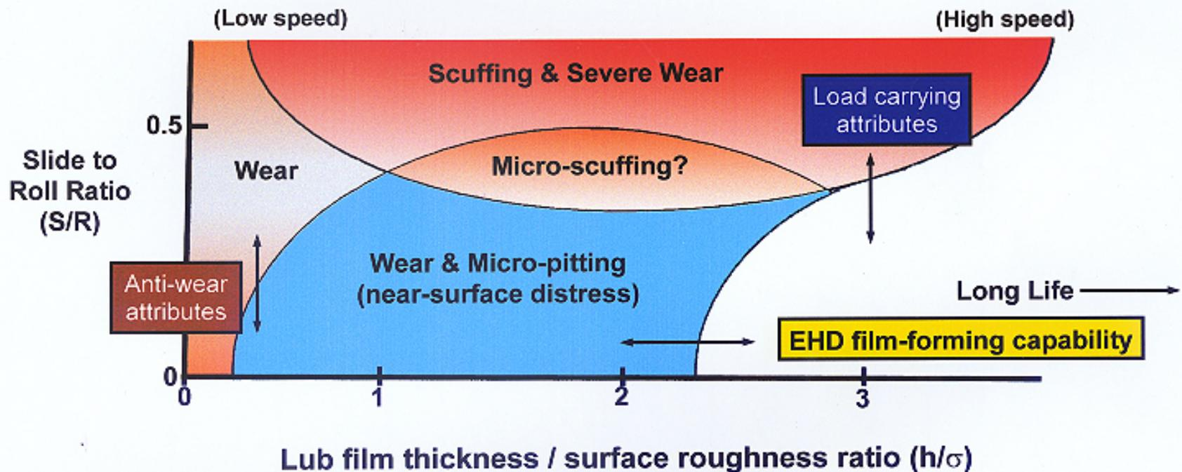
Schematic of life-limiting surface failure modes (boundaries are postulated)
