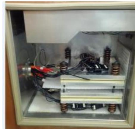
Test Cells in Thermal Chamber
