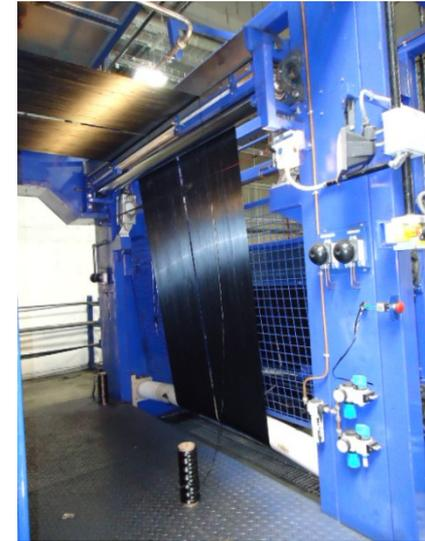
**Oxidized sample fed through commercial line furnace; carbon fiber wound using commercial winder**
