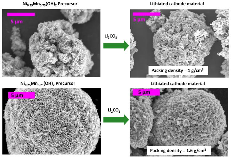
Tuning of both experimental and engineering conditions during CTRS co-precipitation have led to obtaining spherical particles and higher packing density Ni<sub>0.25</sub>Mn<sub>0.75</sub>(OH)<sub>2</sub>
