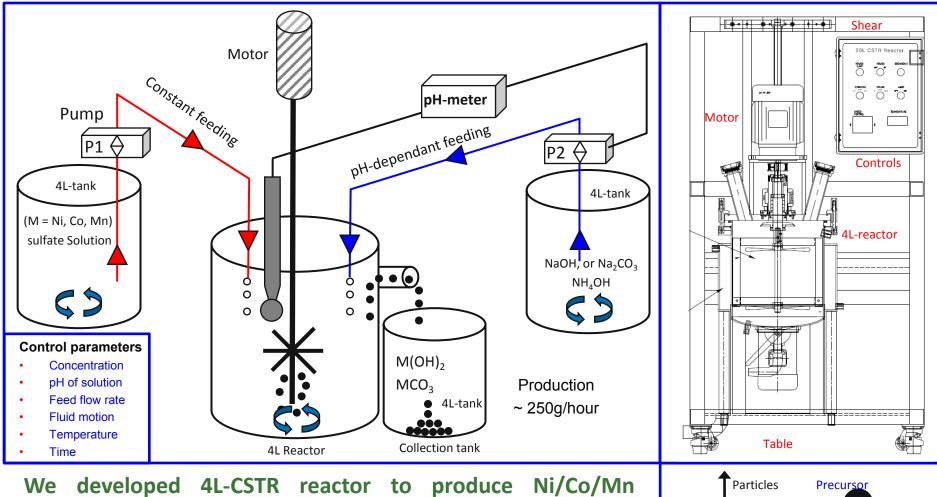
We developed 4L-CSTR reactor to produce Ni/Co/Mn carbonate, hydroxide, oxalate precursors. Basic design was transferred to ES division at Argonne for scale up.
