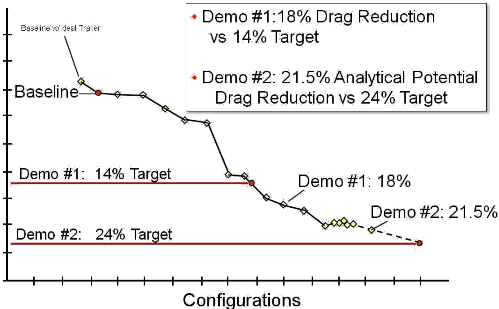
\* Cd's Shown Are Adjusted to SAE J1252 Baseline Using % Average Deltas From 0 and 6 Degree CFD Runs
