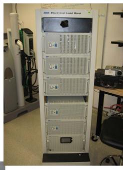
Labview based test rack; AC, DC loads and sources; J1772 signal pass through monitoring/fault injection
