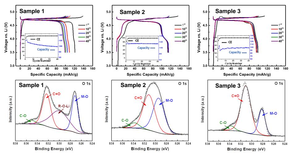
□ Sample 2 exhibits the best cycling performance and does not have surface contamination as shown in XPS. This sample will serve as baseline cathode for novel electrolyte screening.
