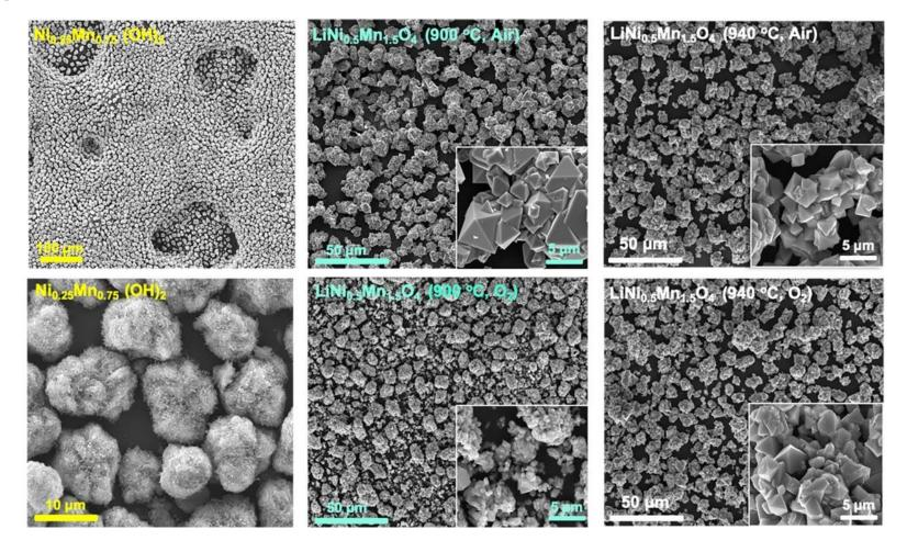
□ UT Austin has synthesized > 1 kg of Ni<sub>0.25</sub>Mn<sub>0.75</sub>(OH)<sub>2</sub> hydroxide precursor by coprecipitation in a 10 L tank reactor, with SEM micrographs depicted in SEM. The calcination temperature and lithium concentration has been optimized as well. 8
