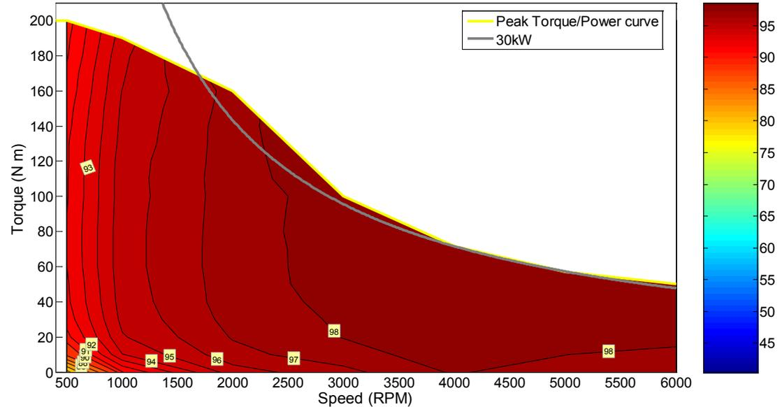
2011 Sonata - Combined Motor-Inverter Efficiency Contours
