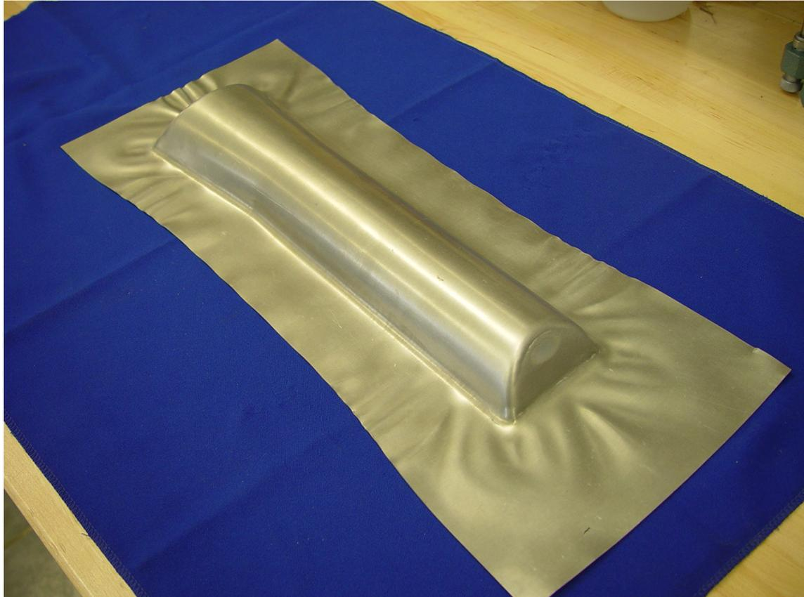
Picture of bottom of hot preformed X608 aluminum tray showing draw-in of sheet
