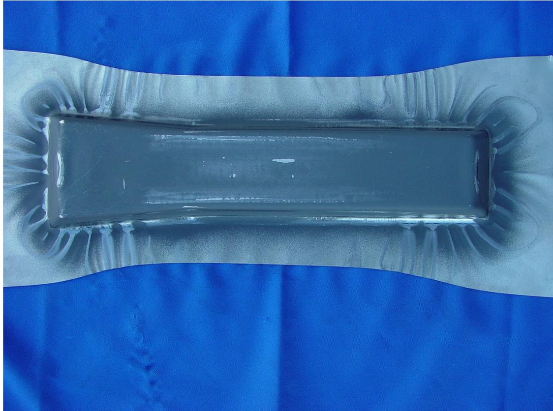
Picture of bottom of room temperature final formed X608 aluminum tray showing additional material draw-in of the sheet
