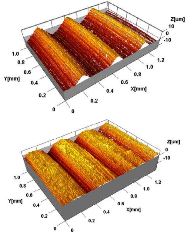
**Figure 8. False-Color 3D Image of Skirt Segment Showing As-Received Surface Texture (top) and Polished Texture (bottom) caused by Wear**
