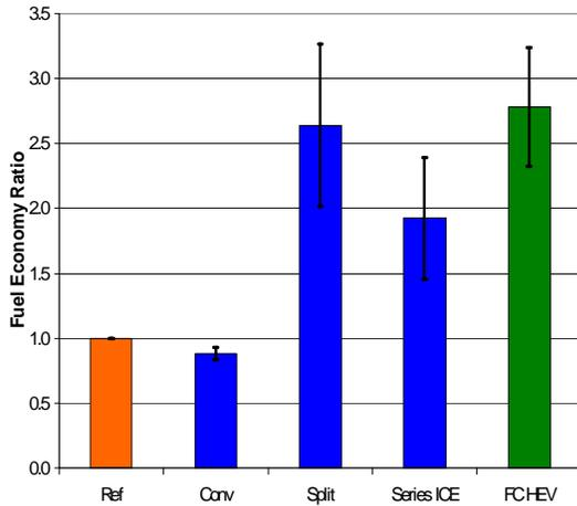
**Figure 3. Vehicle Fuel Economy Gasoline Equivalent Ratio – UDDS**
