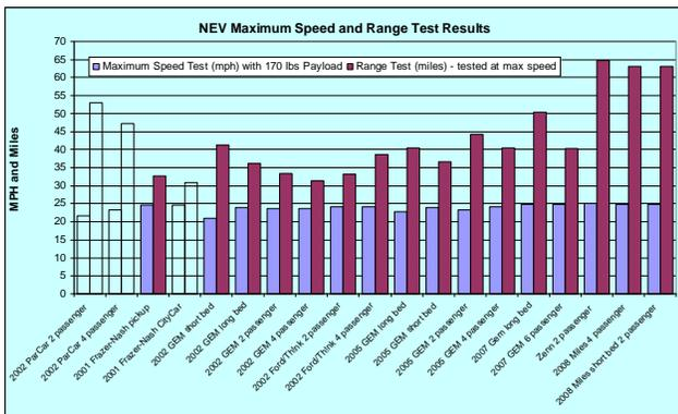
**Figure 1. NEV Maximum Speed as Tested on a Closed Test Track, with the accelerator pedal held to the floor (“brick test”) and the range per charge also conducted on a closed track during the “brick test” method**
