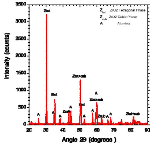
**Figure 6.** XRD pattern of ZT40A composite sample
