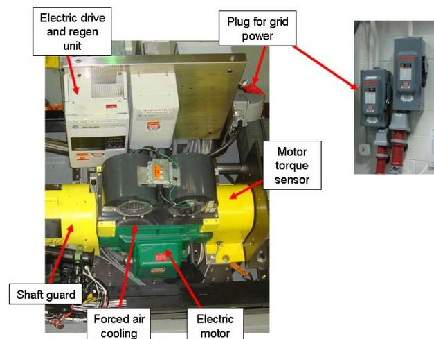
**Figure 8. Top view of virtual scalable motor module**
