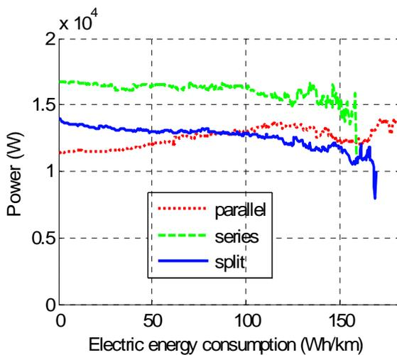
Figure 4. Average Engine Power When On (UDDS)
