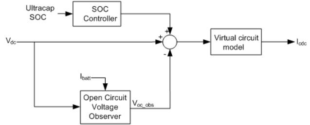
**Figure 5. Schematic of “Active Resistance” Circuit**
