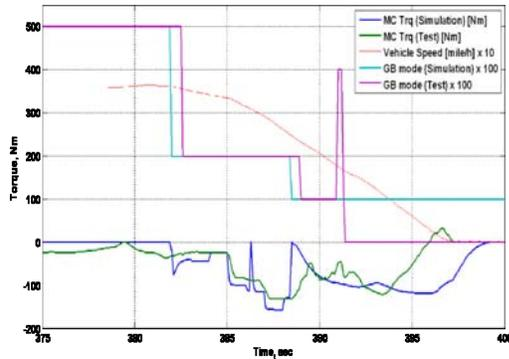
Figure 12. Regenerative Braking – Motor 1 - UDDS
