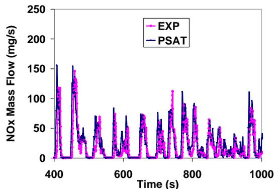
Figure 1. Example comparison between experimental measurements of engine-out NO<sub>x</sub> for the Saab flex-fuel vehicle (fueled with gasoline) and transient adjusted map-based predictions from PSAT. For visibility, the plot shows only a 600-second interval from a cold start UDDS drive cycle.
