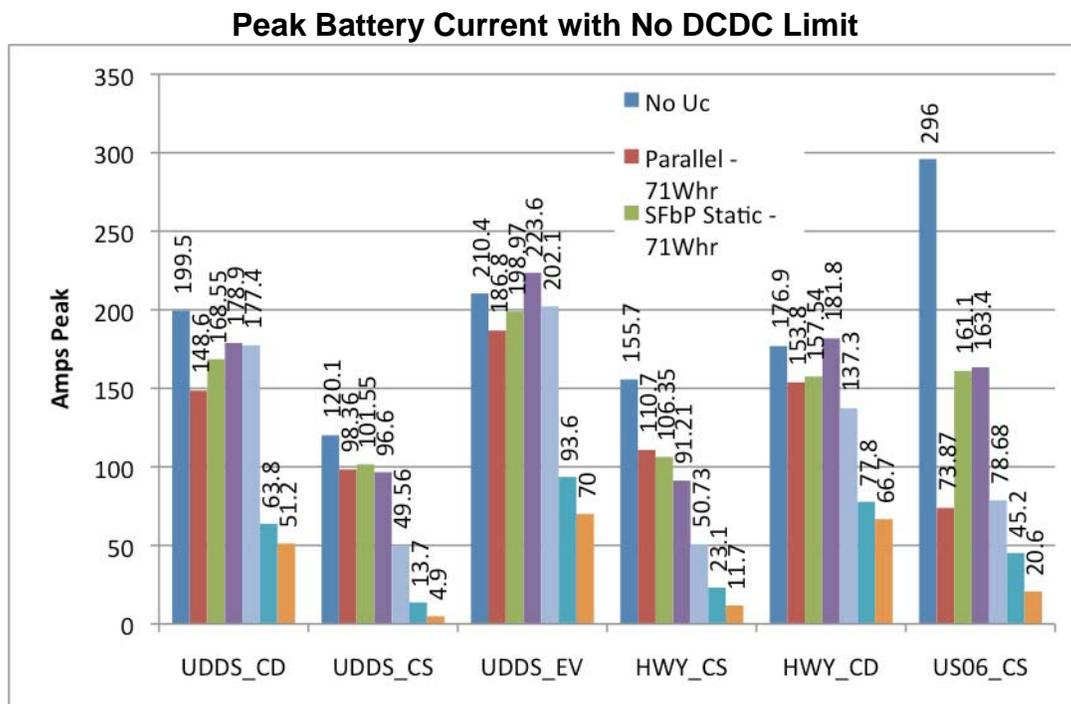
**Figure 23. Battery Current Limit with no DC/DC Limit**
