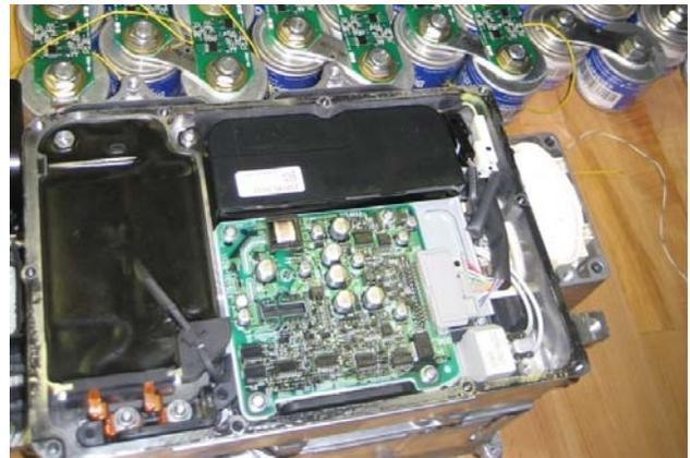
**Figure 12. Toyota Camry 35-kW DC/DC Converter**
