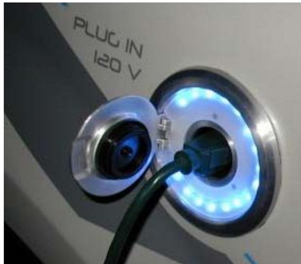
**Figure 2. Ford E85 PHEV Escape’s unique 120-Volt Charge Port Located in the Front Left Side Fender, in Use**
