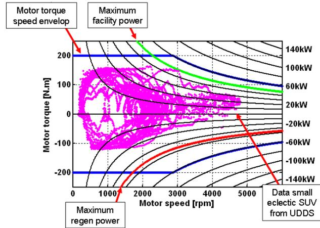
**Figure 10. Limits of the physical motor overlaid with the motor torque speed requirements for a small SUV on a UDDS**
