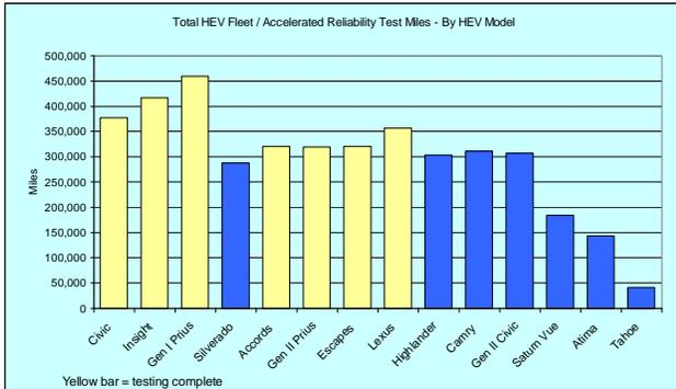
Figure 1. Total HEV Test Miles by Vehicle Model.
