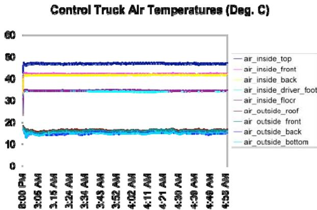
Figure 7. Measured Inside and Outside Truck Air Temperatures
