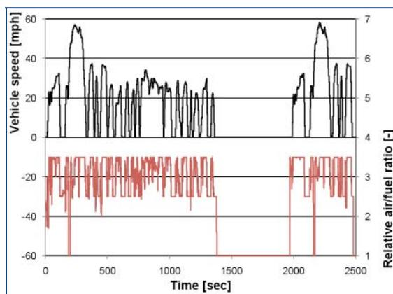
Figure 15. Relative Air/Fuel Ratio during FTP-75 Test
