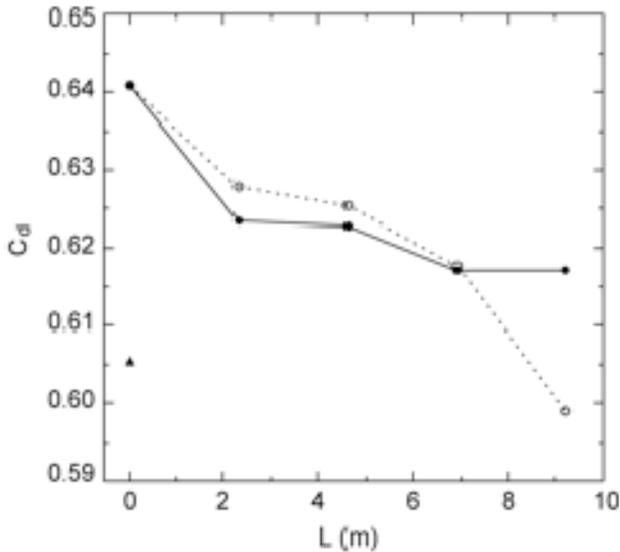
**Figure 5. Drag Coefficient of the Vehicle at 6.1° yaw, as a function of the fairing length for the T1 (solid line) and T2 (dashed line) fairings; drag coefficient of the vehicle with trailer side skirts, solid triangle.**
