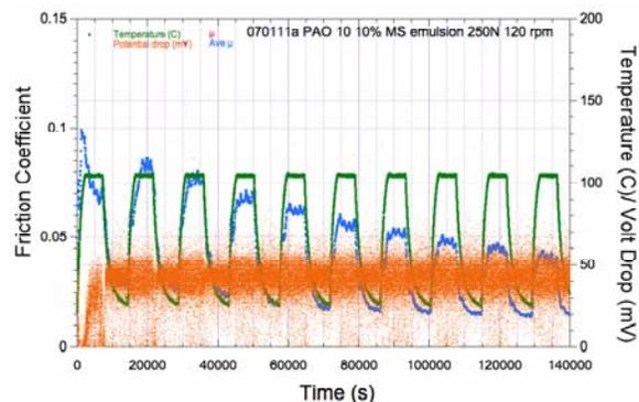
**Figure 3. Friction Response of Prototypic Heavy-Duty Ring and Liner Segments, during laboratory tests with PAO 10 and a commercial boric-acid-based additive. Blue: 20-point running average of friction; Green: temperature; and Orange: contact resistance.**
