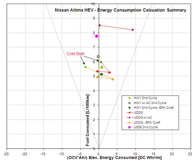
Figure 15. Altima Hybrid Fuel Consumption Dynamometer Testing Results
