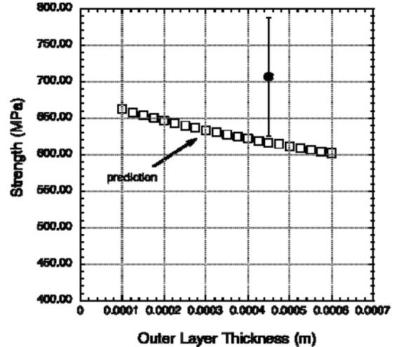
Figure 11. Comparison of experimentally measured flexural strength with the prediction for the layered structure as a function of the outer layer thickness
