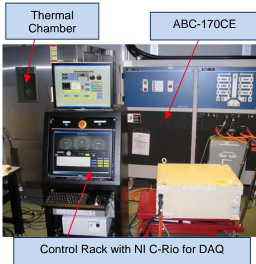
Figure 2. Battery HIL2 Test Facility
