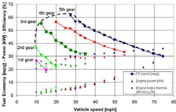
Figure 39. Conventional Vehicle Steady State Speed Results
