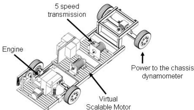
**Figure 1. Illustration of the Modular Automotive Technology Testbed**
