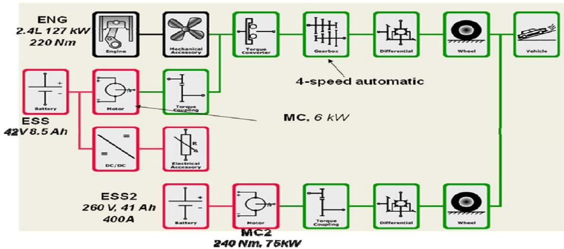
Figure 1. Vehicle Characteristics
