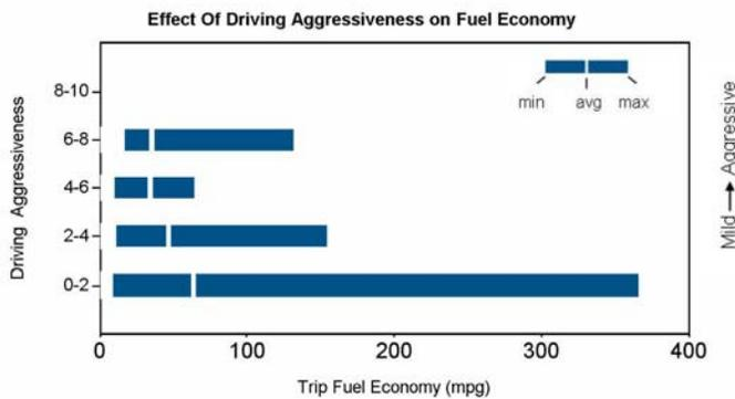
Aggressiveness factor is based on accelerator pedal position. The more time spent during a trip at higher accelerator pedal position, the higher the trip aggressiveness.
