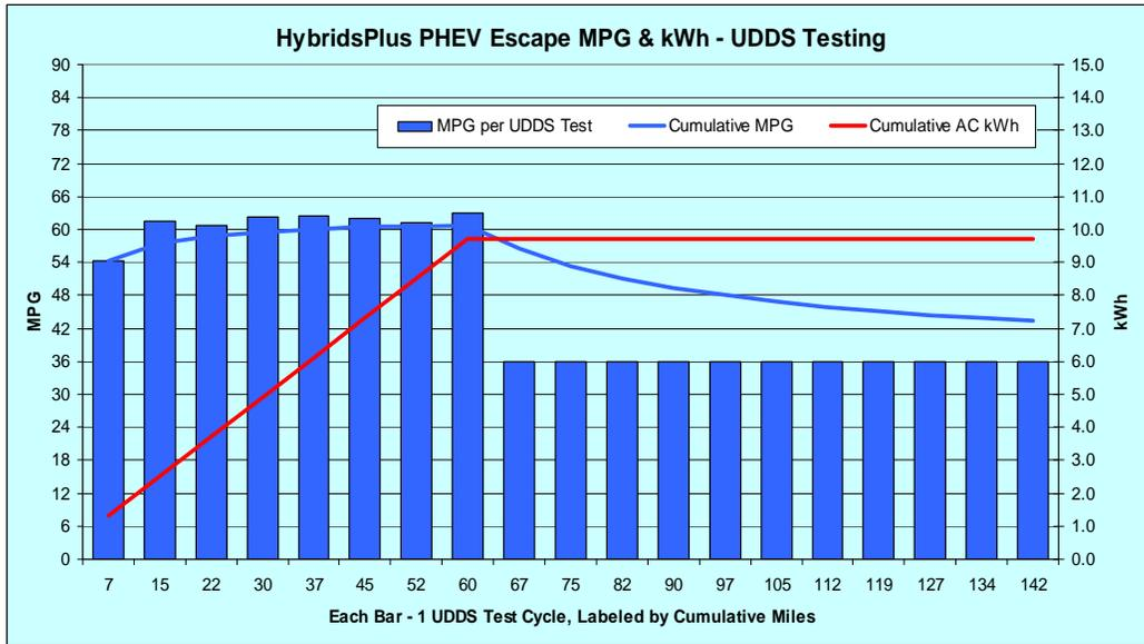
**Figure 19. Hybrids Plus Escape PHEV conversion UDDS testing results.**
