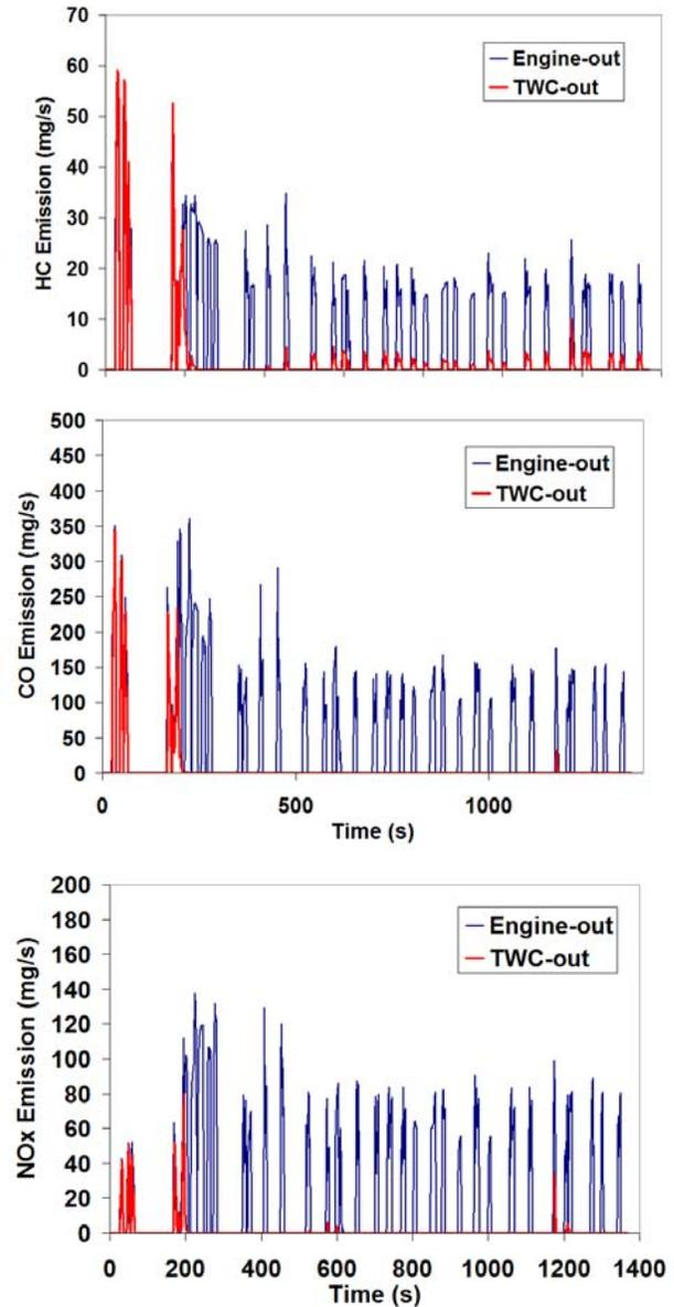
**Figure 3. Example PSAT HEV simulation results illustrating the impact of a 3-way catalyst on emissions. Blue indicates the engine out level and red indicates the catalyst out (tailpipe) level. The catalyst reduces cycle average emissions from 1.03 g HC/mi, 7.06 g CO/mi, and 3.13 g  $\text{NO}_x$ /mi to 0.29 g HC/mi, 1.14 g CO/mi, and 0.21 g  $\text{NO}_x$ /mi.**
