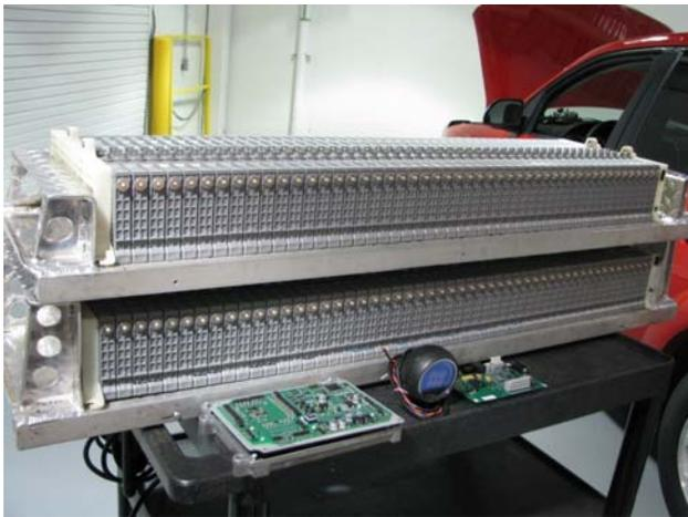
Figure 9. NiMH Battery Pack Configuration
