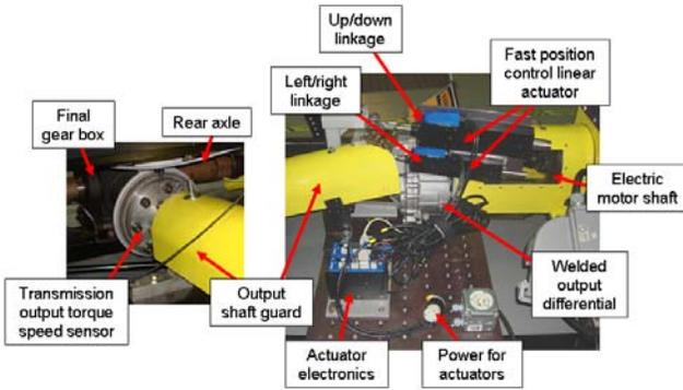
Figure 11. Manual Transmission Hardware
