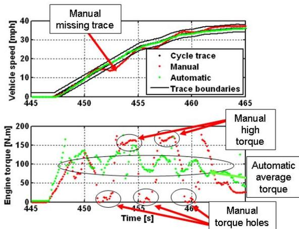
**Figure 14. Comparison of the Manual to the Automatic Transmission in Conventional Operation**
