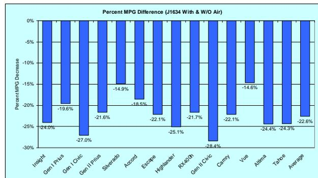
Figure 6. Percentage Decrease in Baseline Performance Fuel Economy Test Results for SAE J1634 Drive Cycle Testing when the Air Conditioning is Turned on during the Testing
