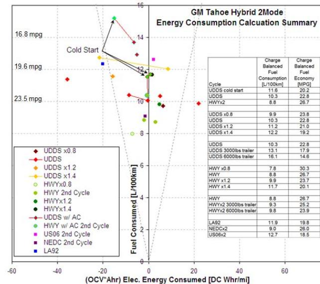
**Figure 3. Fuel Consumption Results of Tahoe Hybrid 2 Mode**
