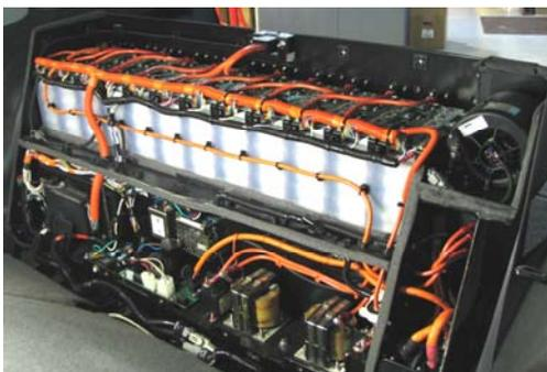
**Figure 6. Inside the Hymotion Escape Battery**
