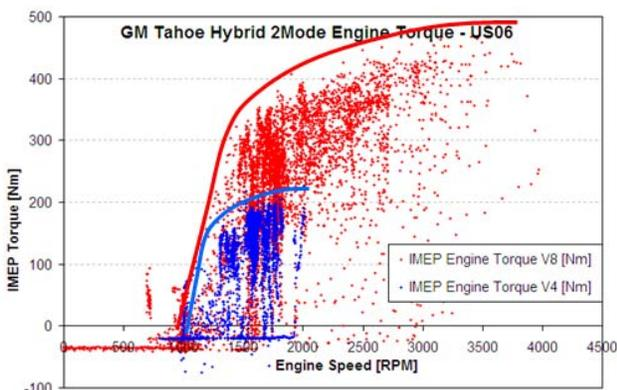
Figure 8. Engine Torque on a US06
