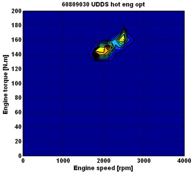
Figure 32. Engine Operation of the “Engine Optimum” Mode
