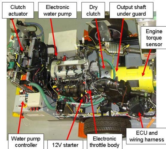
**Figure 3. Top View of the Gasoline Engine Module**
