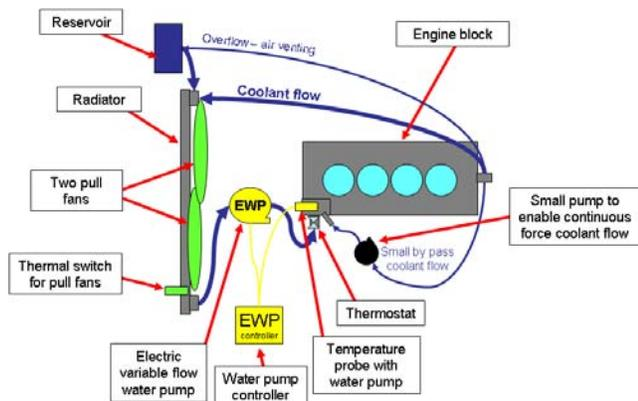
Figure 4. Schematic of Coolant System for the Engine
