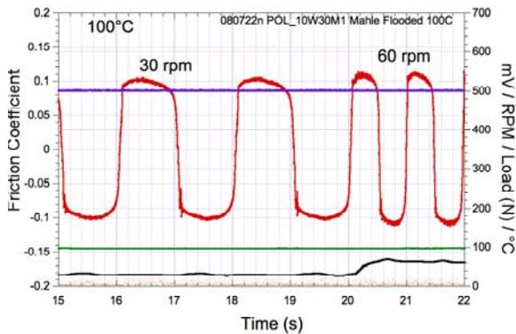
**Figure 7. Instantaneous Friction Response of Unmodified Piston Skirt Sliding on Liner, during laboratory tests with formulated synthetic engine oil (10W-30) at 100°C. Black – reciprocating speed; Purple – load; Red - friction; Green – temperature; and Orange – contact resistance.**
