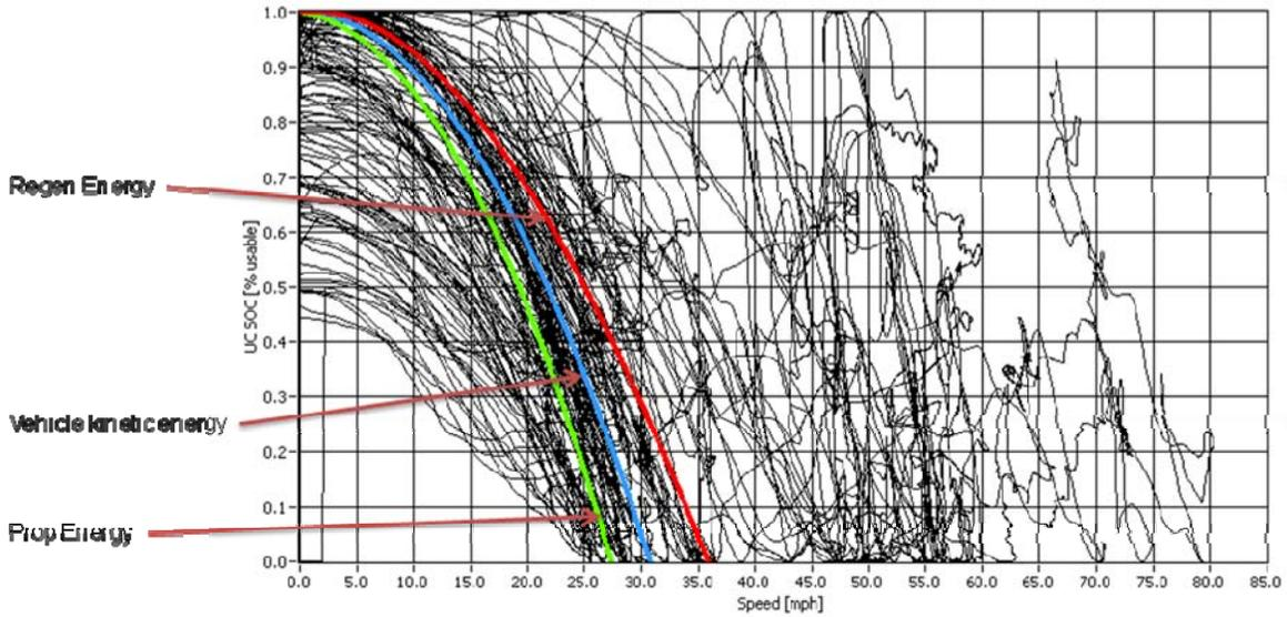
Figure 20. Demonstration of SOC and Vehicle Speed Correlation
