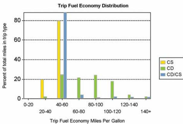
Figure 23. Page 2 of 3 for the PHEV Summary Report for 30 PHEVs operating January – June 2008 with onboard Kvaser data loggers
