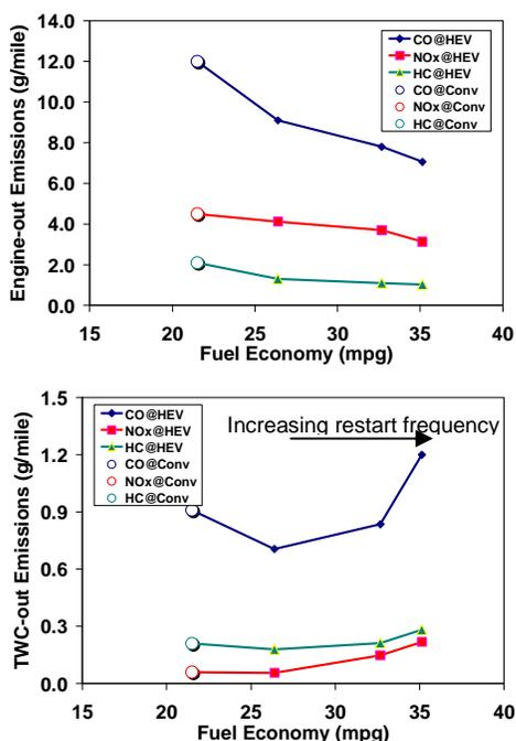
**Figure 4. Example PSAT HEV simulation results illustrating the effect of repeated engine starting on fuel economy and emissions. Cycle average emissions reach a minimum at an intermediate restart frequency where fuel economy is reduced.**
