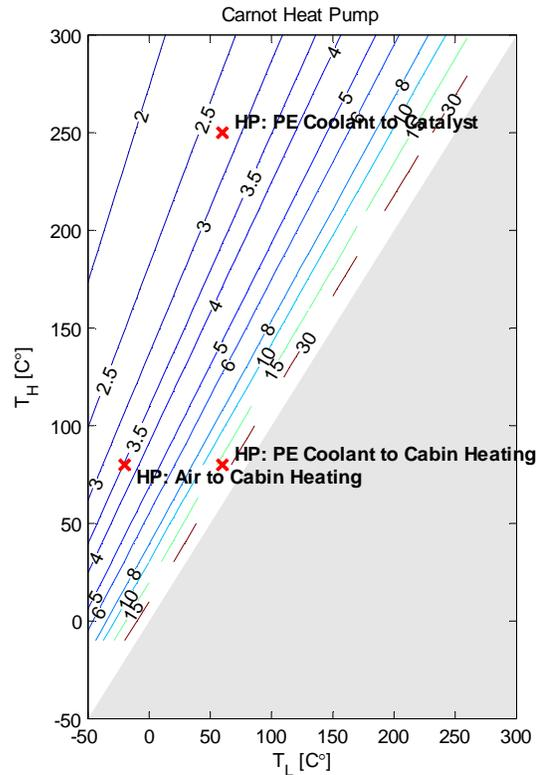
Figure 3. Carnot Heat Pump Coefficient of Performance
