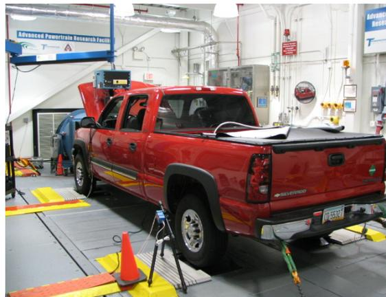
**Figure 1. Hydrogen-Converted Truck Undergoing Tests at the APRF**
