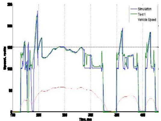
Figure 6. Engine Speed Comparison - UDDS
