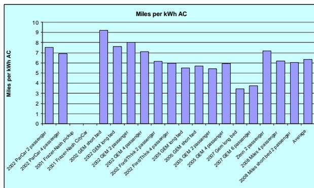
**Figure 5. NEV Vehicle Efficiency, as measured in miles per kWh AC when the vehicles are charged at 110 volts (Level 1 Charging). The two Frazier-Nash NEVs were charged at Level 3, and the 2002 data for charging efficiency are not available. The 17 other NEVs were all charged at 110 volts.**
