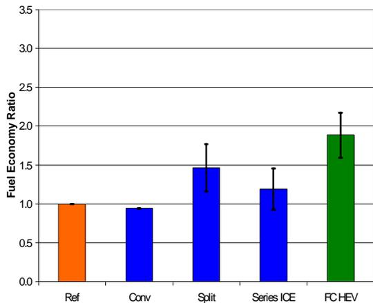
**Figure 4. Vehicle Fuel Economy Gasoline Equivalent Ratio – HWFET**
