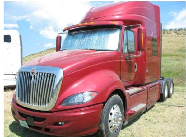
Figure 8. Insulated Windows on Test Truck
