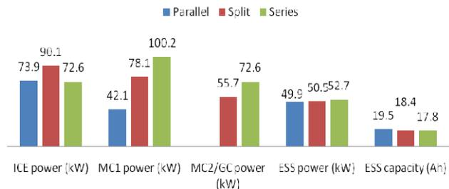
**Figure 2. Power and Battery Capacity of Components**
