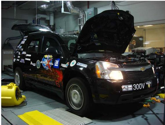
Figure 7. Hydrogen Fuel Cell HEV Test at the APRF
