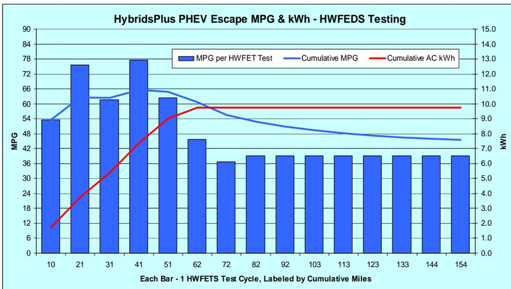
**Figure 20. Hybrids Plus Escape PHEV conversion HWFEDS testing results.**
