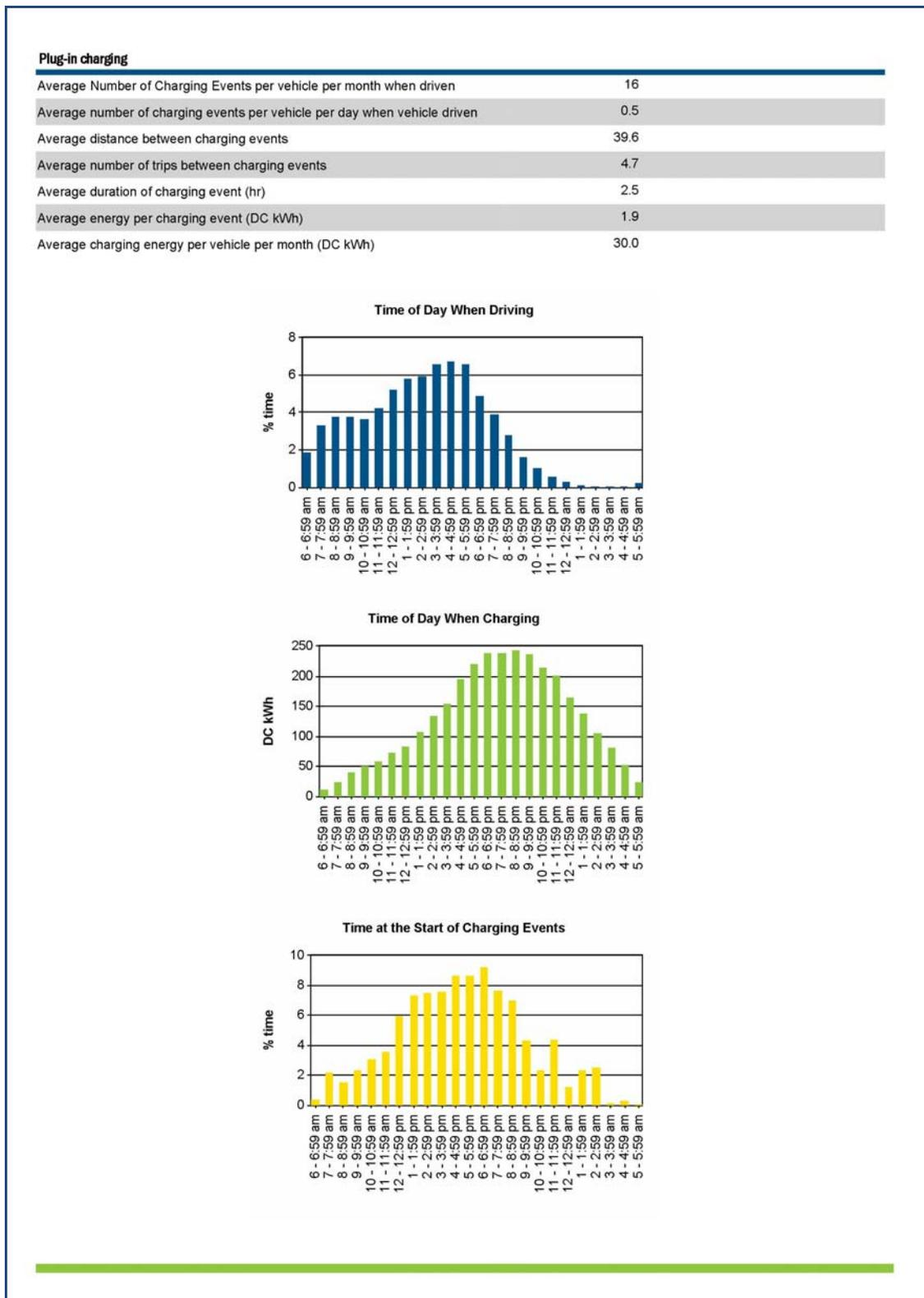
Figure 24. Page 3 of 3 for the PHEV Summary Report for 30 PHEVs operating January – June 2008 with onboard Kvaser data loggers
