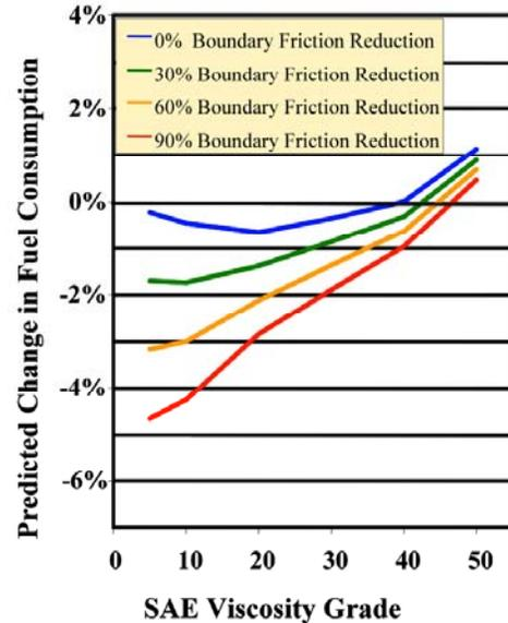
Figure 1. Graph of Predicted Change in Fuel Economy as a Function of Engine Lubricant Viscosity and Boundary Friction
