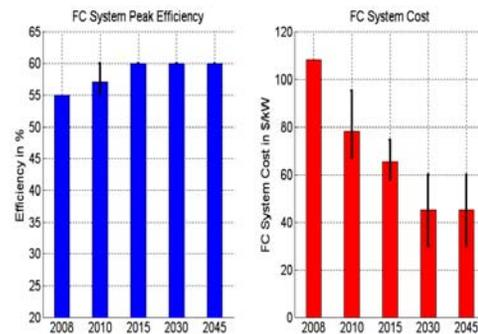
Figure 6. Fuel Cell System Efficiency and Cost
