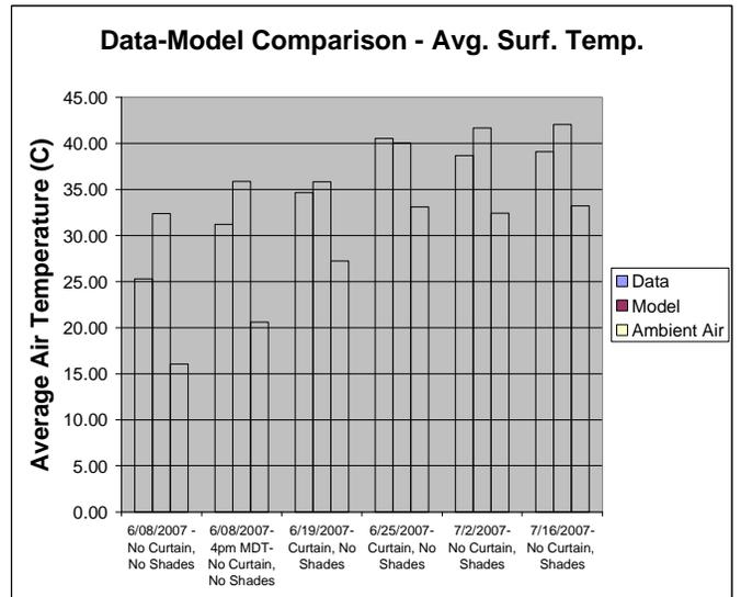
Figure 6. Model Surface Test Temperatures Compared to Test Data
