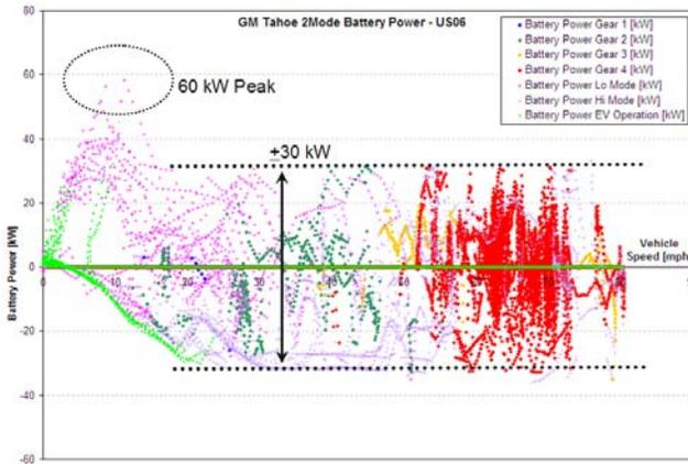
Figure 13. Battery Power over US06 Drive Cycle
