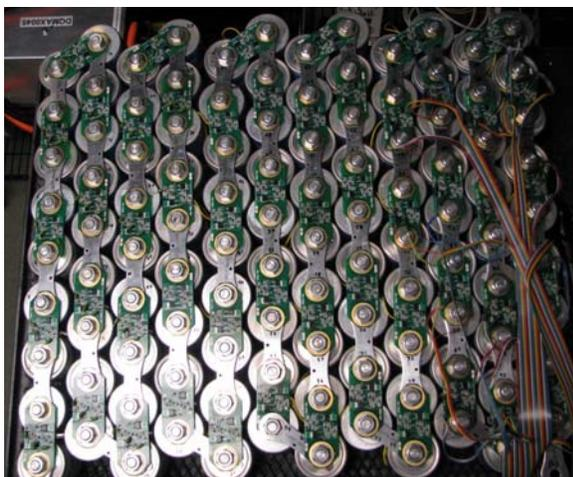
Figure 7. Top View of Ultracapacitor Array
