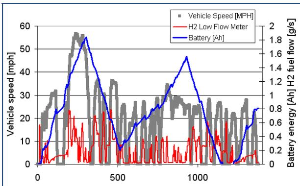
Figure 8. Battery Energy Usage and Fuel Flow on an Urban Cycle
