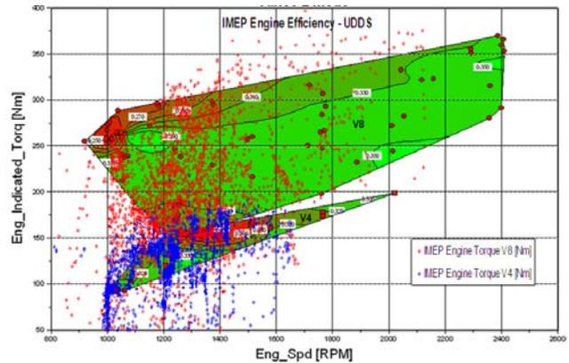
Figure 9. IMEP Engine Efficiency Map
