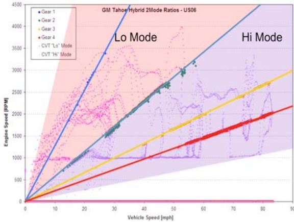
Figure 4. Operating Mode from Test Data
