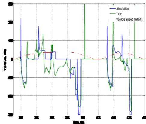
Figure 11. Motor 2 Torque Comparison - UDDS
