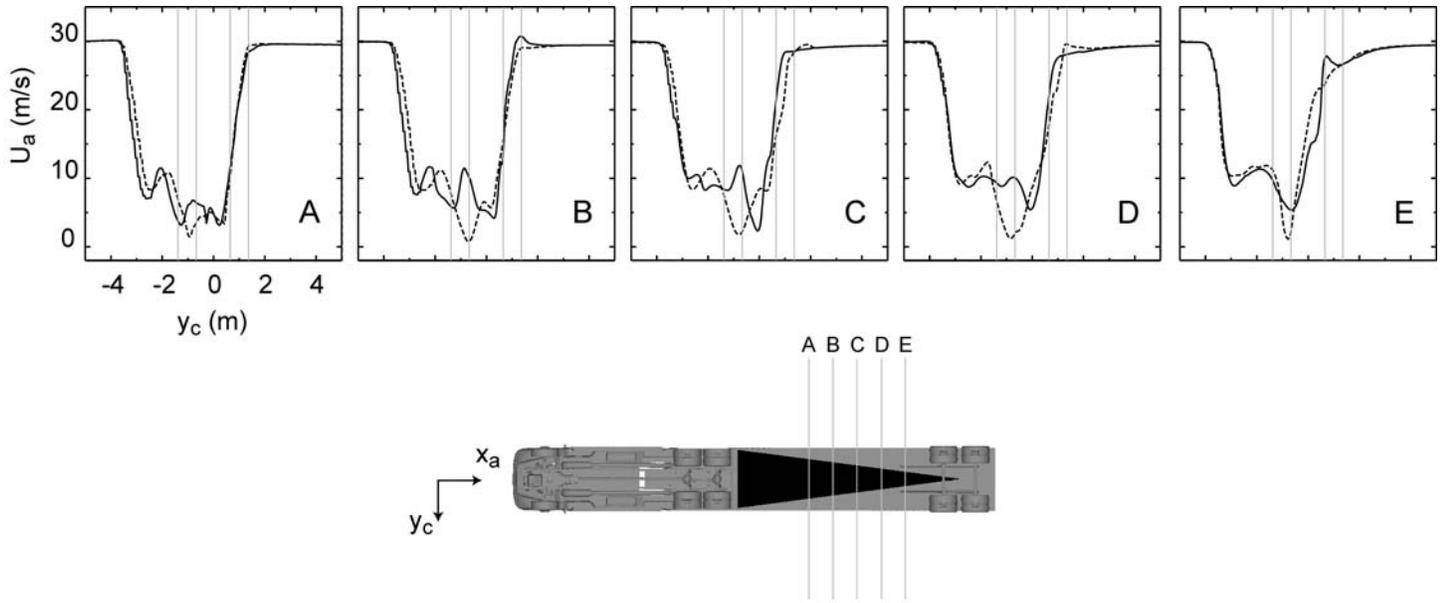
**Figure 9. Trailer underbody velocity profiles of  $U_a$  for the  $L = 9.2$  m T1 (solid line) and T2 fairings (dashed line). The profiles are located at  $z = 0.56$  m (axle height) with a 1 m spacing in the  $x_a$  direction ending 1 m upstream of the trailer tires. The grey vertical lines in each plot denote the edges of the windward and leeward trailer tires.**
