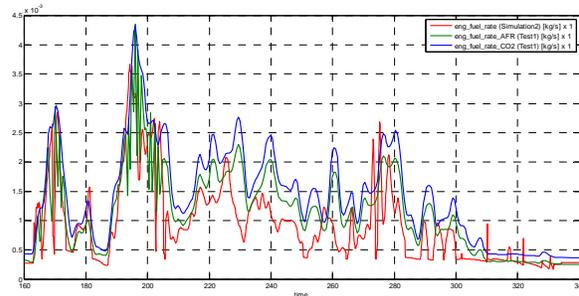
**Figure 3. Conventional Vehicle Engine Fuel Rate Comparison (AFR-based test data in blue, CO<sub>2</sub>-based test data in green, simulated data in red)**
