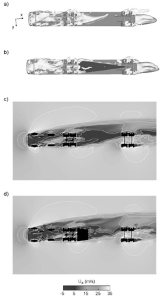
**Figure 6. Iso-surface of  $U_a = -0.001$  m/s for the a) baseline vehicle and the b)  $L = 9.2$  m T1 fairing configurations, where  $U_a$  is the component of velocity in the  $x_a$  direction (see Figure 1). b) Contours of  $U_a$  within a horizontal plane ( $z = 0.56$  m) that passes through the axes of the c) baseline vehicle and d)  $L = 9.2$  m T1 fairing configuration.**
