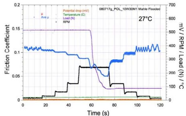
**Figure 5. Friction Response of Unmodified Piston Skirt Sliding on Liner, during laboratory tests with formulated synthetic engine oil (10W-30) at room temperature. Black – reciprocating speed; Purple – load; Blue – running average of friction; Green – temperature; and Orange – contact resistance.**
