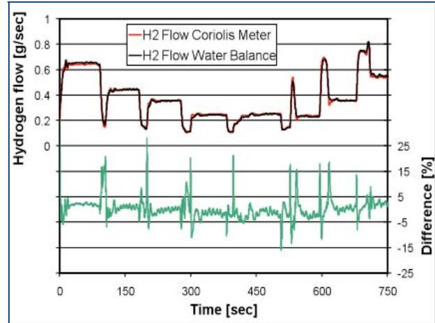
**Figure 12. Correlation between Fuel Consumption Measurement Methods for Steady-State Operating Points**
