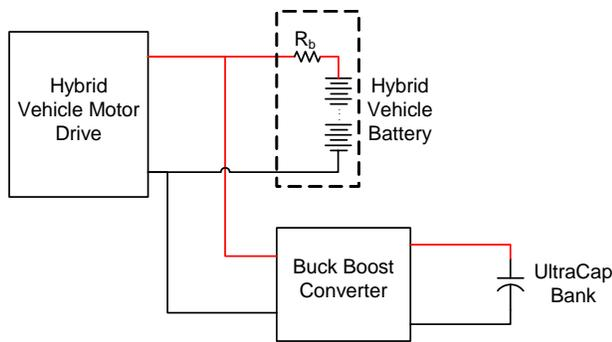
**Figure 4. DC/DC Converter Acting as an “Active Resistance”**
