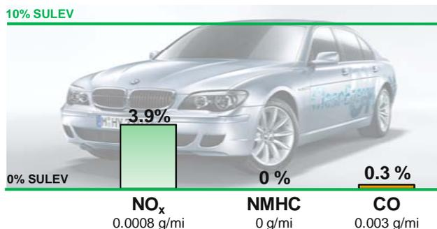
Figure 13. Hydrogen 7 Emissions Results Compared to SULEV Limits
