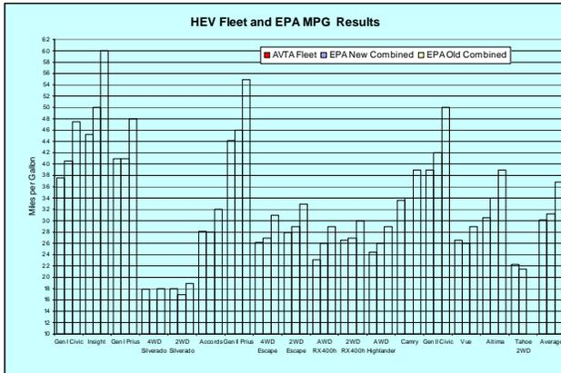
**Figure 9. Results for the AVTA Fleet Testing compared to the results for the old and new EPA mpg testing: The 14 HEV models are broken out into two-wheel, four-wheel, and all-wheel drive categories to match EPA vehicle categories.**
