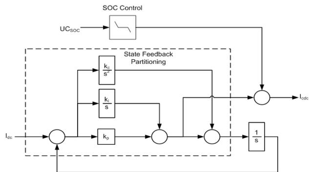
**Figure 6. State Feedback Partitioning**
