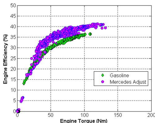
**Figure 5. Simulated engine efficiency comparison for diesel and gasoline HEVs. The points indicate instantaneous efficiency at different times in the drive cycle. The estimated diesel peak engine efficiency is 41% compared to 37% for the gasoline engine. Cycle average efficiencies are 36% versus 34%, respectively.**
