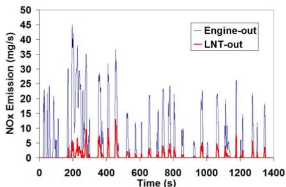
**Figure 6. Simulated impact of lean NO<sub>x</sub> control using an LNT on diesel HEV emissions. The LNT reduces NO<sub>x</sub> emissions by 87% but also results in a 2% fuel penalty.**
