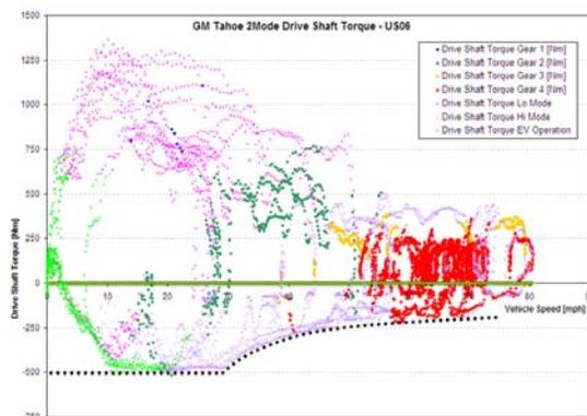
Figure 11. Driveshaft Torque over US06 Drive Cycle
