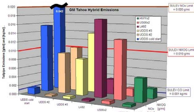
Figure 5. Tailpipe Emissions of Tahoe Hybrid
