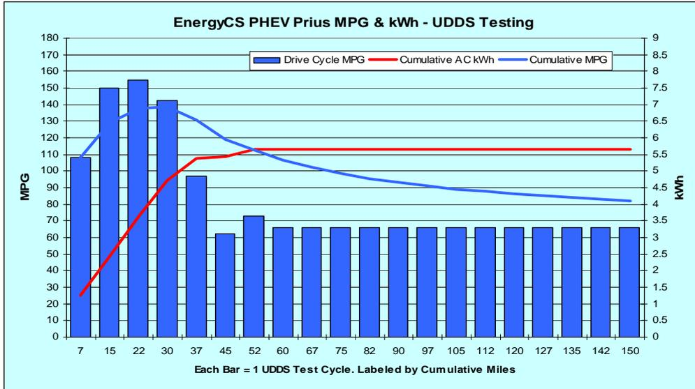
Figure 11. EnergyCS PHEV Prius conversion UDDS testing results. (The blue line is the cumulative mpg and the red line is the cumulative kWh use.)
