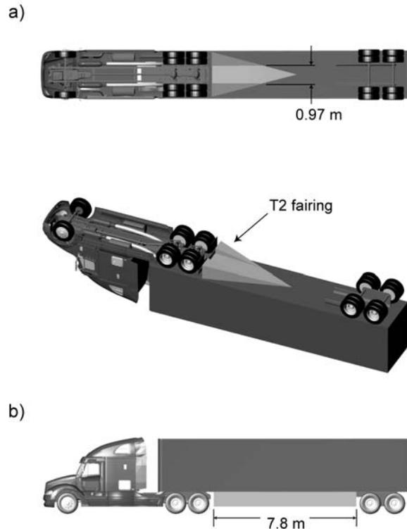
**Figure 3. a) T2 Fairing and b) Trailer Side Skirts Geometries**
