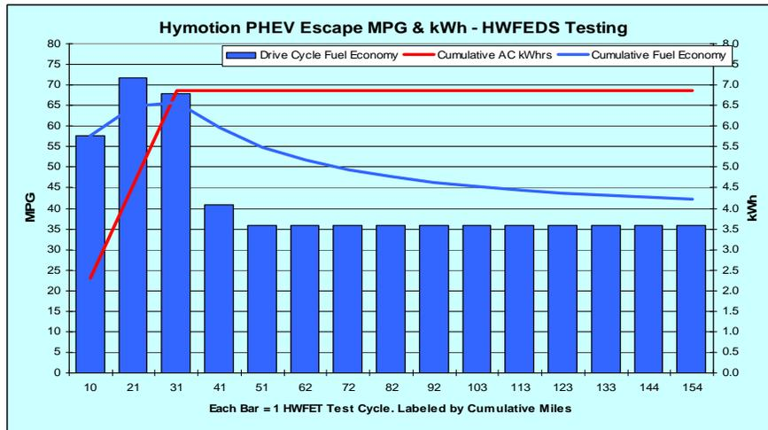
Figure 16. Hymotion Escape PHEV conversion HWFEDS testing results. (The blue line is the cumulative mpg and the red line is the cumulative kWh used.)
