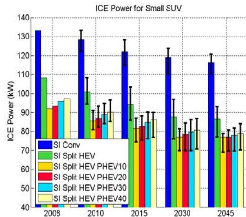
Figure 16. Engine Power for Gasoline Powertrains for Small SUV
