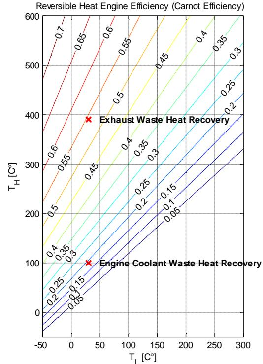
**Figure 2. Ideal Carnot Heat Engine Efficiency**
