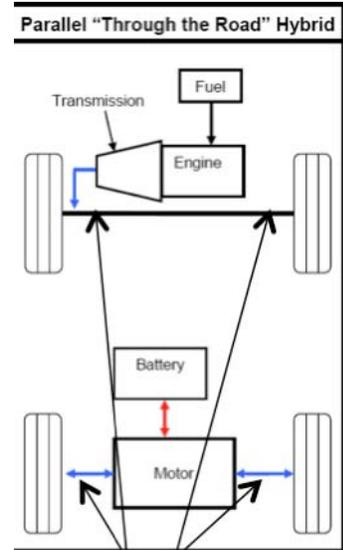
Axle Torque sensors on all 4 1/2-shafts to measure "through the road" power
