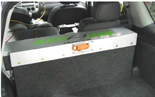
**Figure 5. Hymotion Escape Battery System**
