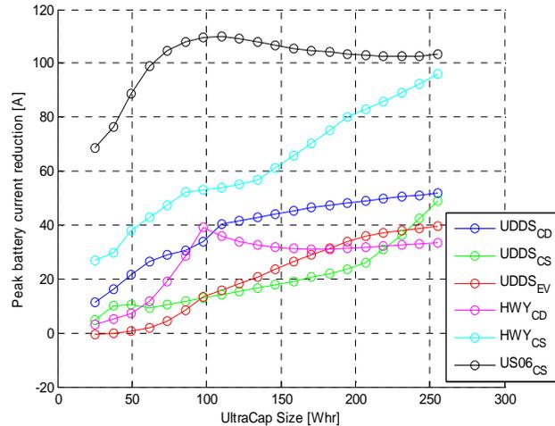
**Figure 14. Simulation Study of Capacitor Sizing**
