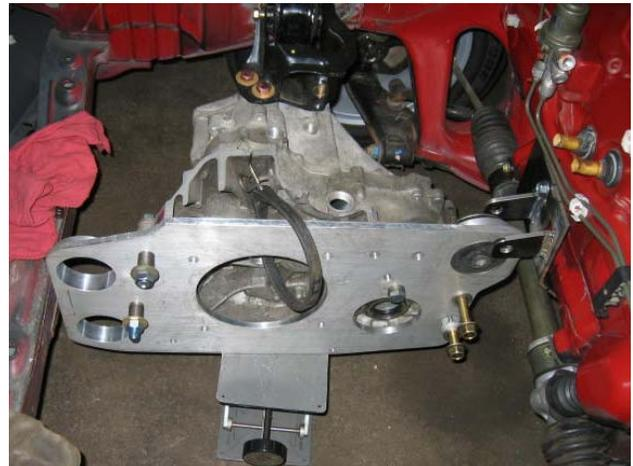
**Figure 16. Fabrication of Series Hybrid Powertrain Configuration**
