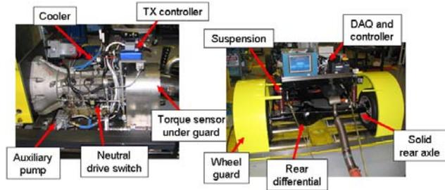
**Figure 13. Automatic Transmission Module and Rear End Hardware**
