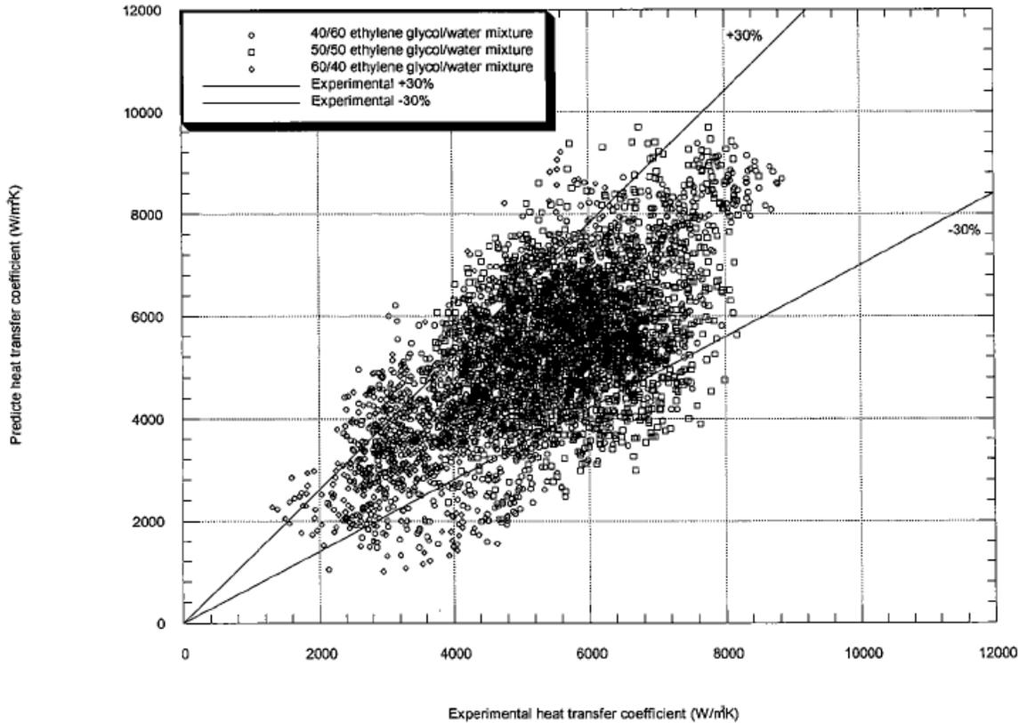
**Figure 6. Heat transfer coefficient comparisons (nucleation-dominant-boiling region)**
