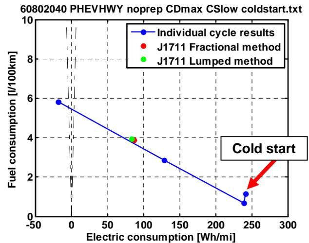
Figure 42. Energy and Fuel Consumption Summary for the Full-Charge Cold Start Test
