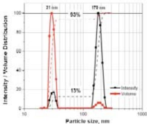
**Figure 3. Dynamic Laser Scattering results on SiC/water nanofluid**
