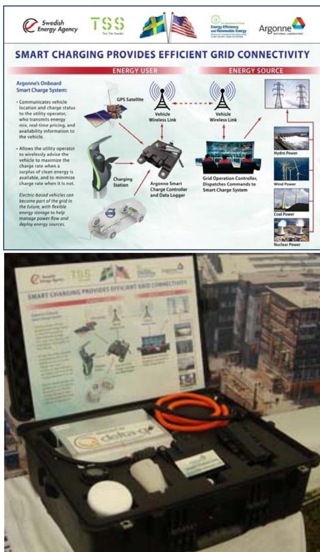
**Figure 11. Argonne-Designed Smart Charging System for a PHEV**
