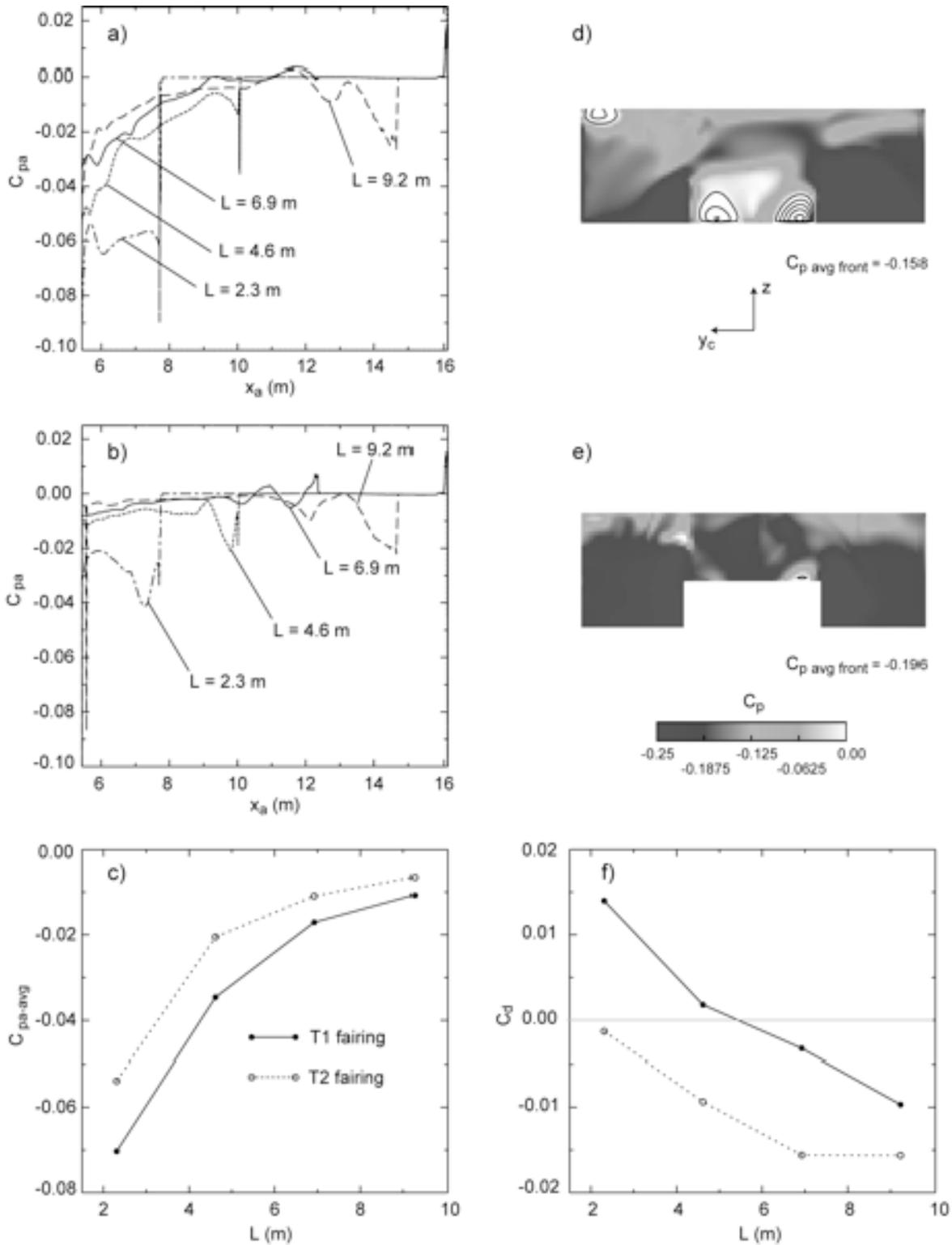
Figure 7. Distribution of  $C_{pa}$  along the centerline of the a) T1 and b) T2 fairings. c) Average pressure coefficient on the downstream facing surface of the T1 and T2 fairings as a function of the fairing length. Pressure coefficient contours on the front of the  $L = 6.9$  m d) T1 and e) T2 fairings. The contour lines indicate areas with positive values of  $C_p$ . f) Drag coefficient of the T1 and T2 fairings as a function of the fairing length.
