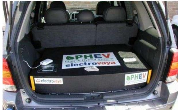
**Figure 8. Electrovaya Lithium Battery Pack in a Ford Escape converted by Electrovaya: The pack takes up the entire rear storage area.**
