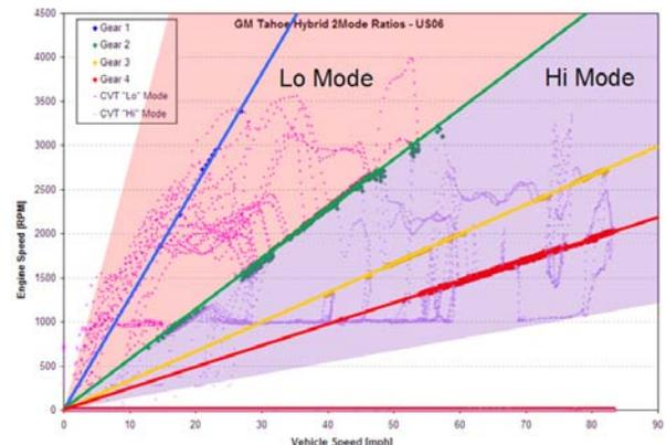
Figure 10. Transmission Ratio Utilization
