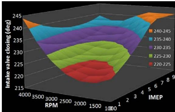
Figure 7. Camshaft Phasing Map
