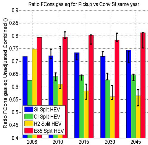
**Figure 23. Ratio of Fuel Consumption Gasoline-Equivalent Unadjusted Combined in Comparison to the Conventional Gasoline Same Year, Same Case, for Pickup**
