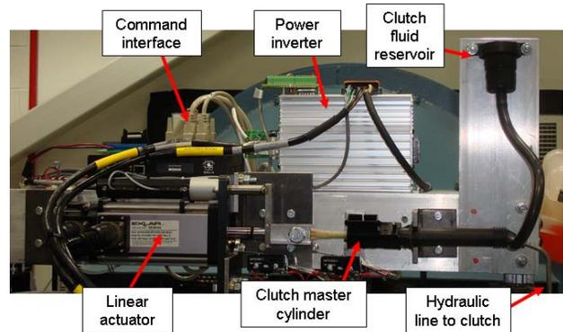
**Figure 7. Position control actuator system for the hydraulic clutch**
