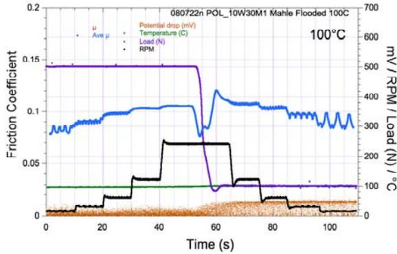
**Figure 6. Friction Response of Unmodified Piston Skirt Sliding on Liner, during laboratory tests with formulated synthetic engine oil (10W-30) at 100°C. Black – reciprocating speed; Purple – load; Blue – running average of friction; Green – temperature; and Orange – contact resistance.**
