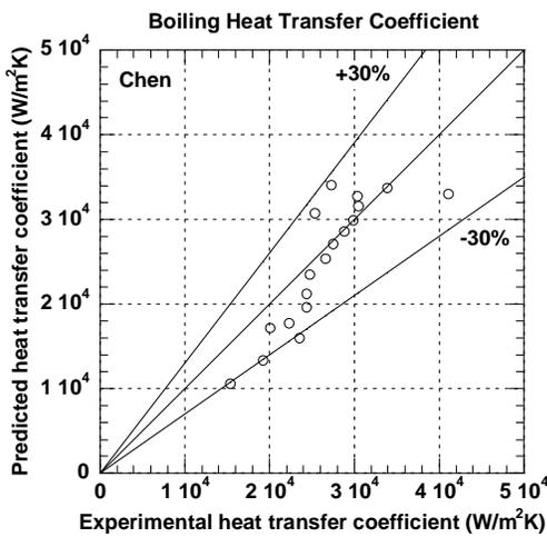
Figure 10. Heat transfer coefficient comparisons
