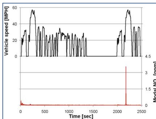
Figure 16. Modal NO<sub>x</sub> Emissions During FTP-75 Test
