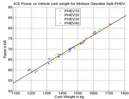
**Figure 6. Engine Power as a Function of Vehicle Weight for Different AER**
