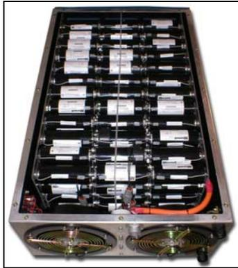
Figure 10. Maxwell Ultracapacitor Pack
