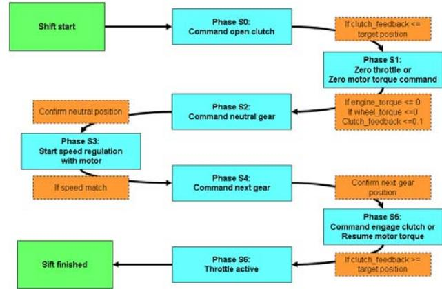
Figure 12. Manual Transmission Lower-Level Shifting Algorithm
