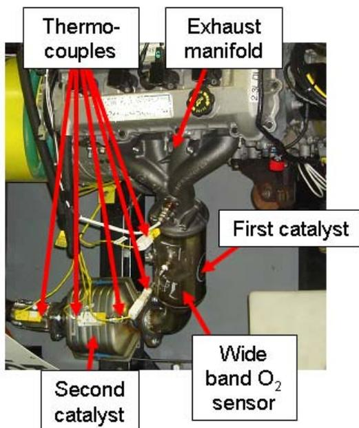
Figure 5. The Engine Exhaust Setup and Instrumentation
