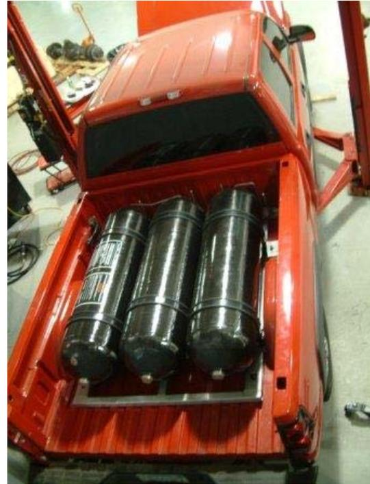
**Figure 2. Dynetek Hydrogen Fuel Tanks in the Bed of the Pickup**
