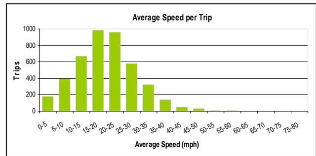
**Figure 4. Average Speed per Trip for the Eight Hydrogen ICE Vehicles at IWHUP**
