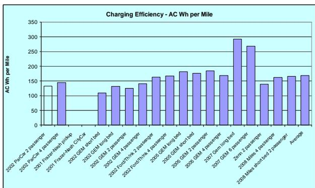
**Figure 4. NEV Charging Efficiency, in AC Wh per mile, for the 17 NEV models. The two Frazier-Nash NEVs were charged at Level 3, and the 2002 data for charging efficiency are not available. The 17 NEVs were all charged at 110 volts (Level 1 charging).**
