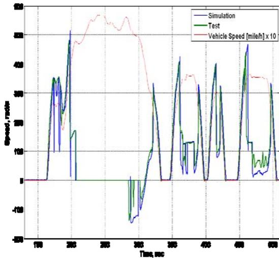
Figure 8. Motor 1 Speed Comparison - UDDS
