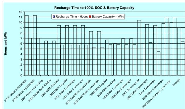
**Figure 2. NEV Recharge Times to 100 percent state of charge (SOC) and battery capacity for each NEV: All testing results are for 110 volt charging (Level 1 Charging). The time to recharge for the two Frazier-Nash NEVs is not given because these vehicles were charged by a Level 3 charger. The Frazier-Nash sedan was recharged in 0.93 hours and the pickup was recharged in 0.97 hours.**
