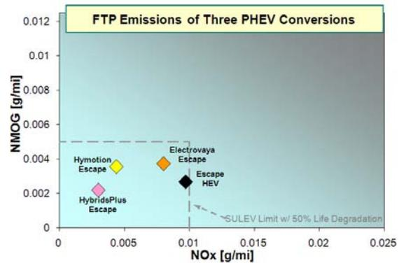
**Figure 11. Tailpipe Emissions of Three Escape PHEVs Conversions**
