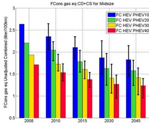
**Figure 8. Fuel Consumption (Gasoline Equivalent, Unadjusted Combined) for Fuel Cell PHEVs Midsize Cars (Note: The Fuel Consumption Values are CD+CS)**
