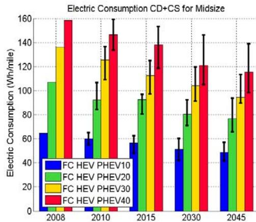
**Figure 9. Electric Consumption in CD+CS for FC PHEVs Midsize Vehicles**
