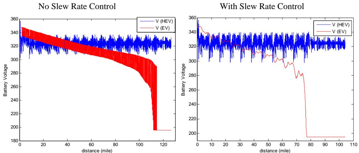
Figure 2. PHEV with dual battery control strategy
