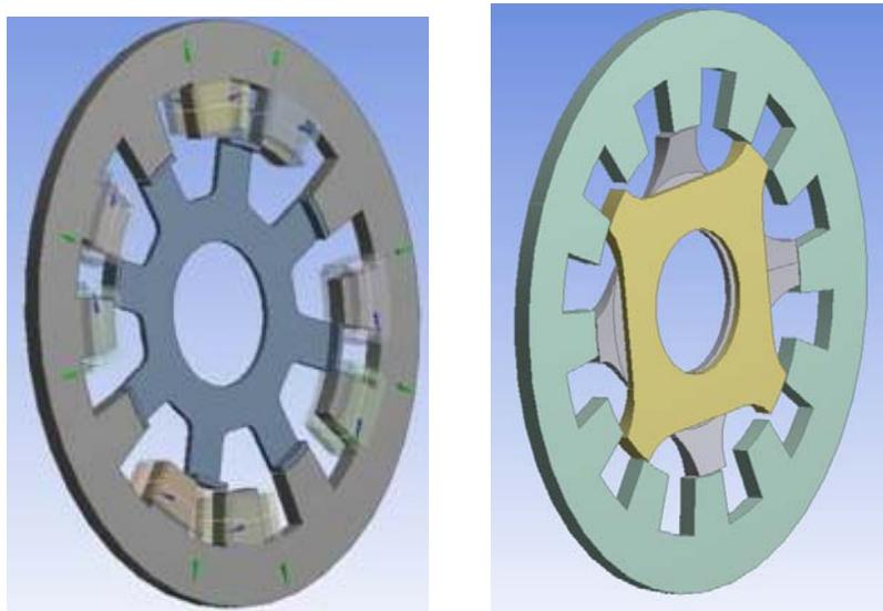
Fig. 5. Infeasible, yet informative applications of lamination taper.
