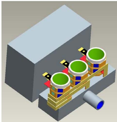
**Fig. 5. Two-chip-deep annulus design.**
