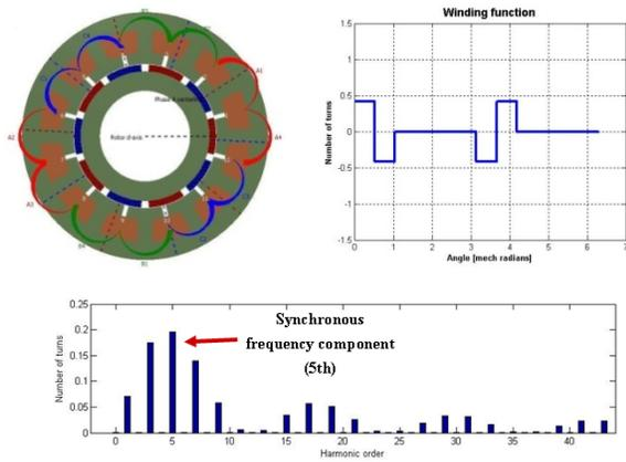
Fig. 1. Three phase (3P) machine: 12 slots/10 poles.
