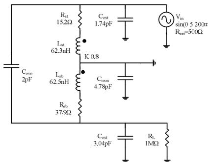
**Fig. 22. Lumped analytical model for stacked transformer.**
