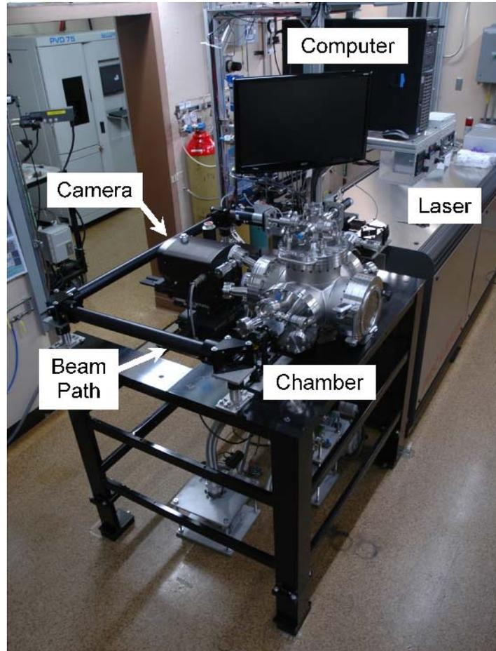
**Fig. 3. Solvent-LHFZ system featuring growth chamber, high power CO<sub>2</sub> laser, beam path, long range optical microscope camera, and automation/data collection computer.**
