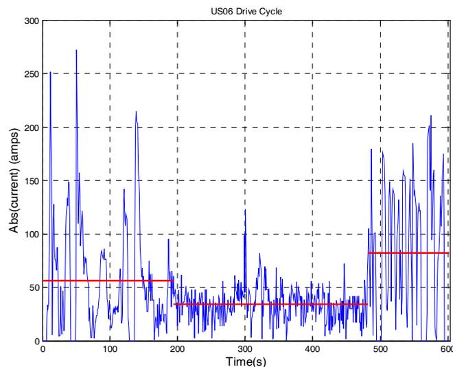
**Fig. 7. Current distribution from the US06 drive cycle.**
