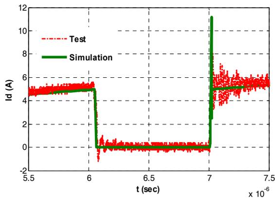
Fig. 29. Comparison of current waveforms of the JFET.
