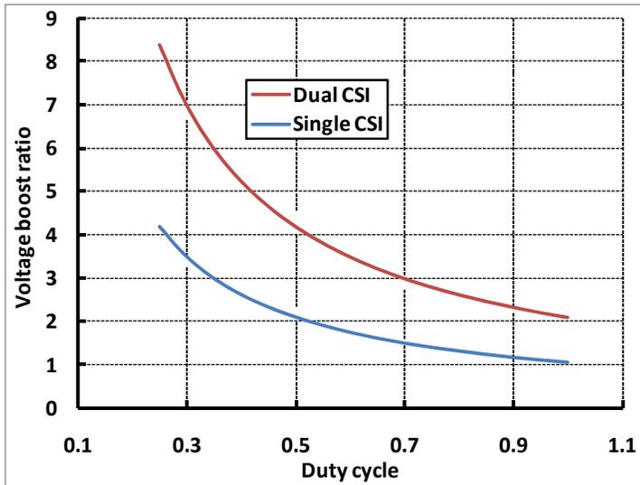
Fig. 3. Voltage boost ratio vs CSI duty cycle.
