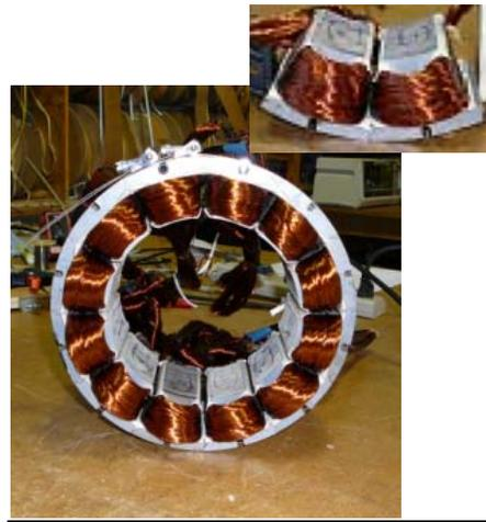
Fig. 2. Stator of the first proof-of-principle machine
