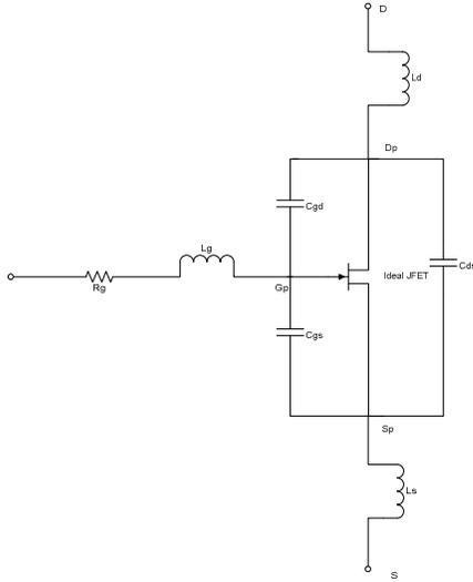
Fig. 23. Equivalent circuit of a SiC JFET.
