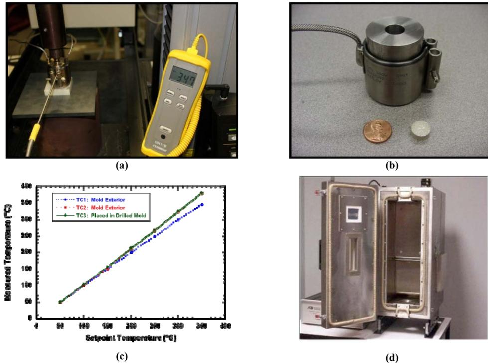
**Fig. 8. Silver sintering technology development for die and substrate attach: (a) ORNL model sintering facility, (b) fixture and sintered silver disk, (c) temperature validation, and (d) furnace for module-level fabrication.**
