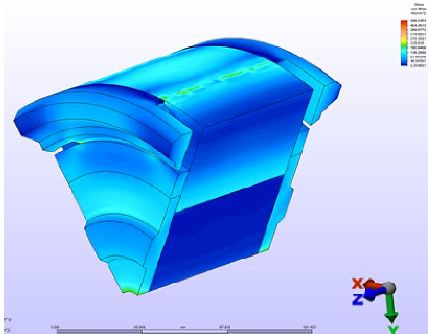
Fig. 10. Maximum Rotor Assembly Stress at 14,000 rpm = 65,122 psi.
