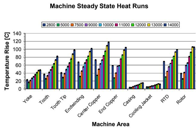
**Fig.8. First proof-of-principle machine heat runs temperature rises in the various machine components at various speeds.**
