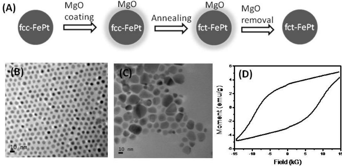
**Fig. 12.** (A) Schematic illustration of the synthesis of fct-FePt nano-particles; (B) TEM image of the 7 nm fcc-Fe<sub>60</sub>Pt<sub>40</sub> nano-particles; (C) TEM image of the fct-FePt nano-particles after MgO removal; (D) room temperature hysteresis loop of the fct-FePt nano-particles.
