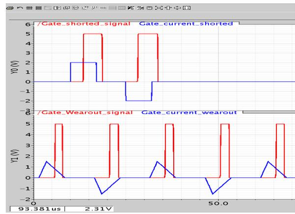
Fig. 29. Gate wear and gate shorted situation.
