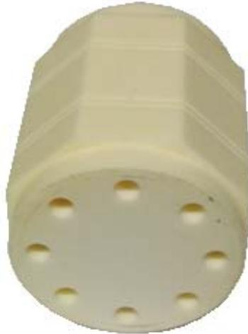
**Fig. 9. Finished alumina octagonal substrate fabricated by CoorsTek.**
