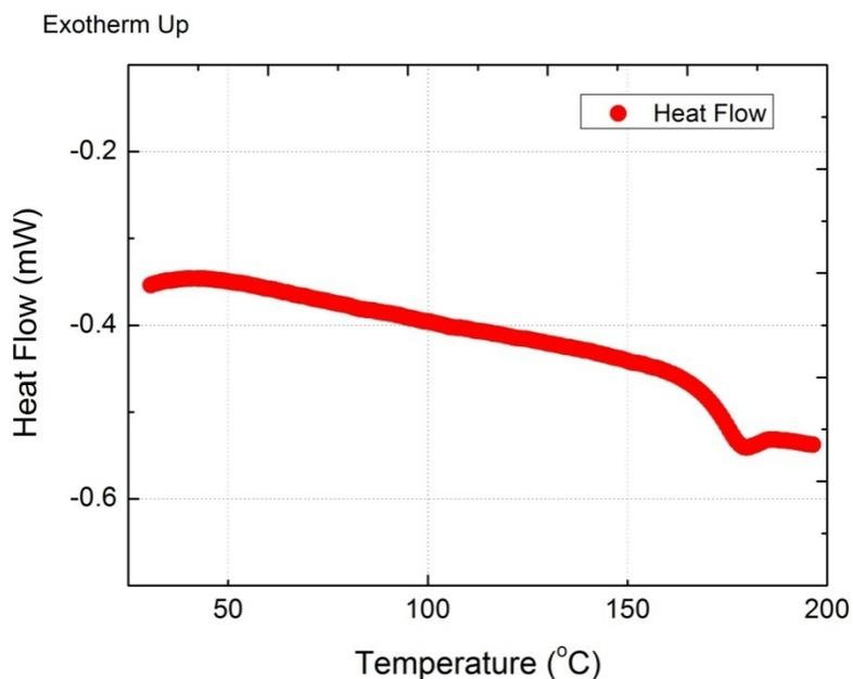
**Fig. 6. DSC data on polymer 2 where  $n = 3m$**
