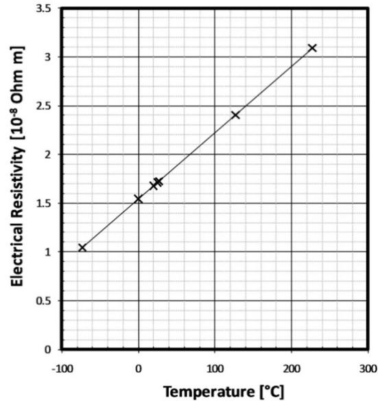
Fig. 28. Electric resistivity vs. temperature for pure copper [13]
