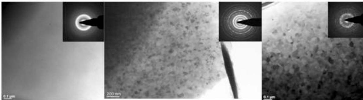
Fig. 4. TEM bright field images with corresponding electron diffraction patterns of (left) NO-121-B (as-spun), (middle) NO-121-B-2 (580°C/60min., 110MPa), and (right) NO-121-B-3 (580°C/60min., no applied pressure).
