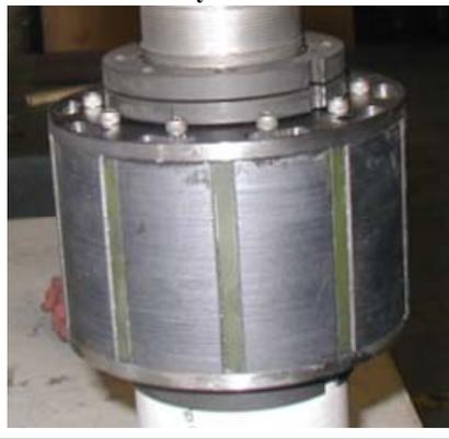
Fig. 3. Rotor of the first proof-of-principle machine
