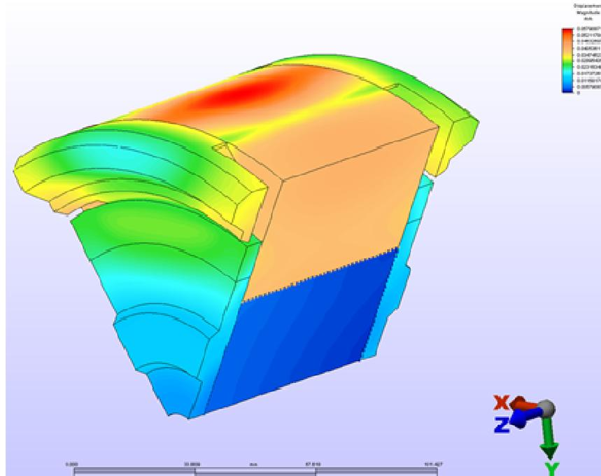
Fig. 11. Maximum rotor assembly displacement at 14,000 rpm = 0.002 in.
