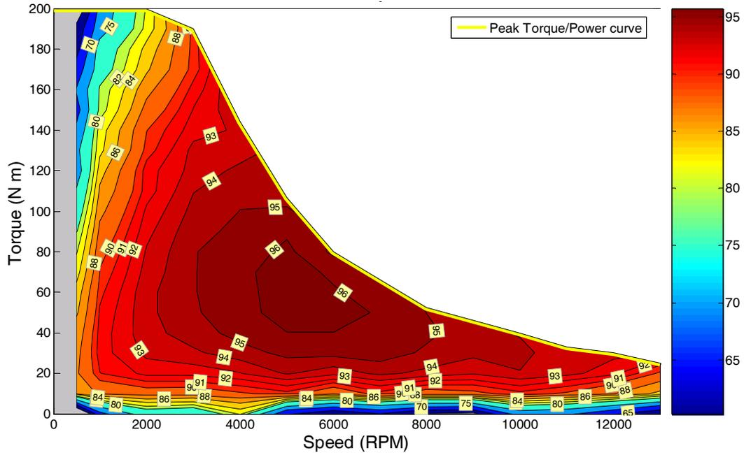
Fig. 11. 2010 Prius motor efficiency map for 650 Vdc.
