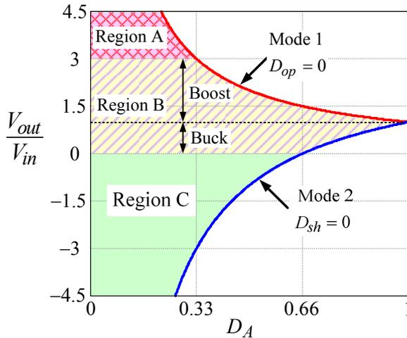
Fig. 10. CF-trans-ZSI and CF-trans-qZSI dc output voltage gain.
