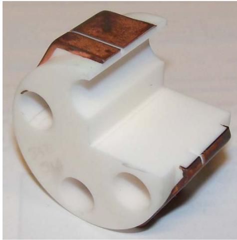
**Fig. 7. Sectioned part used for copper bond evaluation.**
