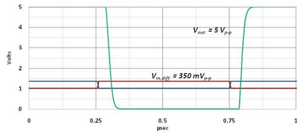
Fig. 18. Corinth LVDS receiver simulation at 200°C.
