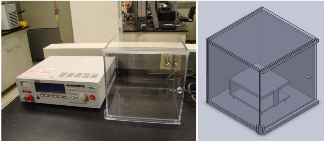
**Fig. 56. Dielectric resistance tester.**
