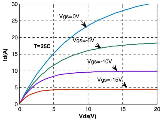
Fig. 27. Simulated forward characteristics of the SiC JFET.
