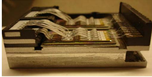
**Fig. 5. Cross-section of boost converter modules 2010 Prius.**
