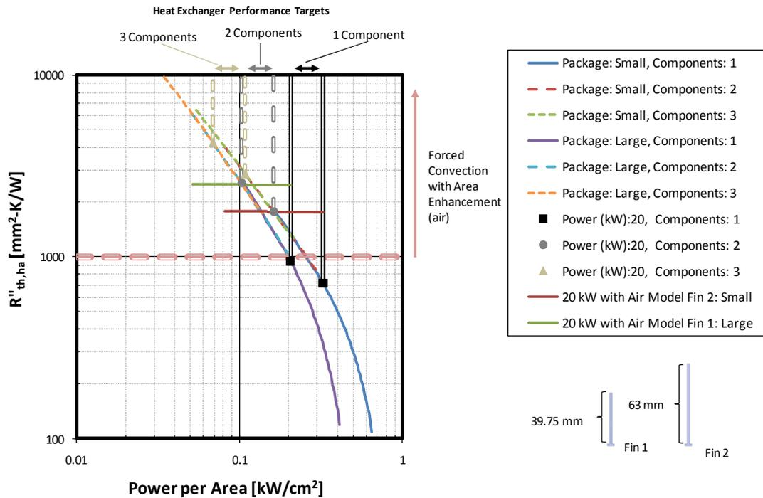
Fig. 6. Example system analysis, air-cooled 20 kW DC-DC converter for vehicle charging application
