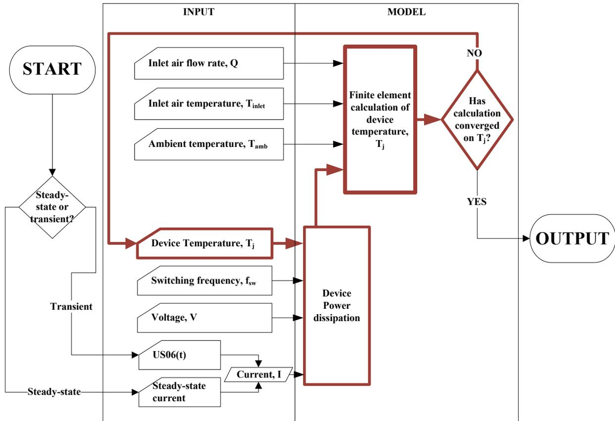
Fig. 1. Flowchart outlining junction temperature iterative procedure.
