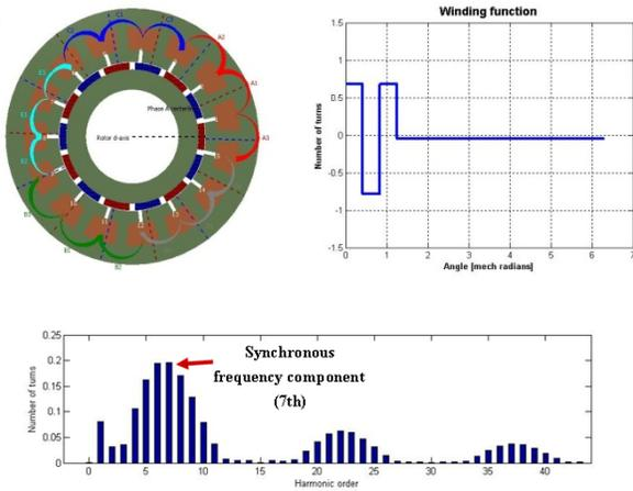
Fig. 3. Five phase (5P) machine: 15 slots/14 poles.
