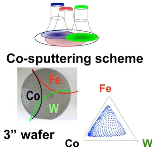
Fig. 10. Schematic of combinatorial synthesis experiment to generate composition field of Co-Fe-W.
