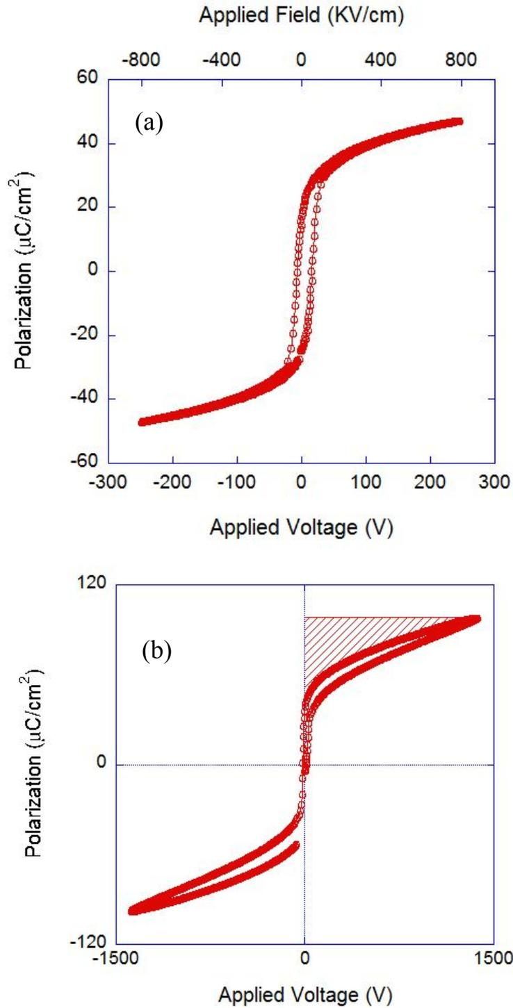
Fig. 7. Hysteresis loop of a  $\approx 3\text{-}\mu\text{m}$ -thick PLZT/LNO/Ni film-on-foil measured at room temperature with applied field of (a) 250 V and (b) 1400 V.
