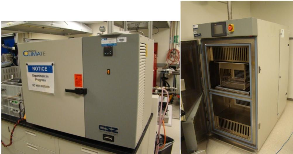
Fig. 57. CSZ MicroClimate (left) and VTS Compact Thermal Shock Chamber (right)
