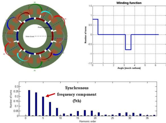
Fig. 4. Six phase (6P) machine: 2 slots/10 poles.
