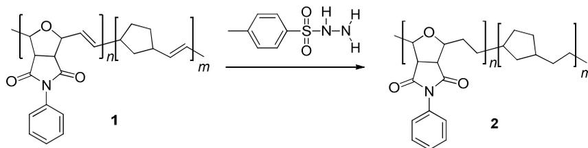
**Fig. 5. Hydrogenation of a model polymer dielectric**
