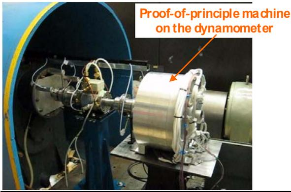
Fig. 1. Proof-of-principle machine on the dynamometer.
