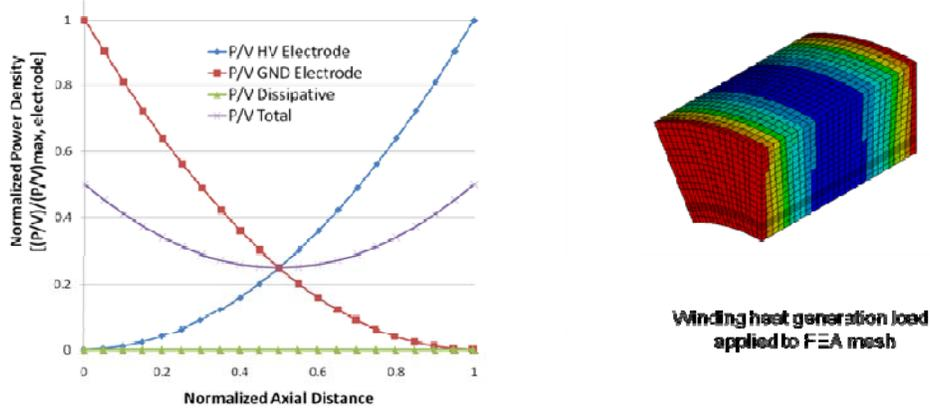
Fig. 39. Non-uniform heat generation in the capacitor windings
