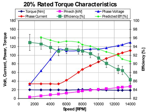
Fig. 13. Second roof-of-principle machine measured performance at 20% rated torque
