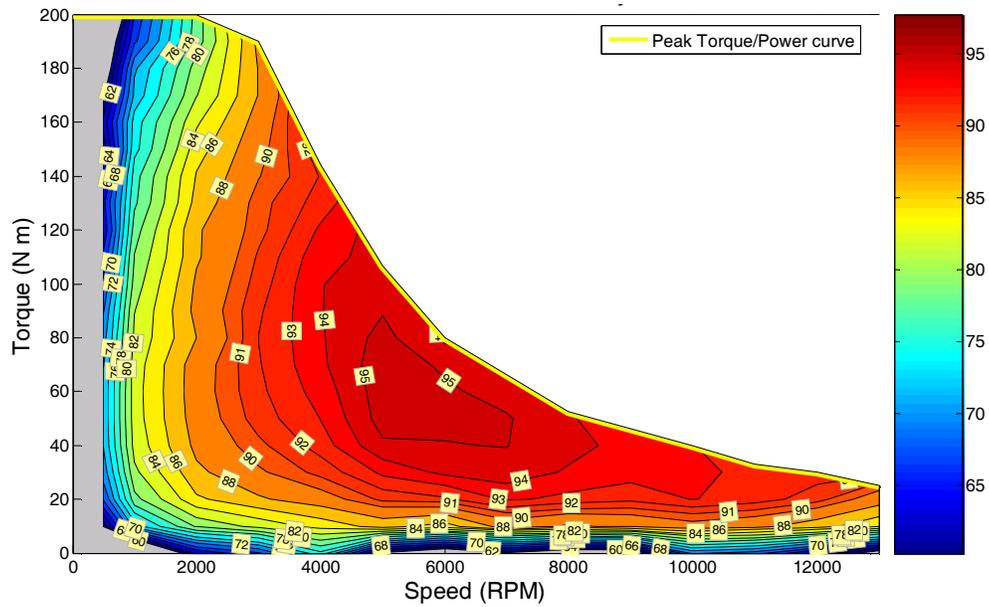
Fig. 12. 2010 Prius combined motor-inverter efficiency map for 650 Vdc.
