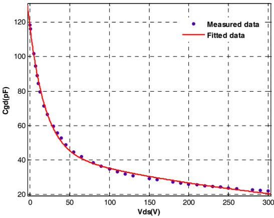
Fig. 25. Gate to drain capacitance (Cgd) vs Vds.
