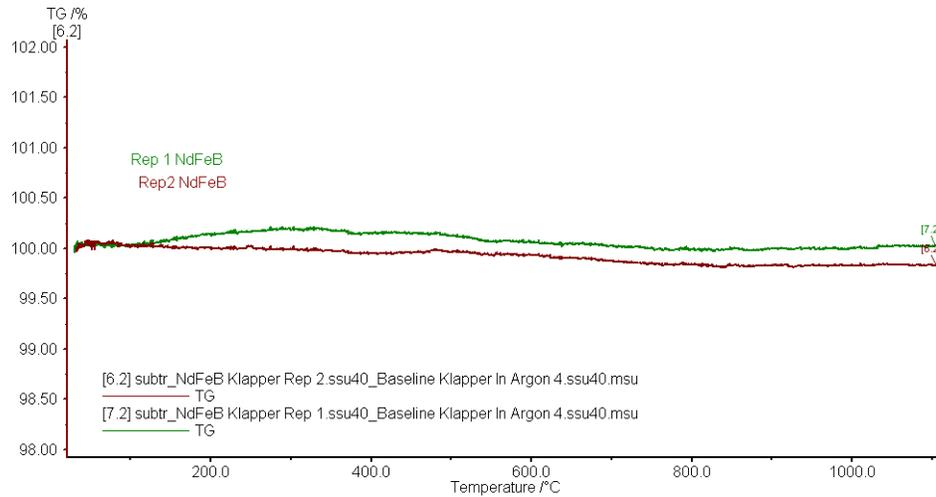
**Fig. 21. Thermogravimetric analysis (TGA) on  $\text{Nd}_{15}\text{Fe}_{77}\text{B}_8$  powder heated at  $10^\circ\text{C}/\text{min}$  under gettered Argon.**
