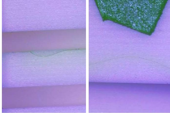
**Fig. 11. Cracks revealed by dye penetrant testing.**
