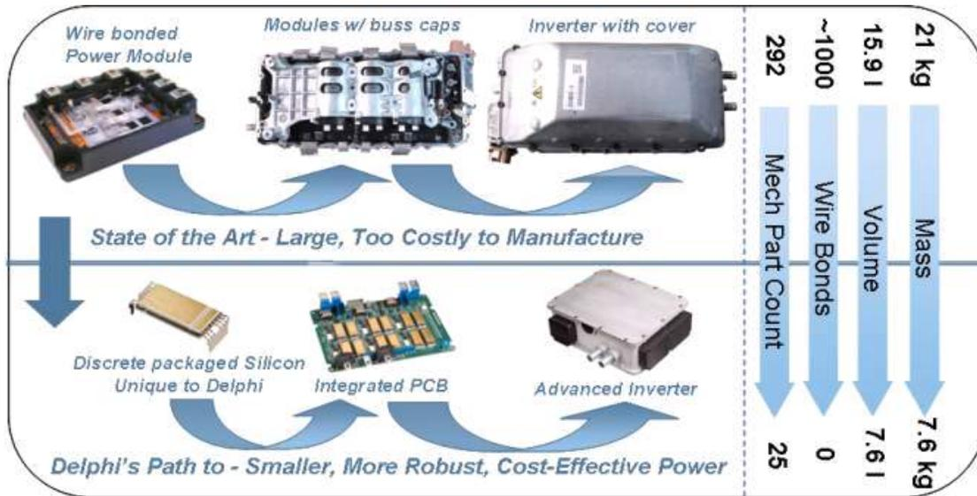
**Fig. 6. Delphi's Power Technology Path to Smaller, Lighter, Manufacturable and Lower Cost Power Electronics**
