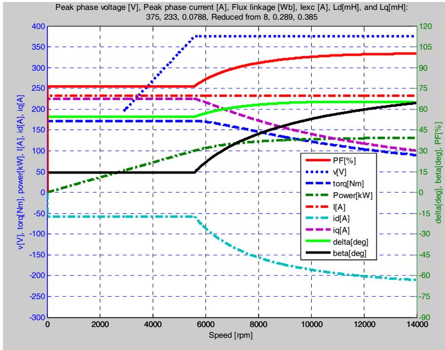
Fig. 7. Adjustable field can improve power factor.
