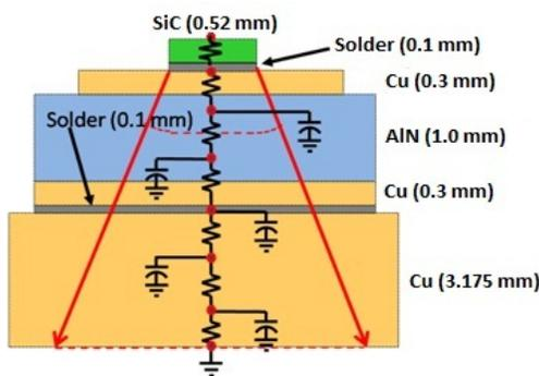
Fig. 7. Outline of electrothermal model for the SiC MOSFET in the Co-Pack Module
