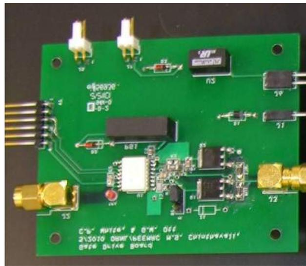
**Fig. 4. Gate Drive Board used for Testing**
