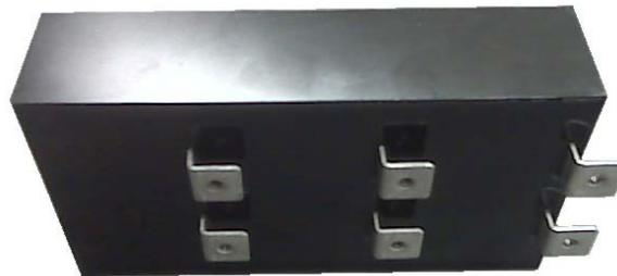
**Fig. 17. Completed capacitor from Electronic Concepts.**
