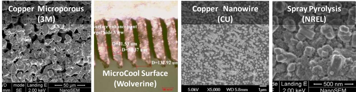
Fig. 17. SEM images of the enhanced surfaces tested
