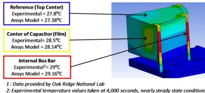
Fig. 40. Preliminary validation of DC-link capacitor thermal model
