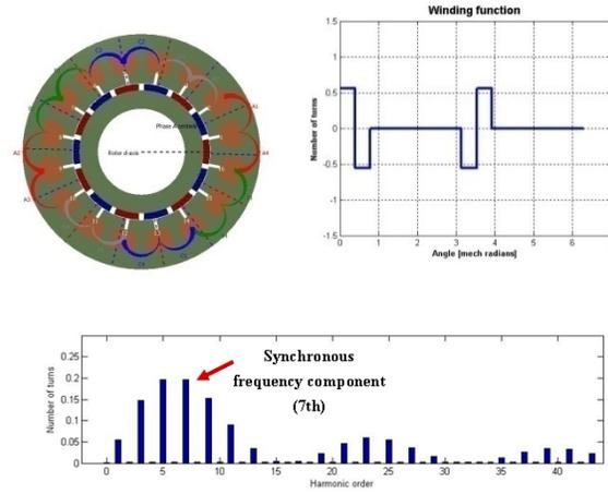
Fig. 2. Four phase (4P) machine: 16 slots/14 poles.
