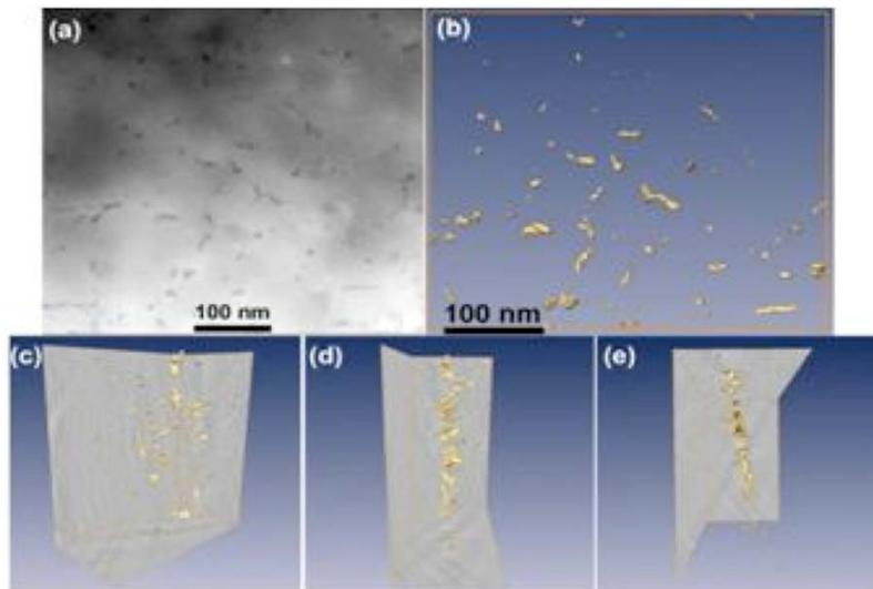
Fig. 6. (a) STEM HAADF image of the alloy (TiC particles in darker contrast) and corresponding ET 3-D reconstructed volume shown in (b) z-axis, (c) random, (d) x-axis, and (e) y-axis. The shape and morphology of the TiC particles are illustrated in yellow by using the iso-surface method.
