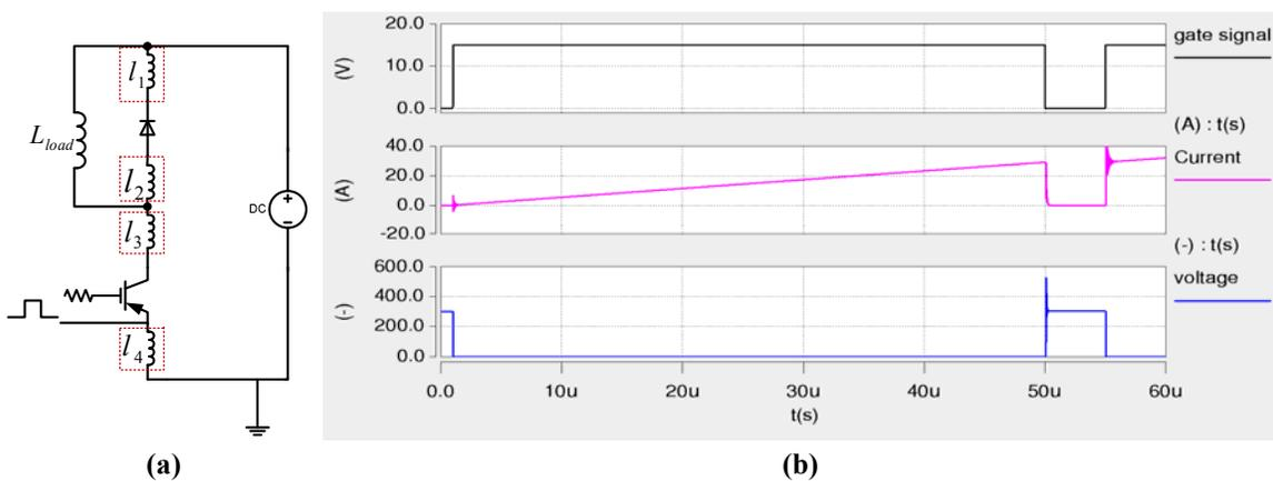
**Fig. 7. Double pulse tester: (a) circuit and (b) typical waveforms.**
