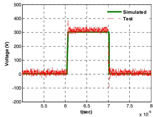
Fig. 30. Comparison of voltage waveforms of the JFET.
