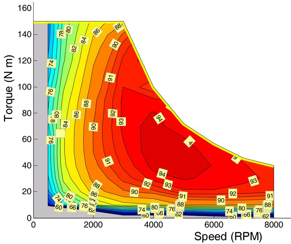
Fig. 13. 2010 Prius combined motor-inverter efficiency map for 500 Vdc.
