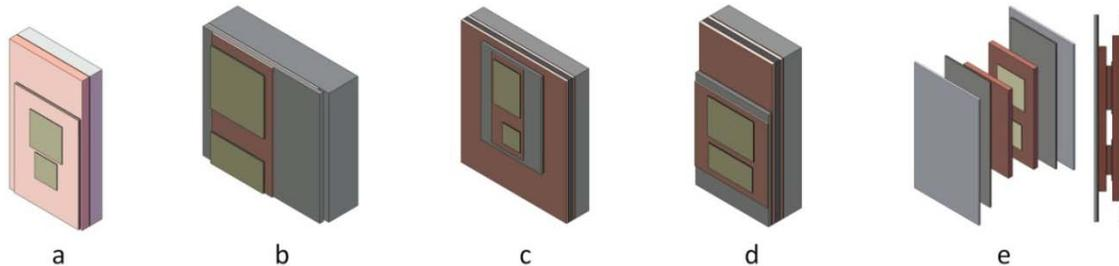
**Fig. 29. Alternative package configurations for package thermal performance comparison. Configuration geometries are based on existing commercial packages: (a) Semikron SKM, (b) Semikron SKAI, (c) 2004 Prius, (d) 2007 Camry, (e) 2008 Lexus LS 600H.**
