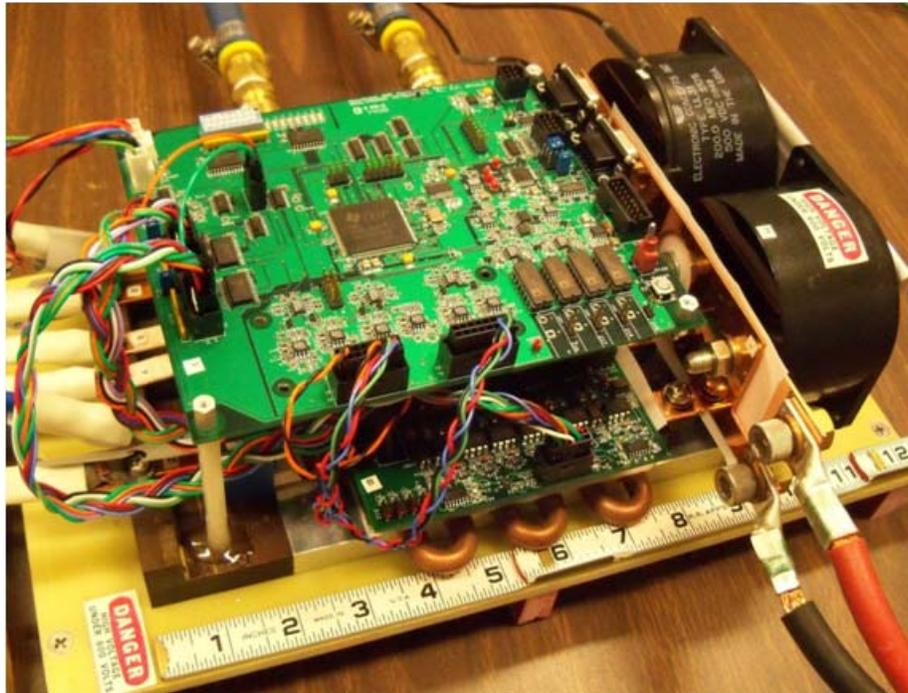
**Fig. 6. A 55 kW segmented inverter prototype.**
