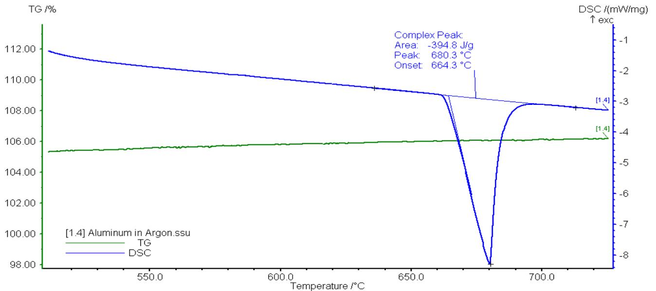
**Fig. 22. Differential scanning calorimetry (DSC) of  $\text{Nd}_{15}\text{Fe}_{77}\text{B}_8$  powder under gettered argon at  $10^\circ\text{C}/\text{min}$ . The onset of melting of the Nd-rich minority is observed at  $664.3^\circ\text{C}$ , close to the published values. Melting of this phase is required to achieve full densification during sintering.**
