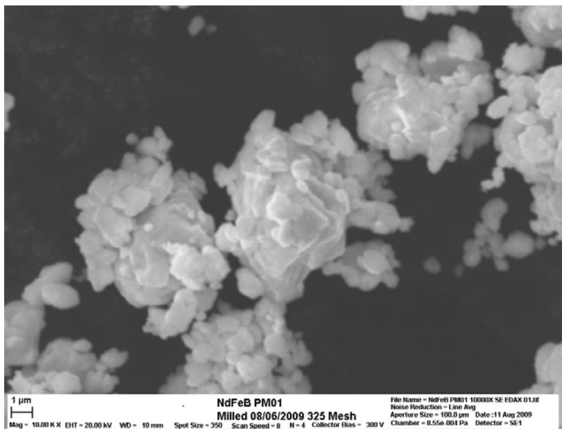
**Fig. 20. Scanning Electron Microscopy image of hydrided and planetary milled Nd<sub>15</sub>Fe<sub>77</sub>B<sub>8</sub> powder produced at GE Global Research. Average particle size is 3 to 5  $\mu\text{m}$ , with some finer particles agglomerated to larger particles.**
