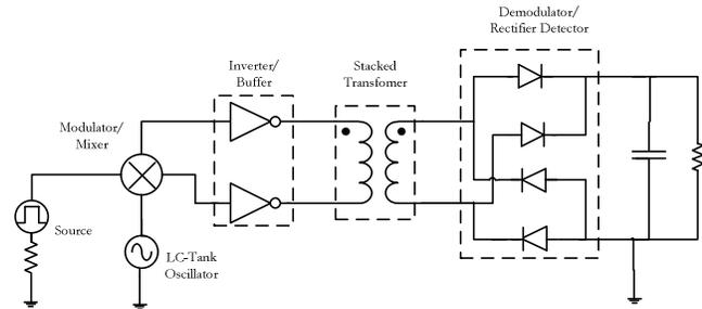
**Fig. 21. Block diagram of transformer based input isolation.**
