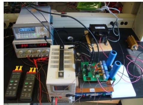
Fig. 15. Hardware testbed for high temperature switching experiments.
