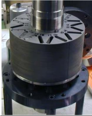
Fig. 10. Rotor of the second proof-of-principle machine
