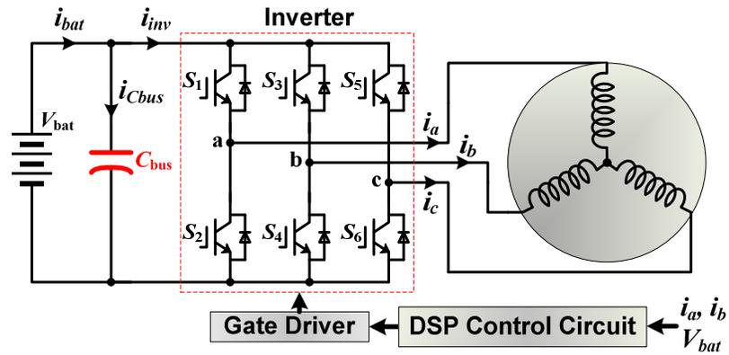
**Fig. 1. Standard VSI based drive system in HEVs.**
