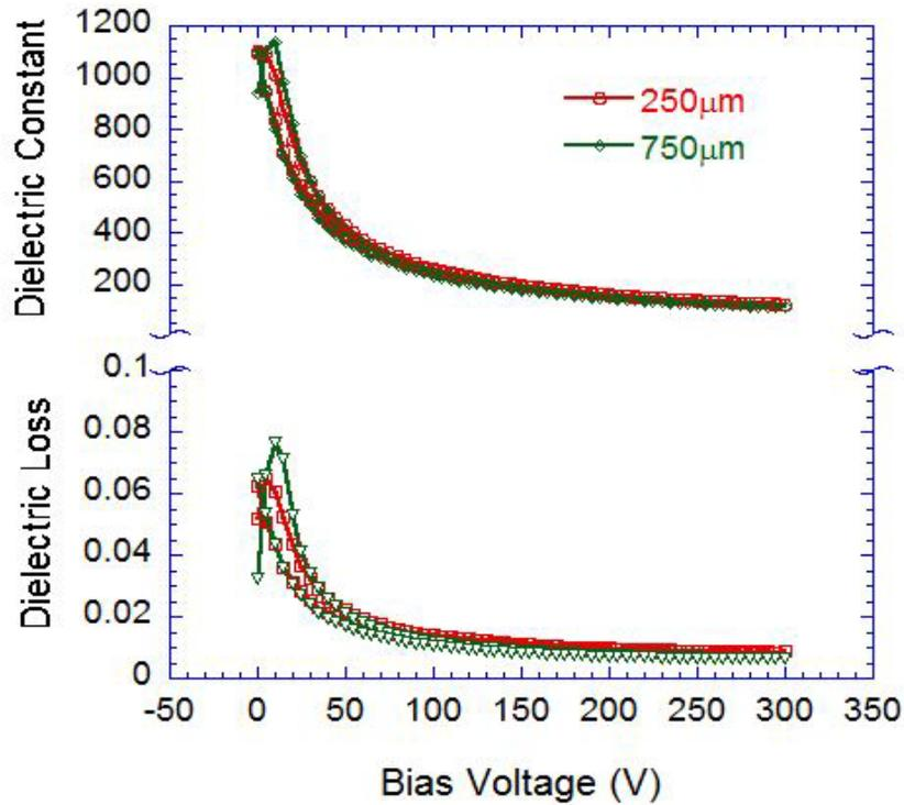
Fig. 4. Dielectric properties as a function of bias voltage measured on a  $\approx 3\text{-}\mu\text{m}$ -thick PLZT/LNO/Ni film-on-foil at room temperature.
