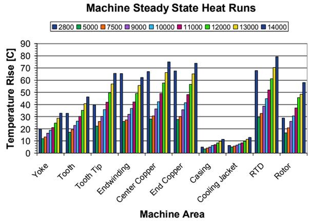
Fig. 15. Second proof-of-principle machine heat runs temperature rises in the various machine components at various speeds.
