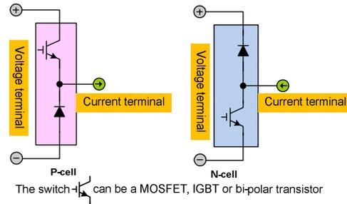
Fig. 2. Two basic switching cells: P-cell and N-cell.
