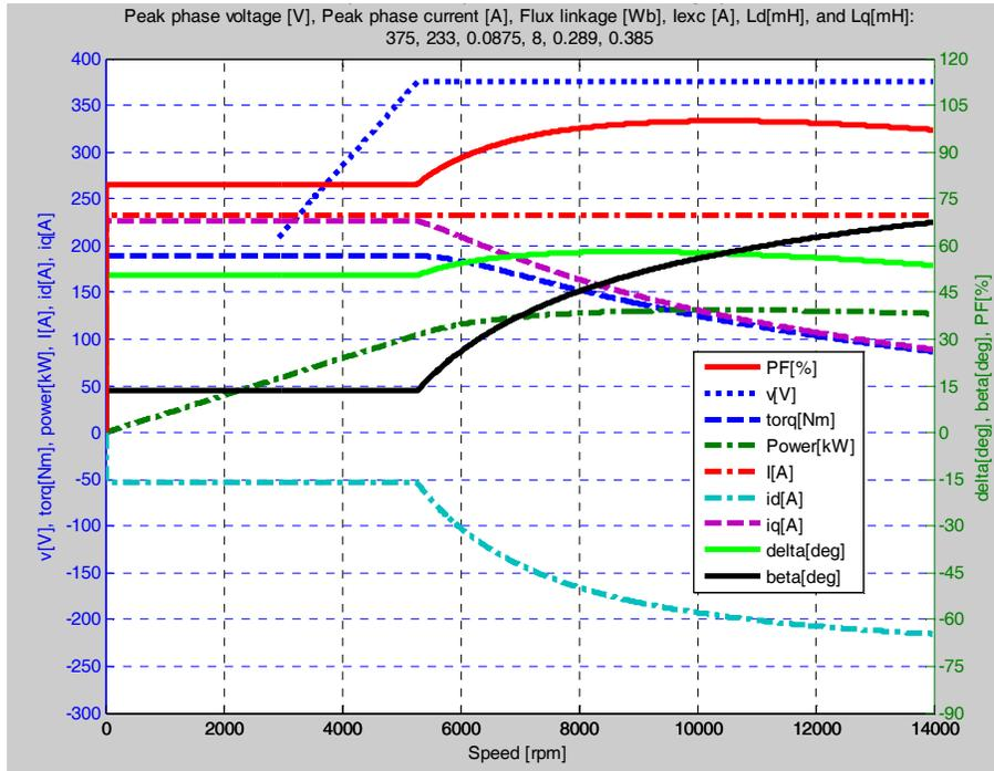
Fig. 6. Simplified motor performance versus speed curves.
