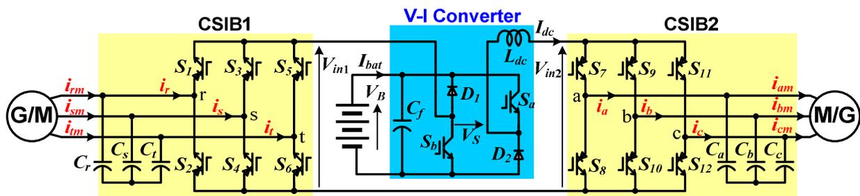
Fig. 2. V-I converter based CSI for a dual-motor drive system for series or power-split series parallel HEV applications.
