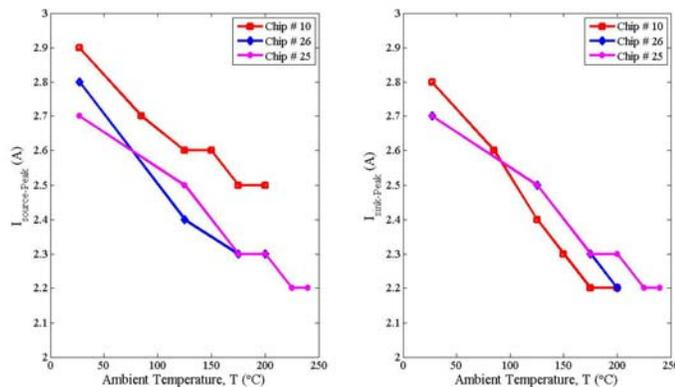
**Fig. 3. Measured source and sink current peaks at different ambient temperatures for three different ICs with same R-C load ( $R_G = 3.4 \Omega$  and  $C = 10 \text{ nF}$ ).**
