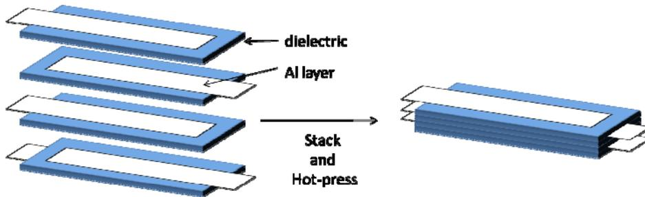
**Fig. 9. Scheme for fabrication of larger value capacitors**
