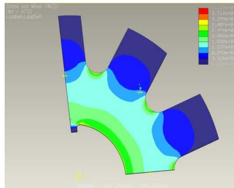
**Fig. 8. Stress analysis of rotor lamination stack.**
