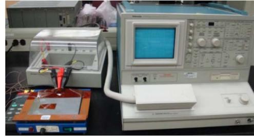
Fig. 10. Static characterization setup with curve tracer.
