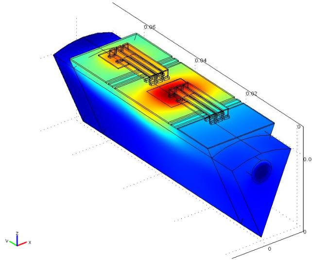
Fig. 5. FEA results of the simulated octagonal model.
