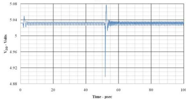
Fig. 15. Corinth voltage regulator transient event simulation.
