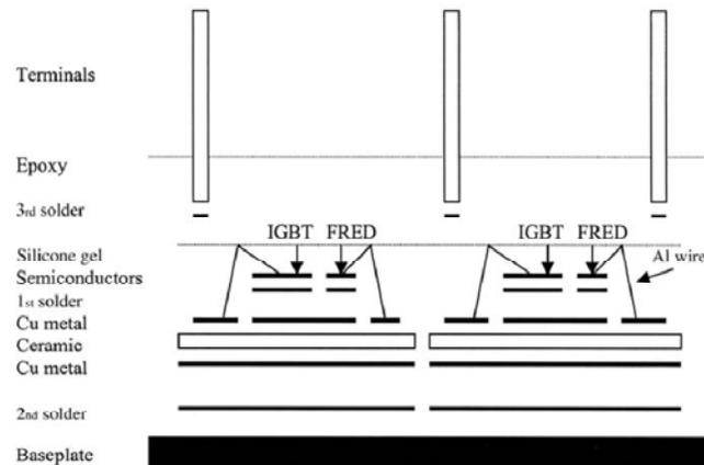
**Fig. 1. Structure of an IGBT module.** {Source: [1].}
