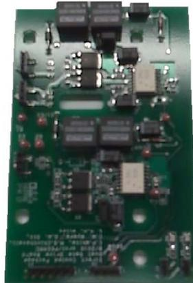
**Fig. 16. Completed gate drive board.**
