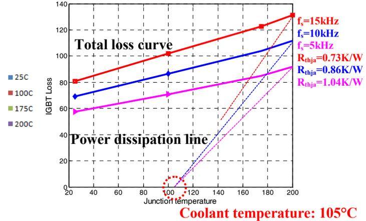
Fig. 18. IGBT power losses and thermal analysis at different frequencies.
