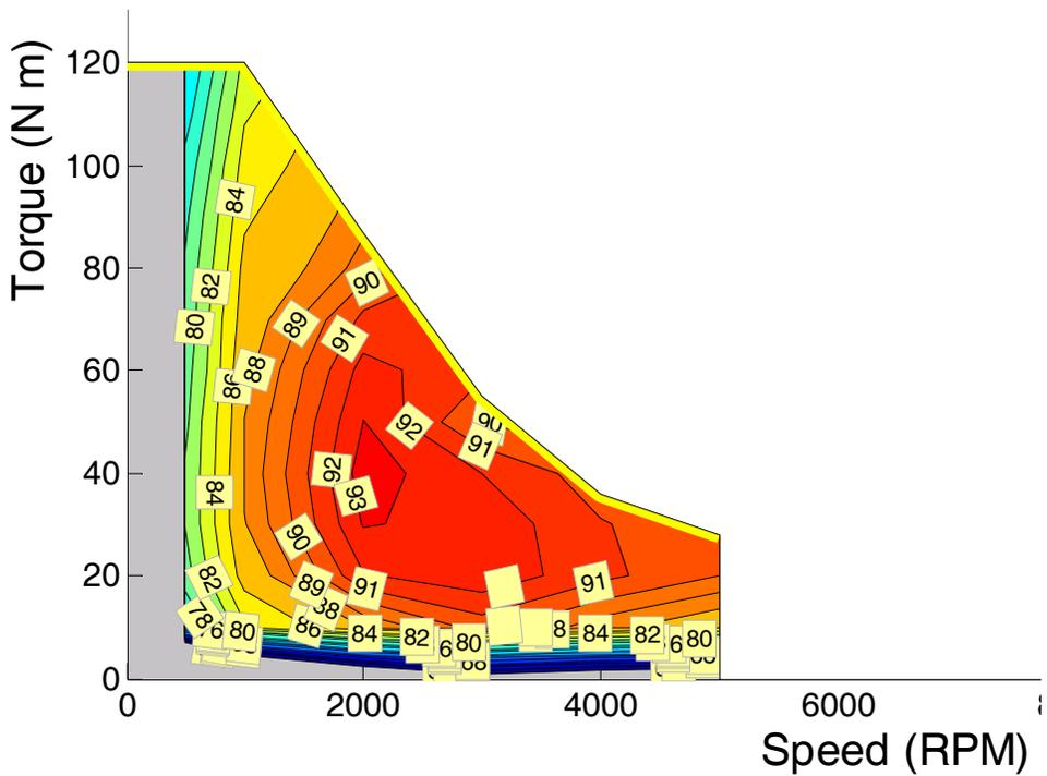
Fig. 14. 2010 Prius combined motor-inverter efficiency map for 225 Vdc.
