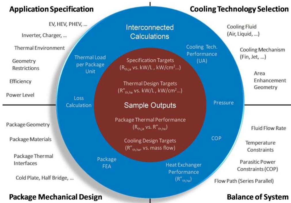
Fig. 5. Power electronics system analysis parameter overview
