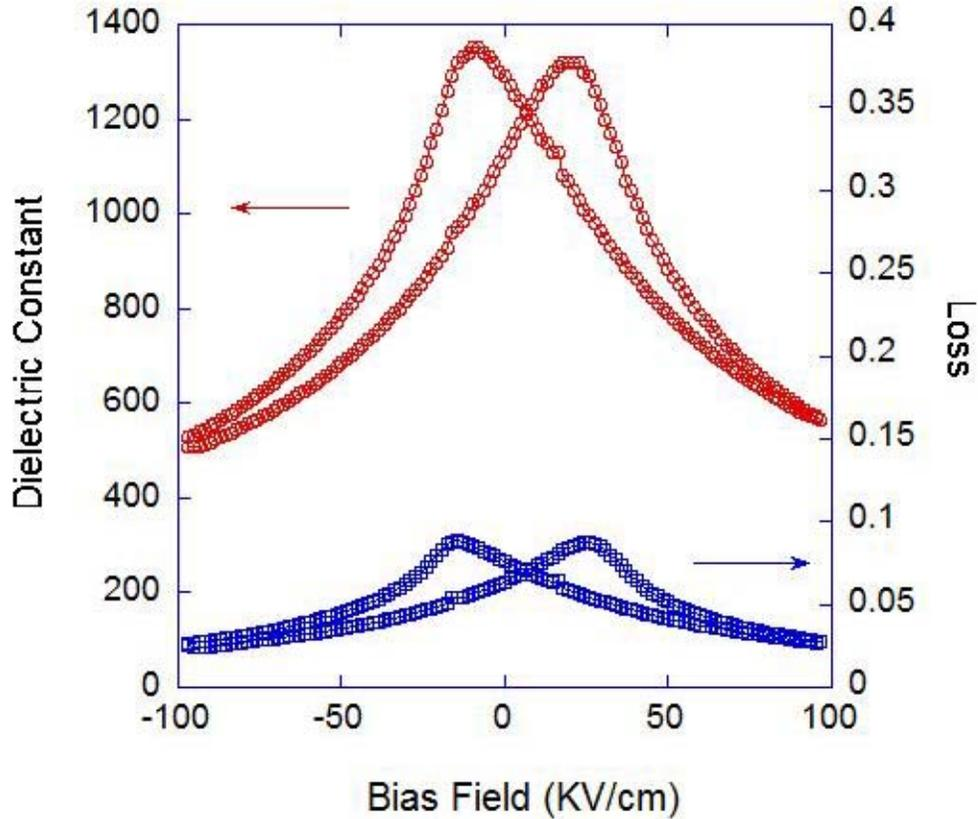
**Fig. 6. Dielectric properties of a 20-mm-diameter,  $\approx 3\text{-}\mu\text{m}$ -thick PLZT/LNO/Ni film-on-foil measured at room as a function of bias field.**
