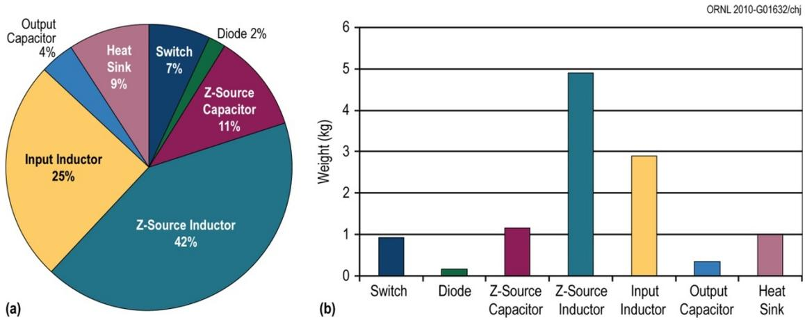
**Fig. 13. Weight breakdown by component for the 55 kW CF-trans-qZSI design:**
