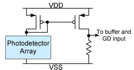
Fig. 20. Photodetector configuration.
