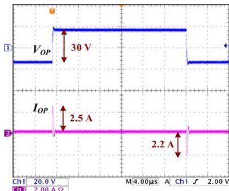
**Fig. 2. R-C load test results at 200°C with  $R_G = 3.4 \Omega$  and  $C_{Load} = 10 \text{ nF}$ .**
