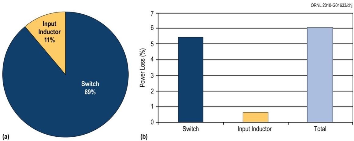
**Fig. 14. Boost mode loss breakdown by component for the 55 kW CF-trans-qZSI design:**
