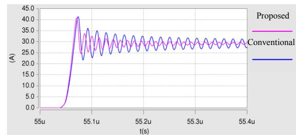
**Fig. 9. IGBT current waveform at turn on.**
