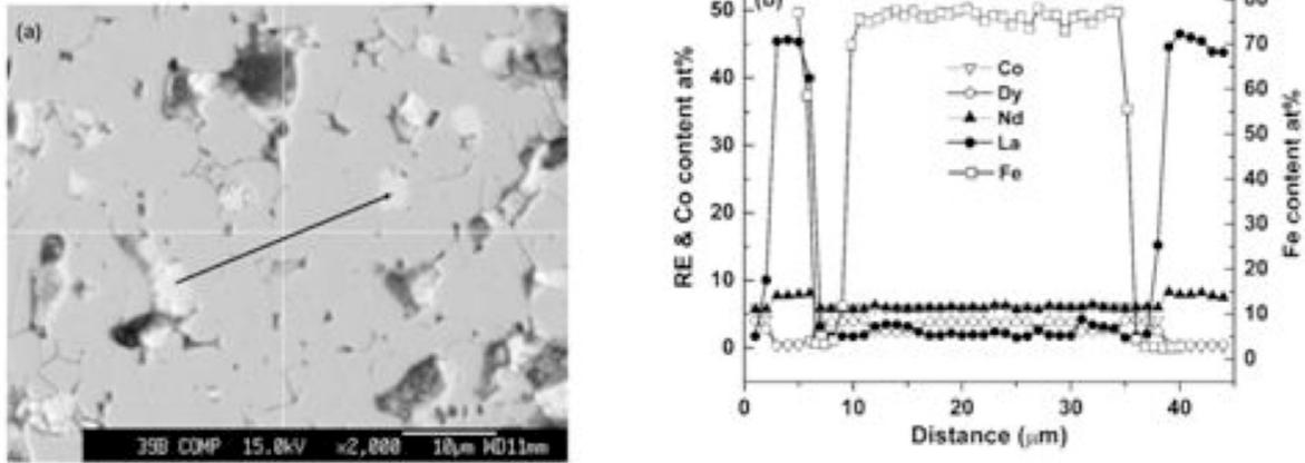
Fig. 2. Microstructure and electron microprobe composition profiles with La substituted for Y.
