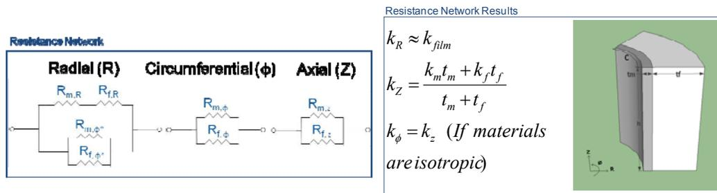
Fig. 38. Resistance network and resulting equations
