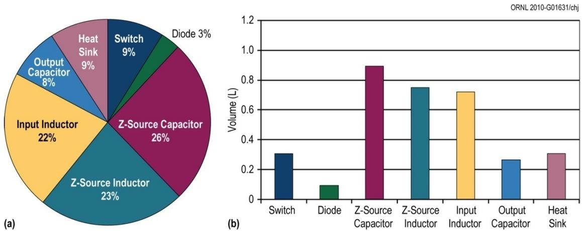
**Fig. 12. Volume breakdown by component for the 55 kW CF-trans-qZSI design:**
