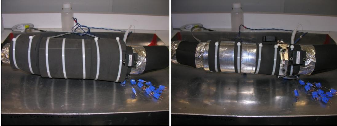
Fig. 2. Final stages of module insulation.
