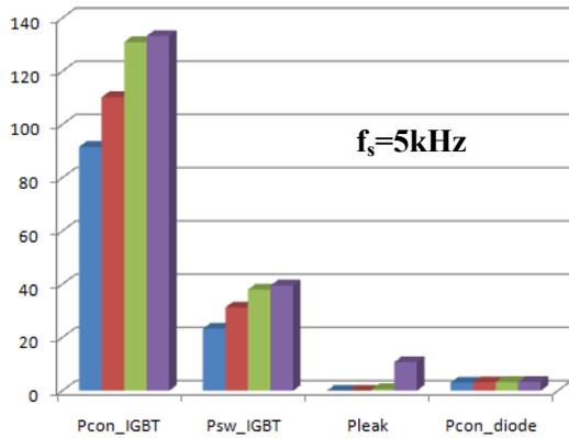
Fig. 17. Power losses in one phase leg at different temperatures (f<sub>s</sub>=5kHz).
