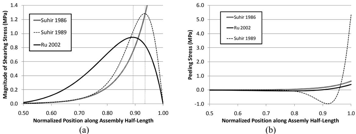
**Fig. 3. Thermally induced stresses predicted in a bi-material assembly for (a) shear stress using the Ru (2002), Suhir (1986), and Suhir (1989) models and (b) peeling stress using the Ru (2002) model.**
