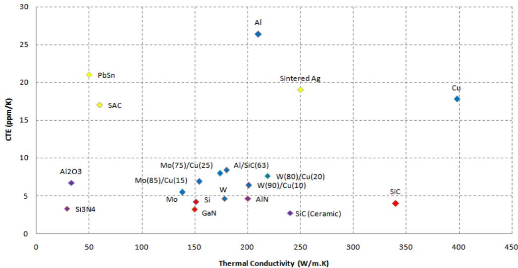
Fig. 7. Thermal properties of power module packaging materials.
