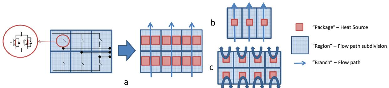
**Fig. 16. a. Coolant system flow path abstraction and definition; b. Cold plate; c. DC-DC converter**
