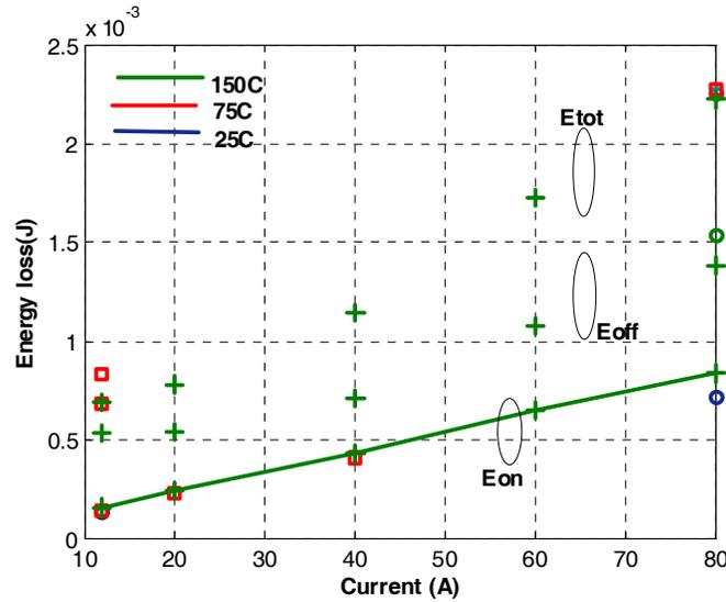
Fig. 7. Switching losses of 1,200 V, 100 A, SiC JFET.
