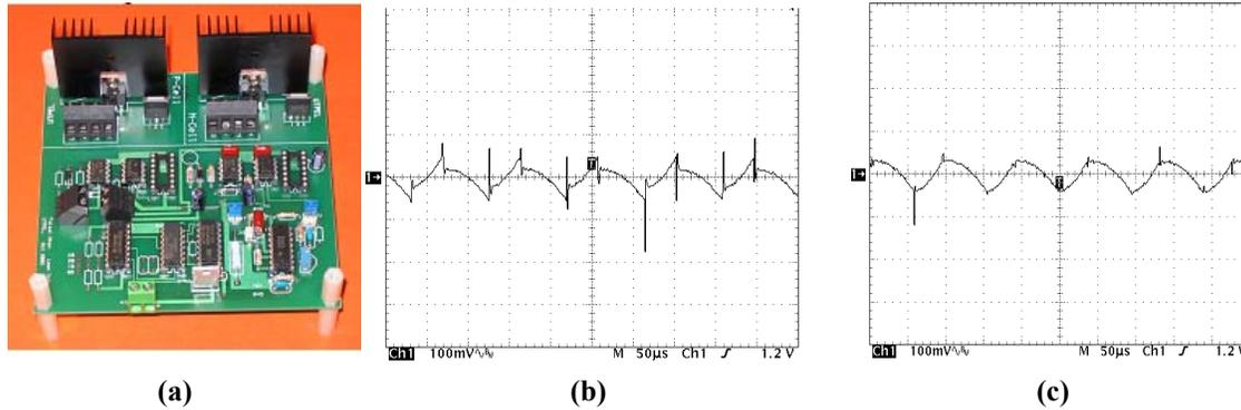
**Fig. 4. Experimental setup for P-cell and N-cell buck converters: (a) experimental prototype of the P-cell and N-cell, (b) output voltage ripple (100 mV/div) of P-cell buck converter, and (c) output voltage ripple (100 mV/div) of N-cell buck converter.**
