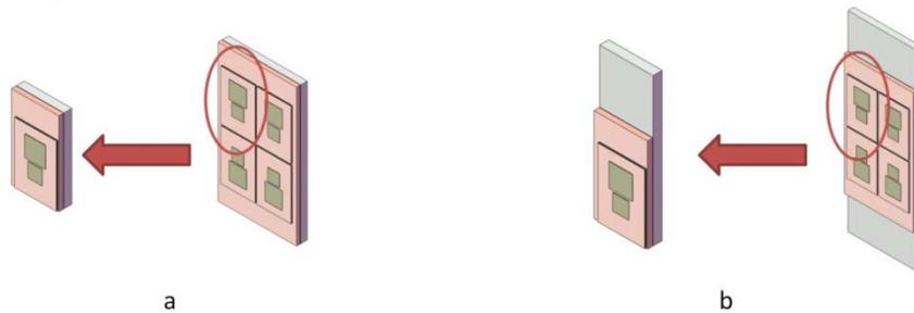
Fig. 47. Package geometry configurations. (a) Small heat sink area (15.34 cm<sup>2</sup>); (b) Large or extended heat sink area (24.19 cm<sup>2</sup>).
