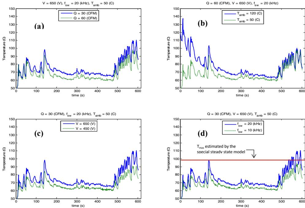
Fig. 5. Transient results showing the effect of changing Q, T<sub>amb</sub>, V, and f<sub>sw</sub>.
