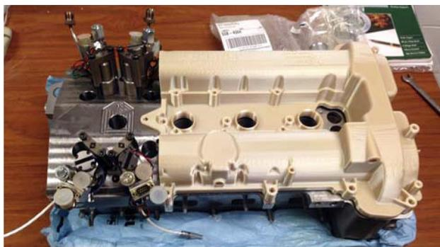
**FIGURE 6.** Cylinder head and custom valve cover for flexible ORNL multi-cylinder engine experiment that will be completed during FY 2014.
