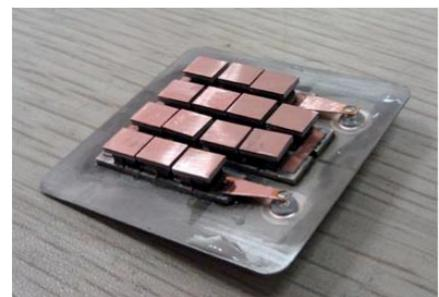
High-temperature thermoelectric module with the hot-side casing removed. (Cleary, GMZ Energy)
