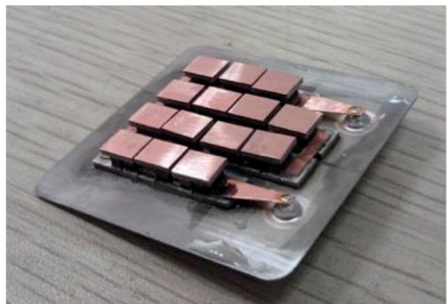
**FIGURE 3.** High-temperature thermoelectric module with the hot-side casing removed.
