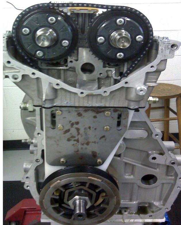
**FIGURE 7.** VCR Engine Timing Chain System
