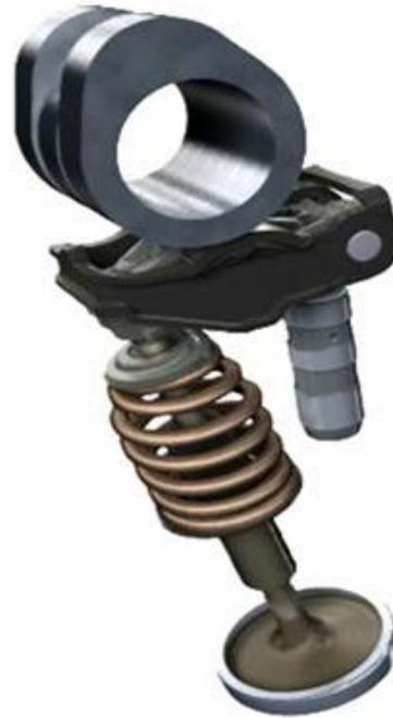
FIGURE 2. Eaton VVA Mechanism
