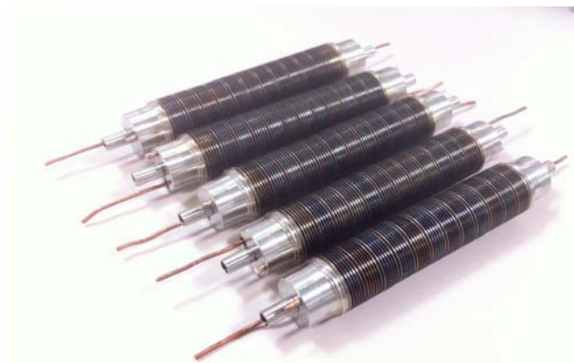
Figure 1 Thermoelectric power generation cartridge Hot and cold side heat exchangers are the finned tube type and are bridged by thermoelectric elements
