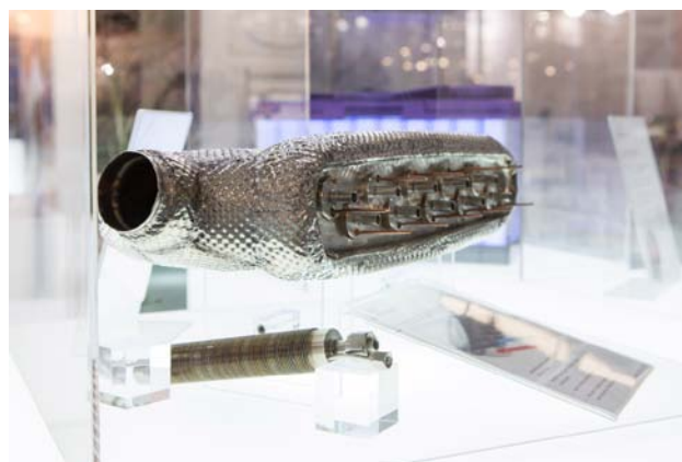
Figure 2 LDV TEG developed by Tenneco and Gentherm shown at the International Motor Show in Frankfurt 2015. Device consists of 10 thermoelectric cartridges electrically and thermally connected in series
