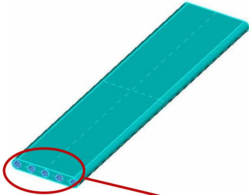
All channels in a tube are in parallel, assume equal flow per channel, so only need to simulate 1 channel per tube, then multiply by number of channels.
