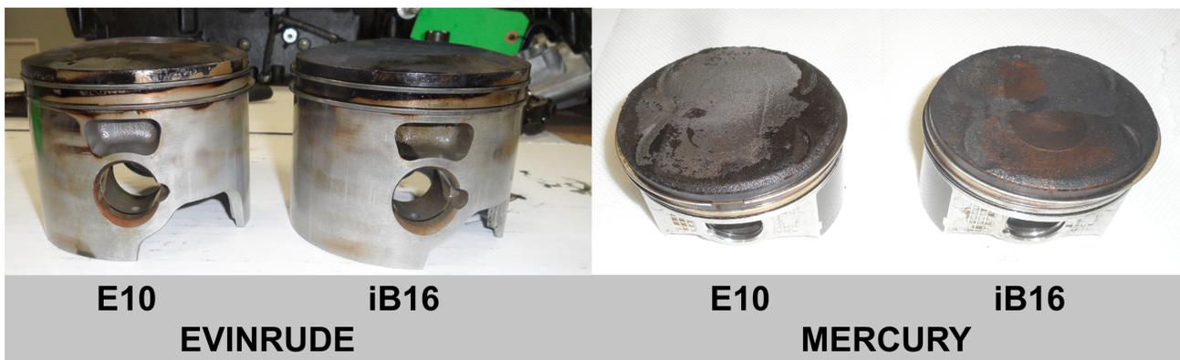
**FIGURE 3.** Comparison of Pistons (cylinder number 1) for the Evinrude and Mercury Engines Operated on E10 and iB16
