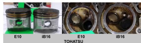
Comparison of Pistons and Cylinder Heads (cylinder number 1) for the Tohatsu Engines Operated on E10 and iB16 (Wallner, report IV.3)
