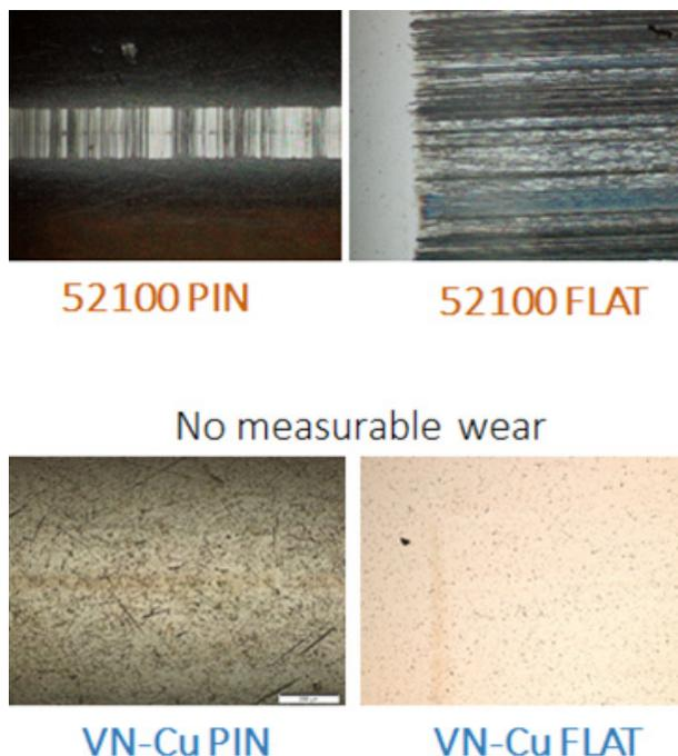
**FIGURE 2.** Wear performance of uncoated (top) and non-ferrous VN-Cu coated pin and flat samples (bottom). Uncoated steel samples show severe wear losses, while the coated samples shown no discernible wear.
