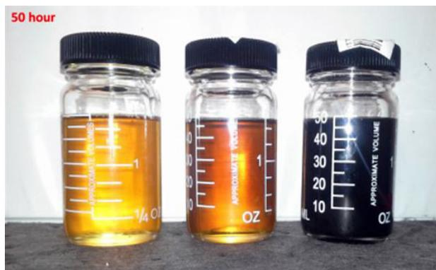
FIGURE 3. Lubrication oil; from left to right: fresh, head, power cylinder.
