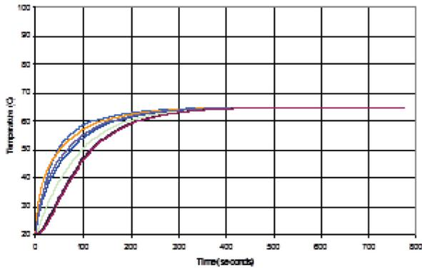
Figure 2. Start-up TC readings at various depths within the ring when preheating with water at 65°C.
