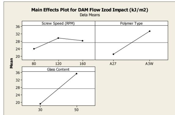
Figure 16: Data show that direct compounding formulations exhibit Izod Impact properties comparable to the pre-compounded pelletized formulations.
