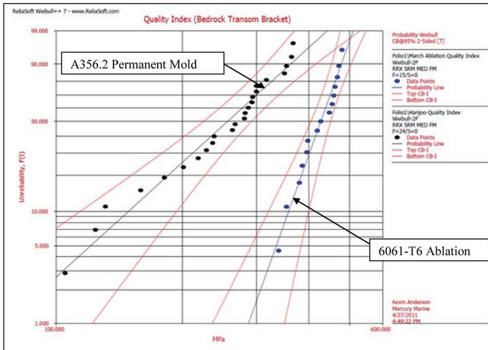
Figure 10. Comparison of 6061-T6 Ablation versus A356.2 Permanent Mold – Quality Index. (This Information was provided courtesy of Mercury Marine. Mercury Marine makes no warranty, express or implied, or assumes any legal liability or responsibility for the accuracy, completeness, or usefulness of this information.)
