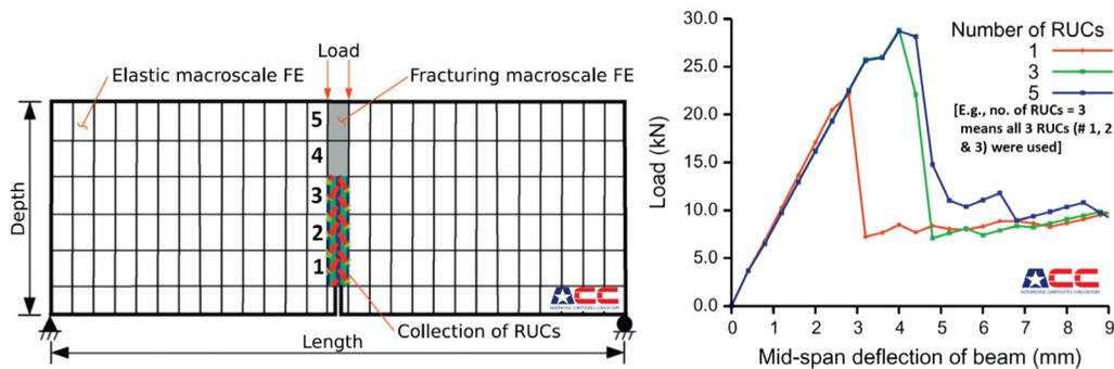
Figure 7. FEM results of 3-point bent specimen. The three curves demonstrate the converging dependence of load-deflection relationship (peak and plateau) on the number of RUCs used.
