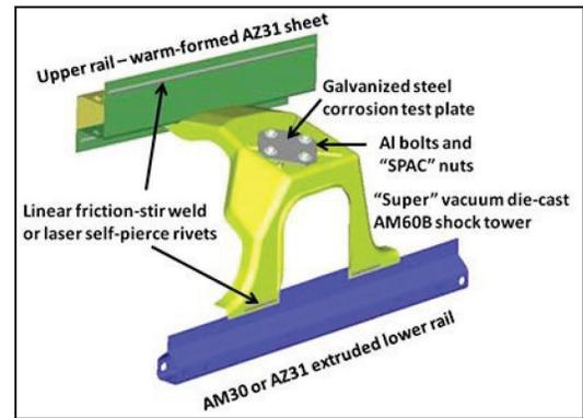
Figure 1. Final version of Mg front-end “demonstration” structure.
