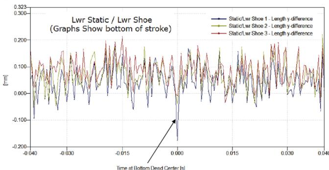
Figure 23. Measured dynamic motions of three points on the lower die shoe
