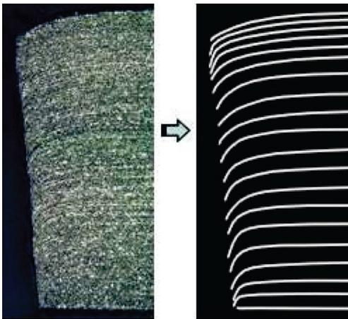
Figure 5. Strain Distribution of Shear-Effected Zone Obtained from the Optical Image
