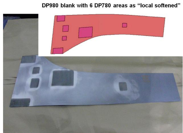
Figure 15. B-Pillar DP980 Blank with Local Softened Patches
