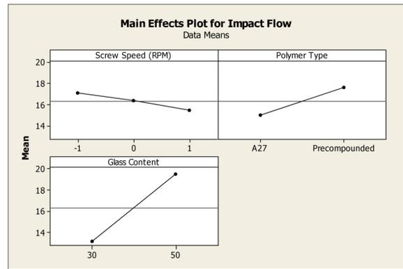
Figure 14: Attributes like screw speed, polymer type and glass content had a significant effect on Impact Flow.
