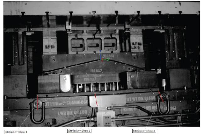
Figure 22. Targets on Die Surfaces
