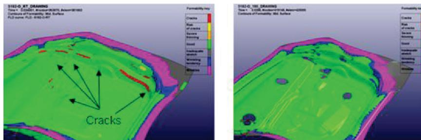
Figure 4. Simulation results for the initial die geometry at 20° C (left) and the final die geometry at 180° C (right).
