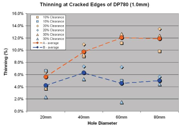
Figure 2. Thinning Limits vs. Hole Diameter DP780 Samples
