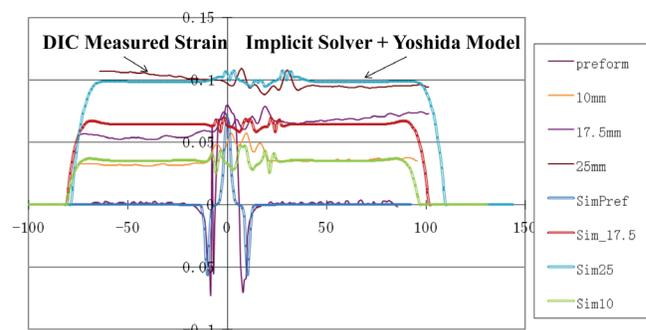
Figure 20. FEA Simulation Results vs. DIC Measurements – Surface Tensile Strain
