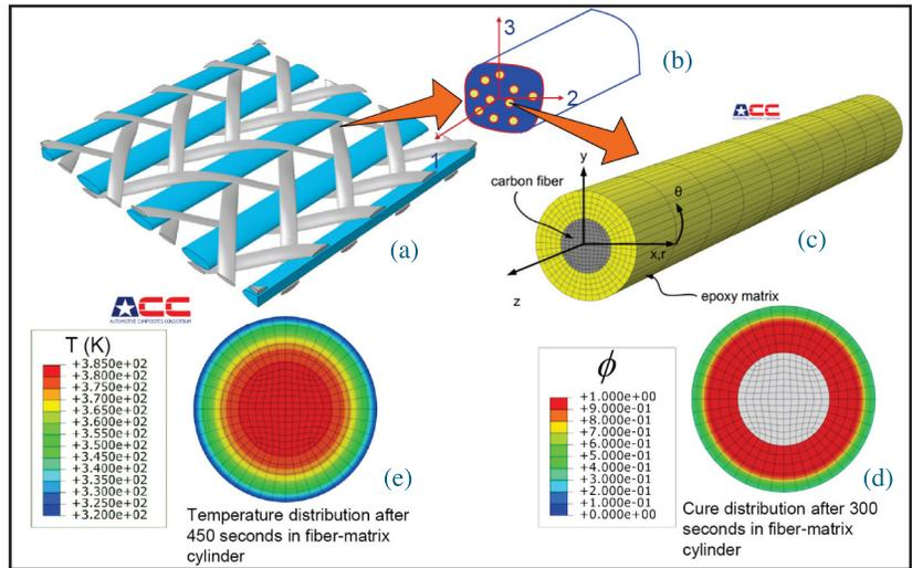
Figure 8. (a) Braided carbon-fiber composite (resin/matrix not shown for clarity). (b) A representative tow is selected. (c) A representative fiber is selected and modeled as surrounded with resin-rich cylinder. (d) Degree of cure ( $\phi$ ) variation in the matrix (the fiber is fully cured and represented as central blue circle with solid color). (e) Temperature ( $T$ ) distribution in the fiber-resin system after a specific curing time.
