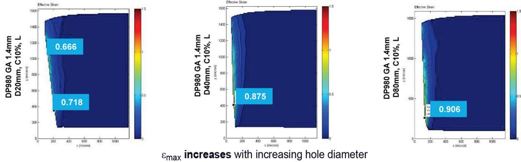
Figure 8. The effect of hole diameter on shear strain distribution of DP980 Samples
