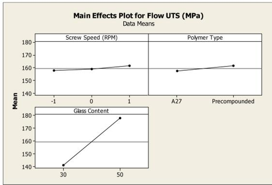
Figure 13: Attributes like screw speed and polymer type had minor effect on Ultimate Tensile Strength (UTS), while glass content had significant effects on UTS (measured in MPa).
