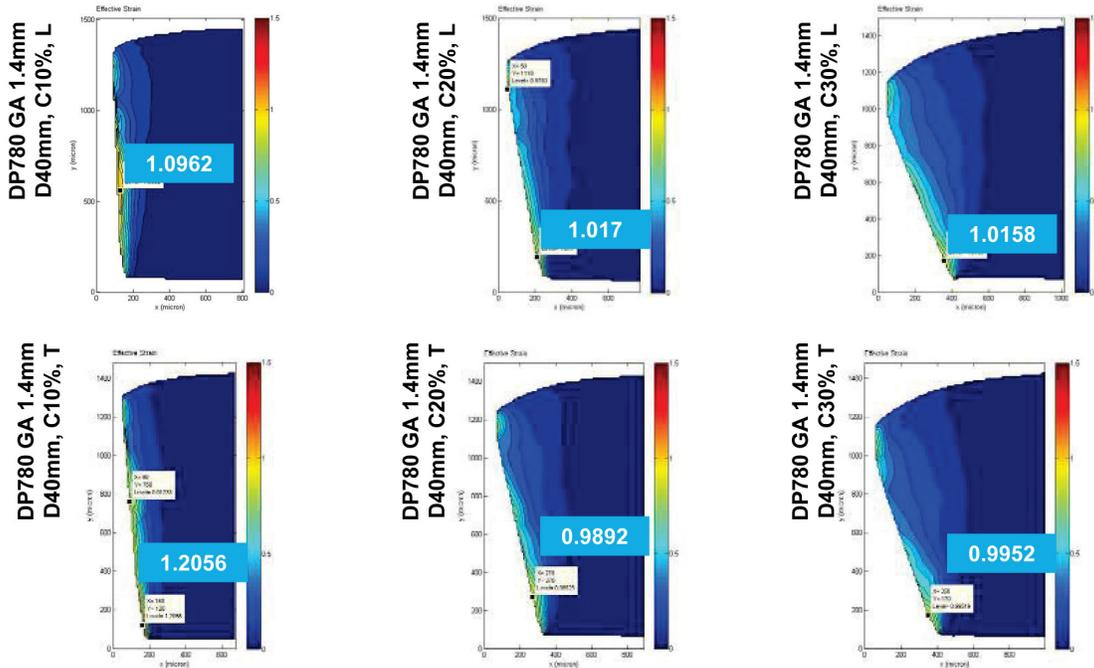
Figure 9. The effects of Cutting Clearance and Orientation on Shear Strain Distribution.
