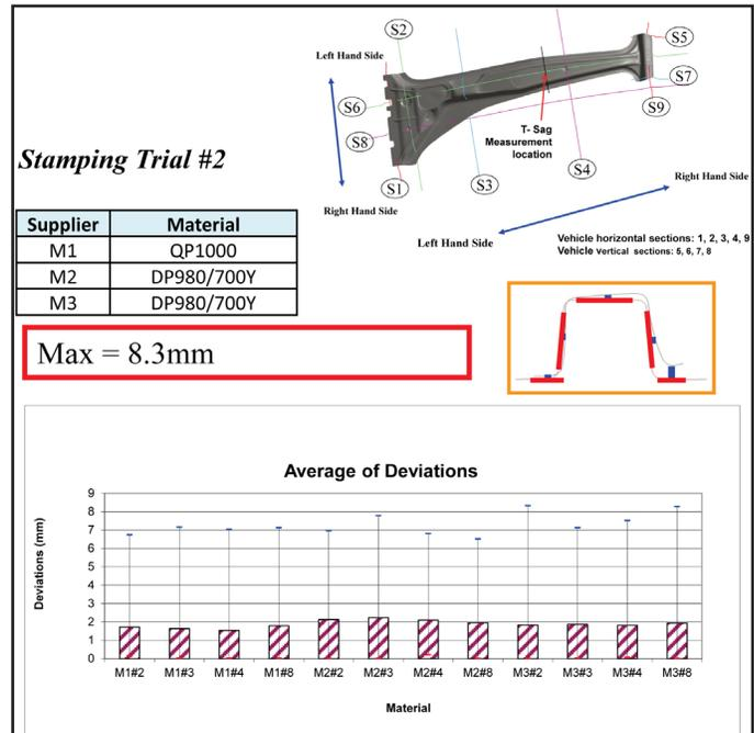
Figure 11. Springback Measurement Results – Average of Deviations
