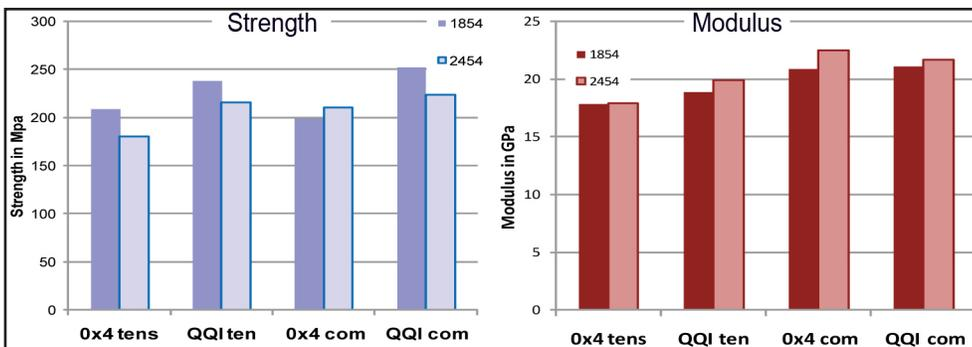
Figure 1. Effect of fabric weight on strength and modulus for tensile and compressive loading, for two different layups for both fabrics.
