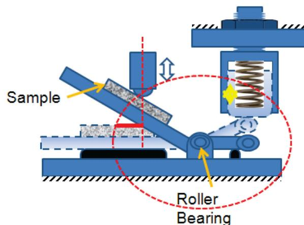
Figure 27. Coating Impact-Sliding Fatigue Test Phase II Apparatus.
