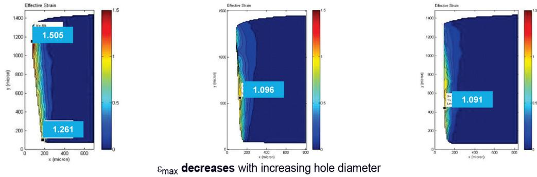
Figure 7. The effect of hole diameter on shear strain distribution of DP780 Samples
