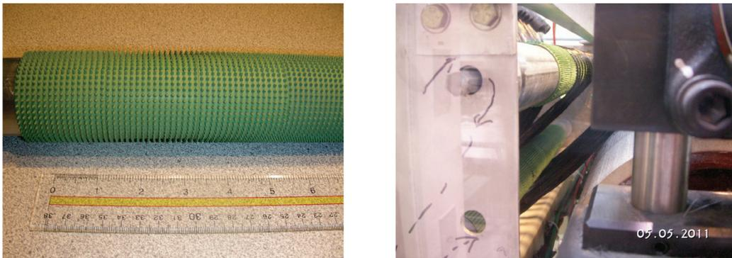
Figure 12: Nubby roller used to open gaps in large carbon fiber bundles before chopping (left). Carbon fiber bundles traveling over two nubby rollers (right).
