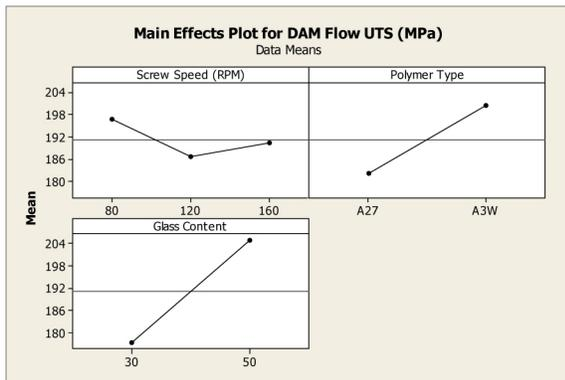
Figure 15: Data show that direct compounding formulations can exhibit tensile strength properties comparable to the pre-compounded pelletized formulations. UTS measured in MPa.
