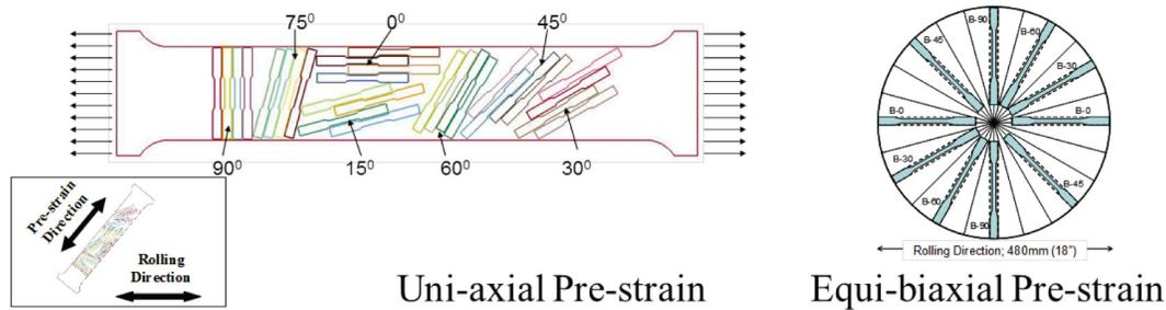
Figure 25. Cut patterns used to obtain desired orientations of tensile specimens in 15 degree increments after prestrain of the metal in uniaxial tension or equal-biaxial tension. These specimens provided information on the nature of transient hardening behavior under discontinuous strain paths.
