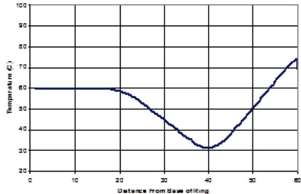
Figure 3. Steady-state TC readings when cooling with water at 15°C.
