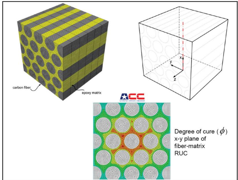
Figure 10. A more detailed larger FE model with multiple fibers embedded in a matrix and the spatial distribution of  $\phi$  within the system at some point in time during the curing process.
