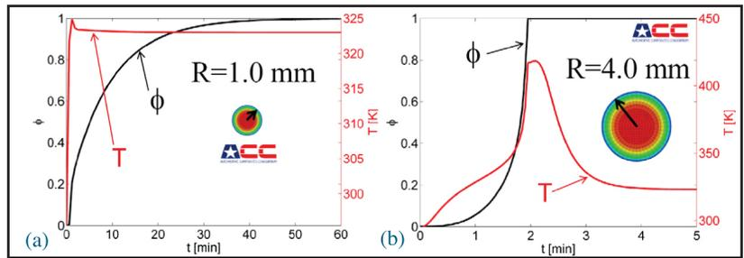
Figure 9. Computational results for  $T$  and  $\phi$  variation with time ( $t$ ) for different size 1-fiber concentric-cylinder FE models.
