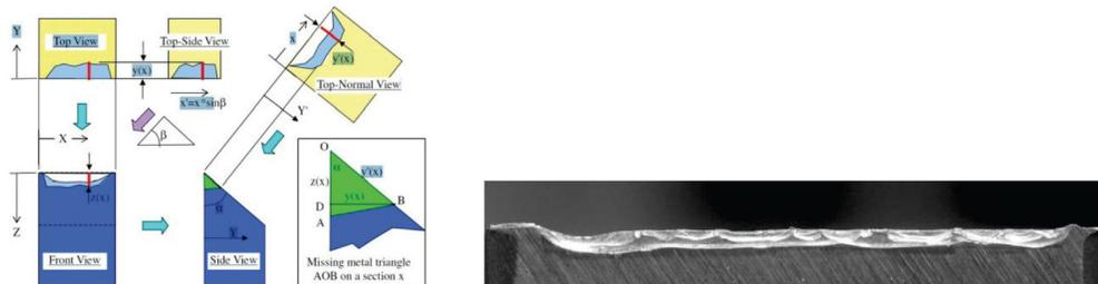
Figure 28. Edge Chipping Study (left) as applied to a chipped tool insert (right)
