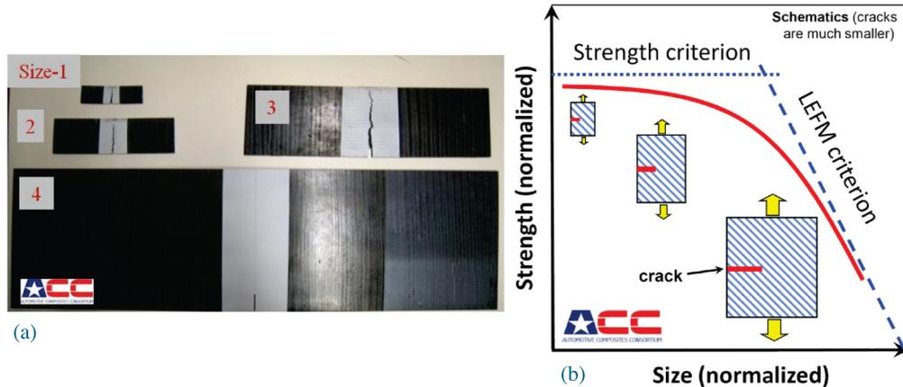
Figure 6. (a) The four different structural (plaques) sizes that were selected in order to study size effects on braided carbon composites’ nominal strength. (b) Schematic showing the classical relationship between nominal strength vs. relative size (normalized measures).
