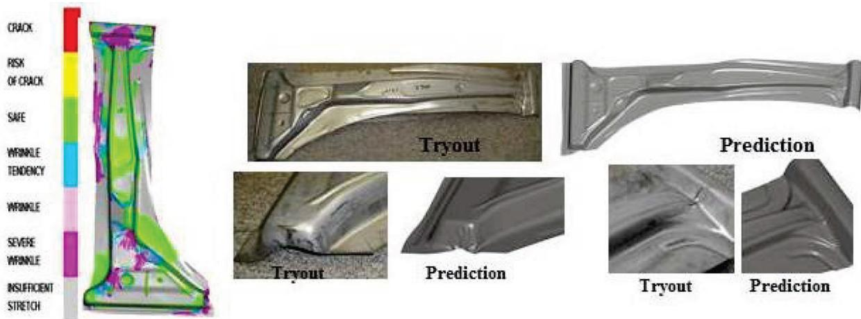
Figure 10. Formability Compression. No split was predicted but several wrinkles were predicted. The prediction agreed with the tryout panel.
