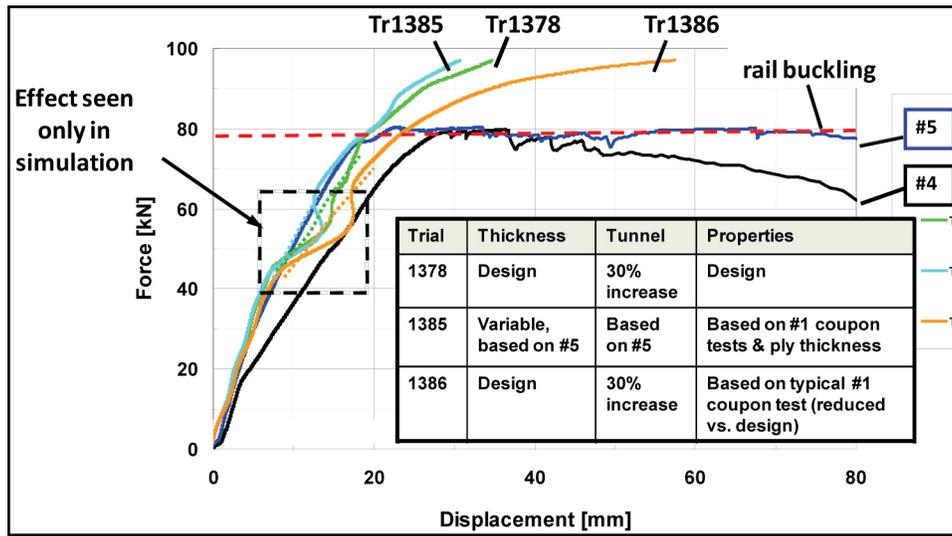
Figure 4. The force-displacement curves for two underbodies assembled into steel frames, compared to the predictions. The predictions are as modified for actually molded parts, which were heavier than the design.
