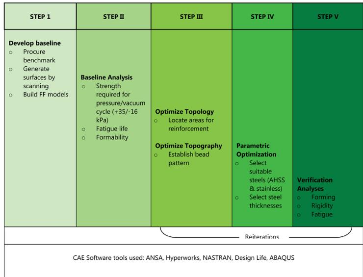
Figure 33. Stepwise procedure used to develop low mass alternatives to the benchmark fuel tanks
