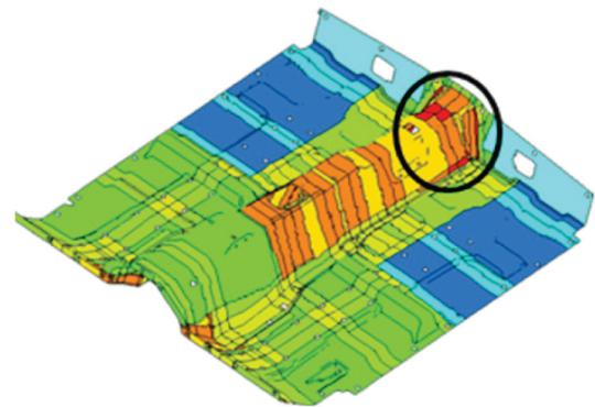
Figure 3. Overlaps in the designed preform layup. More intense shades indicate more overlaps, up to 4 in the circled area.
