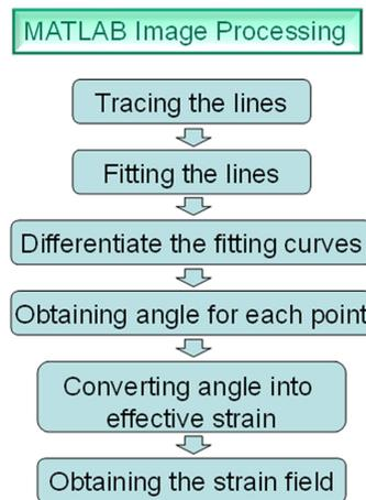
Figure 6. Flow-Chart of Matlab Strain Calculation Program and Mathematic Equations
