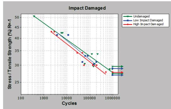
Figure 2. S-N curve showing fatigue life of undamaged fabric SMC specimens, in comparison to two levels of impact damage.
