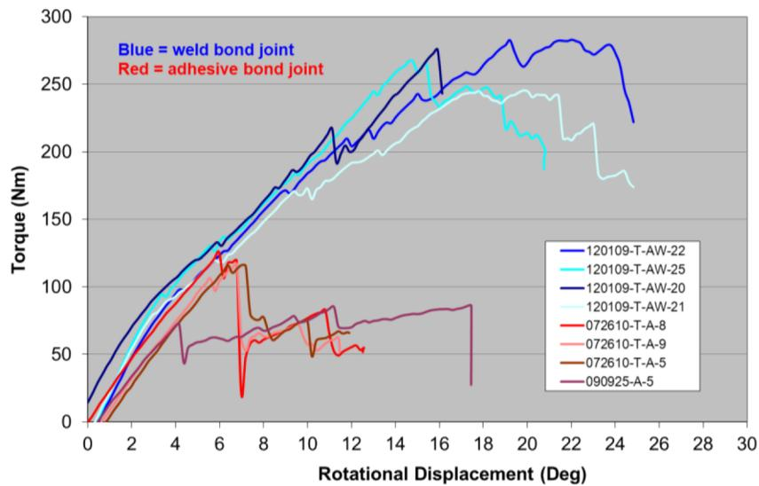
Figure 9. Quasi-static torsion test results for weld bonded and adhesively bonded joint specimens.
