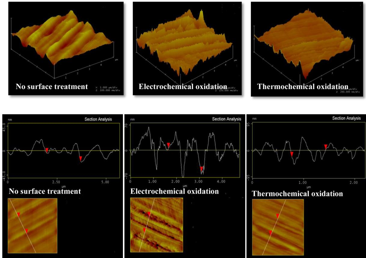
Figure 23. AFM imaging of the surface of the fibers showing roughness of the surface of the fibers perpendicular to the fiber axis.
