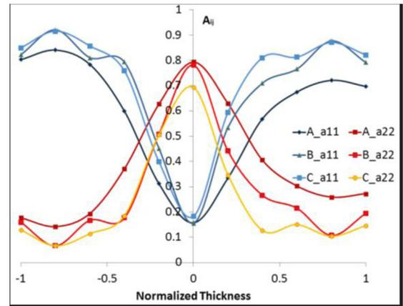
Figure 4. Fiber orientation tensor components A11 and A22 for 40% glass-PP center-gated sample with slow fill.
