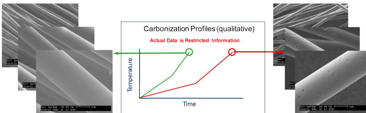
Figure 4. Influence of carbonization heating rate on structure of CF.
