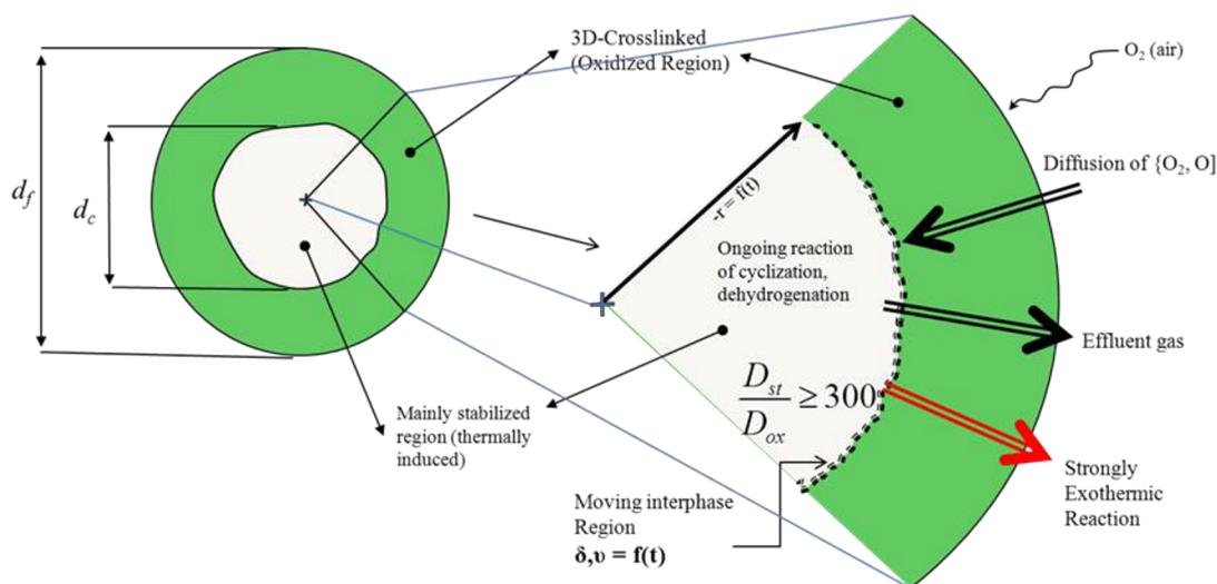
Figure 15. Single filament cross section during conventional oxidative stabilization process.
