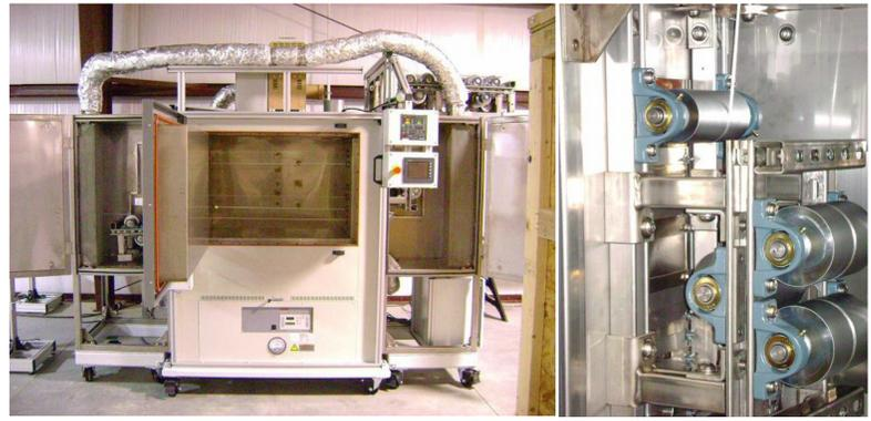
Figure 19. Oxidation oven with fully integrated tension controls, shown at right.
