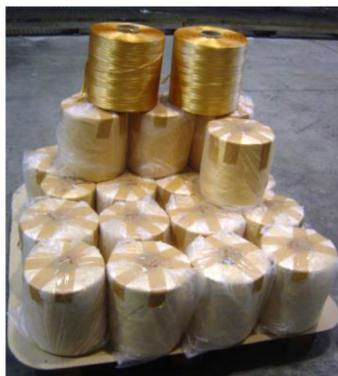
Figure 7. Textile tow precursor as produced by FISIFE and supplied to ORNL on spools for evaluation.
