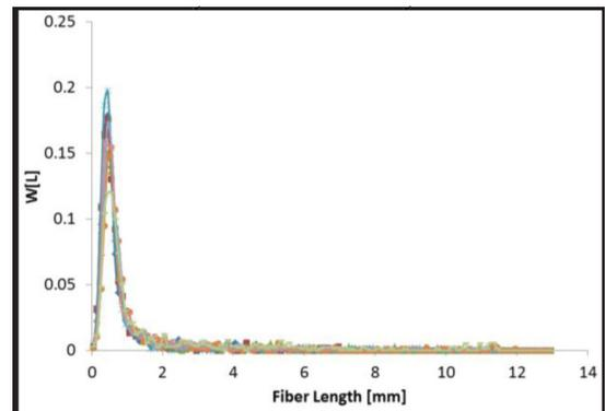
Figure 3. Fiber length distribution at location B for all samples.
