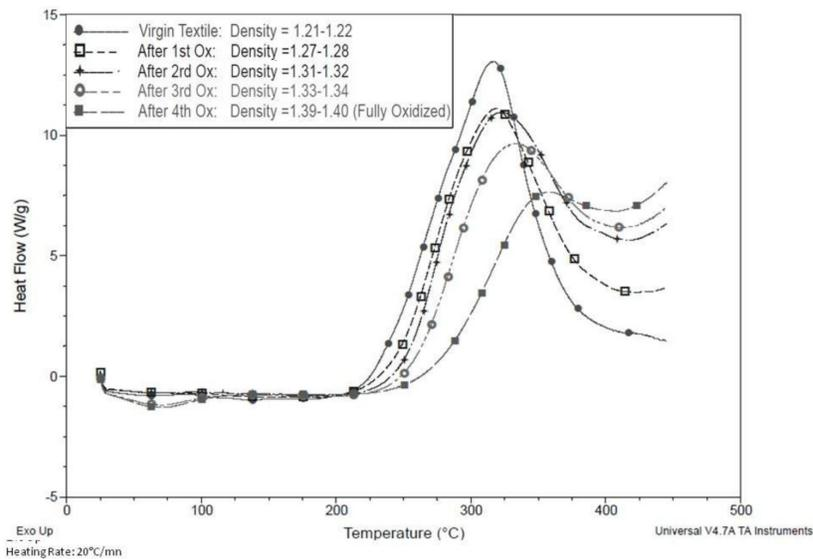
Figure 16. DSC plots of various stages of conventional oxidation for textile grade PAN. Density in grams per cubic centimeter for each stage is noted in the legend.
