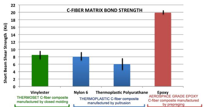
Figure 20. Comparison of relative interfacial bond strength of commercial epoxy sized CFs (C-fiber in the figure) with different resins using SBSS measurements. Industrial standard epoxy based sized CFs were used for all resins and processes.
