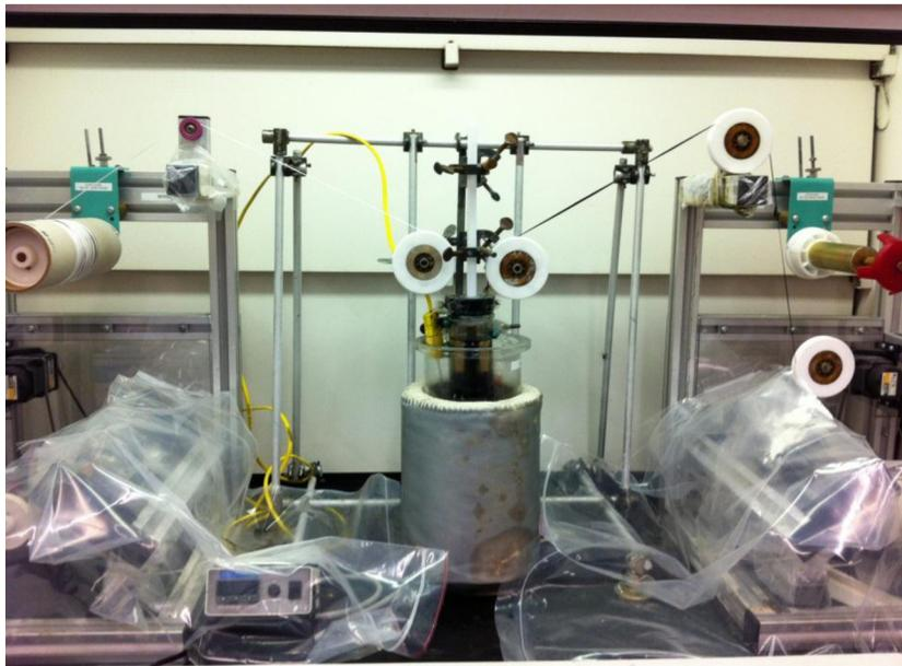
Figure 13. Continuous functionalization reactor assembly. White fiber is polyolefin fiber and black fiber exiting the reactor is functionalized polyolefin fiber.
