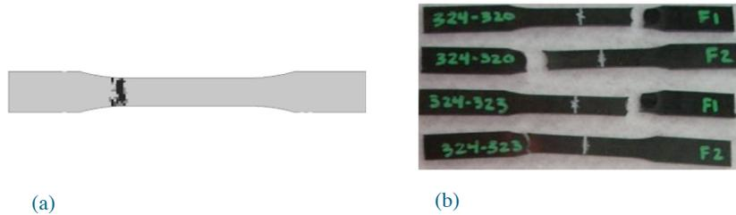
Figure 6. (a) Predicted failure and (b) experimental failure for the flow-direction specimens cut from the 40% glass-PP center-gated plaques
