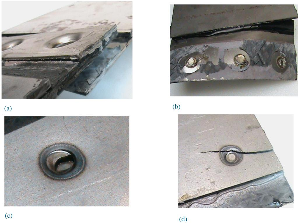
Figure 11. Cyclic torsion fatigue failures observed with composite-to-steel weld bonded joint specimens: (a) composite delamination, (b) combination delamination-adhesive failure, (c) spot weld, and (d) crack in the vicinity of a spot weld..
