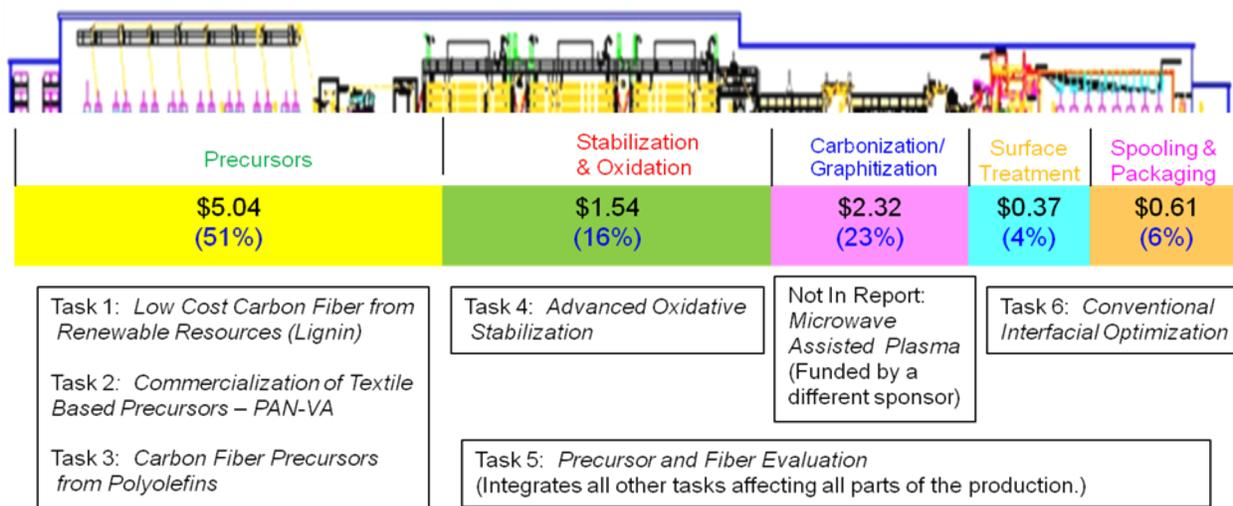
Figure 1. Role of LCCF development program tasks in the CF production process. (Base diagram courtesy of Harper International.)
