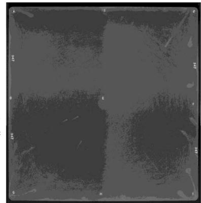
Figure 1. Center-gated sample from the first ACC molding trial exhibiting weld lines.
