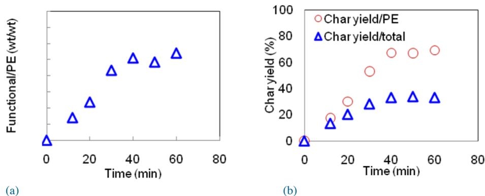
Figure 12. Functionalization of PE fibers in wt/wt basis (arbitrary scale) (a), and char yield data (b) as a function of reaction time at undisclosed conditions.
