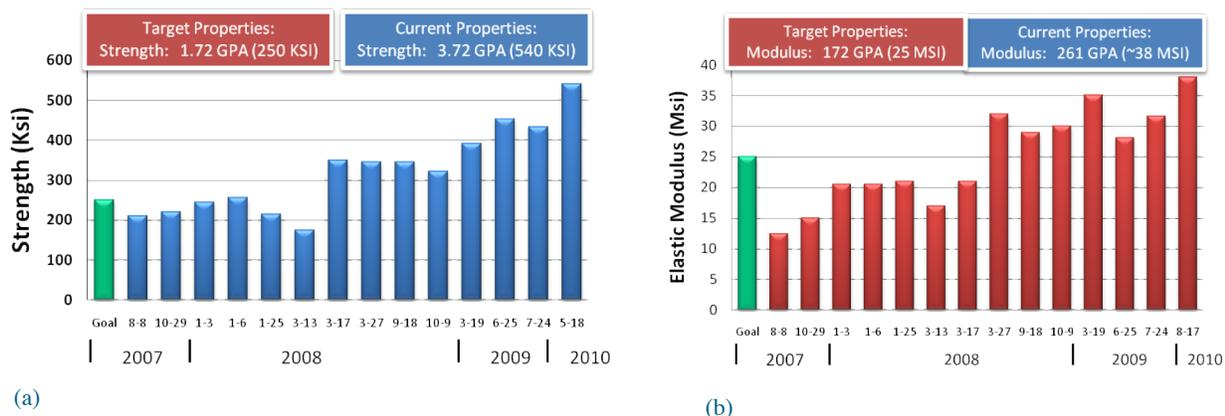
Figure 9. Strength (a) and modulus (b) data from FISIFE precursor converted and tested at ORNL showing substantial improvement trends.
