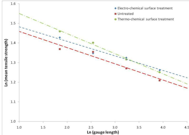
Figure 22. Determination of the Weibull modulus and the scaling parameter.
