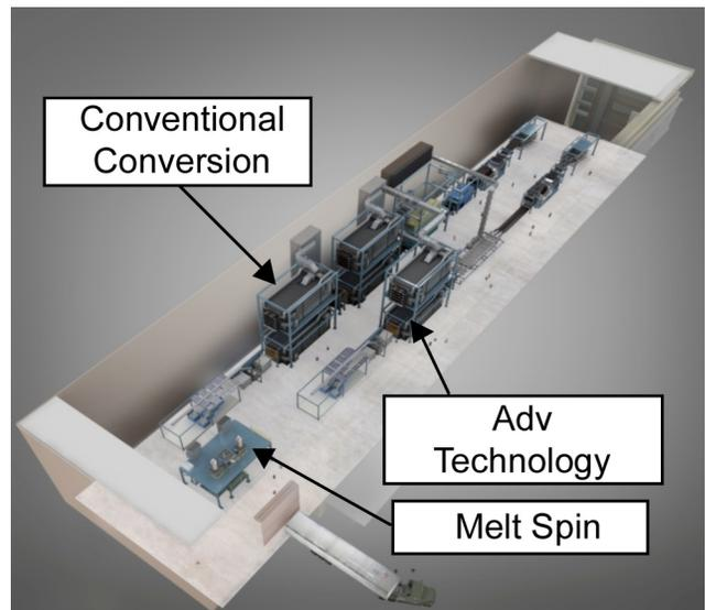
Figure 2. Schematic of the CFTF and equipment.
