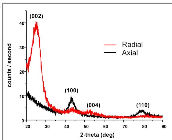
Figure 6. Axial and radial XRD patterns for PAN based CF.
