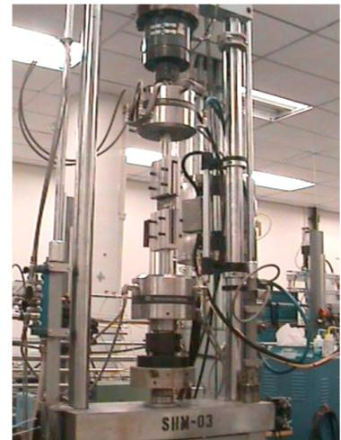
Figure 8. MTS axial-torsion test machine and test fixtures for torsional loading of composite-to-steel joint specimens.
