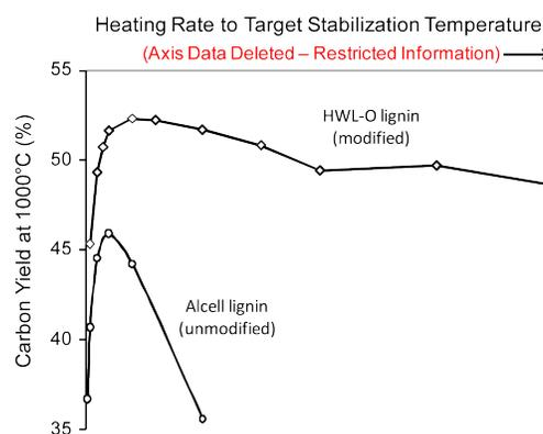
Figure 3. Carbon yield as a function of stabilization heating rate.
