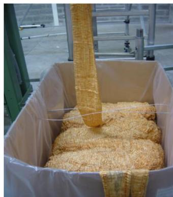
Figure 8. Textile tow precursor as produced by FISIFE and evaluated internally.
