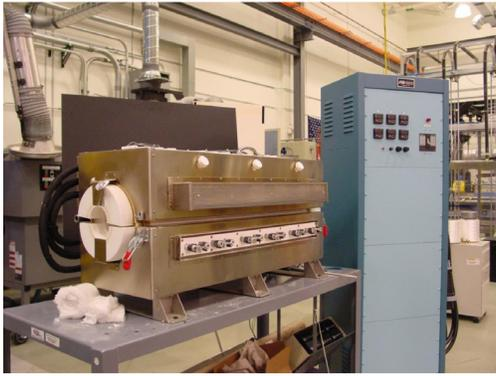
Figure 18. Three-zone high temperature carbonization furnace.
