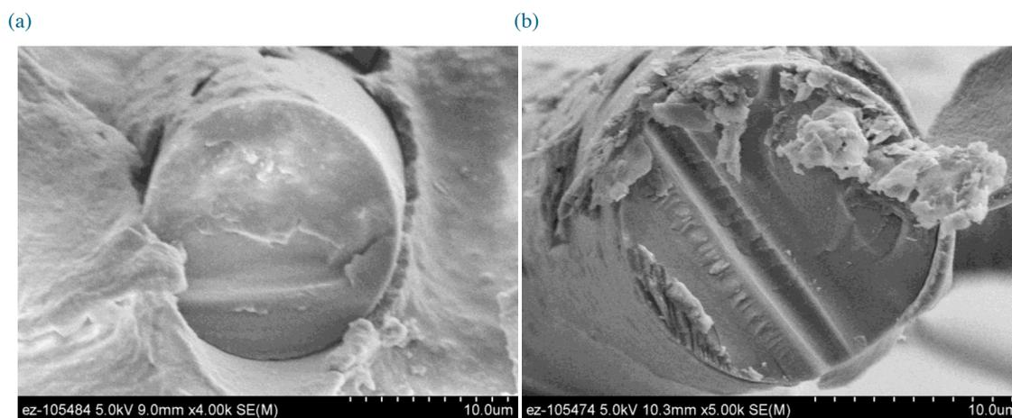
Figure 14. Scanning electron micrographs of fracture surfaces of CFs carbonized under (a) low and (b) high tension.
