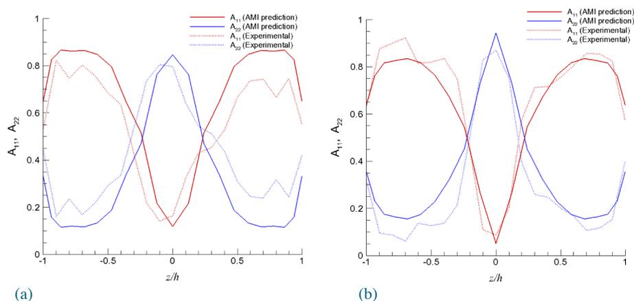
Figure 5. Comparisons of the experimental and predicted fiber orientation results for (a) the 40% slow-fill glass-PP center-gated plaque at location A, and (b) the 40% fast-fill glass-PA6,6 center-gated plaque at location B.
