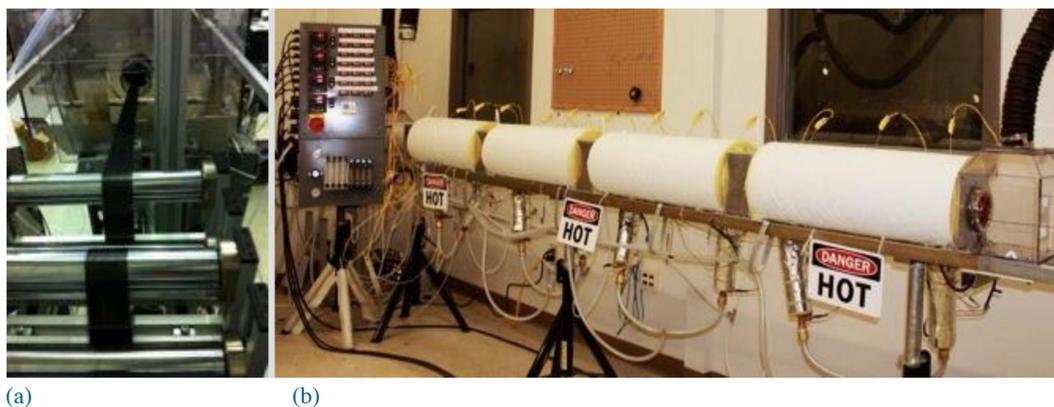
Figure 21. ORNL surface treatment system: (a) delivery of continuous 50,000 filament CF using spreading bars and (b) developed and scaled-up experimental ORNL thermochemical surface treatment applicator.
