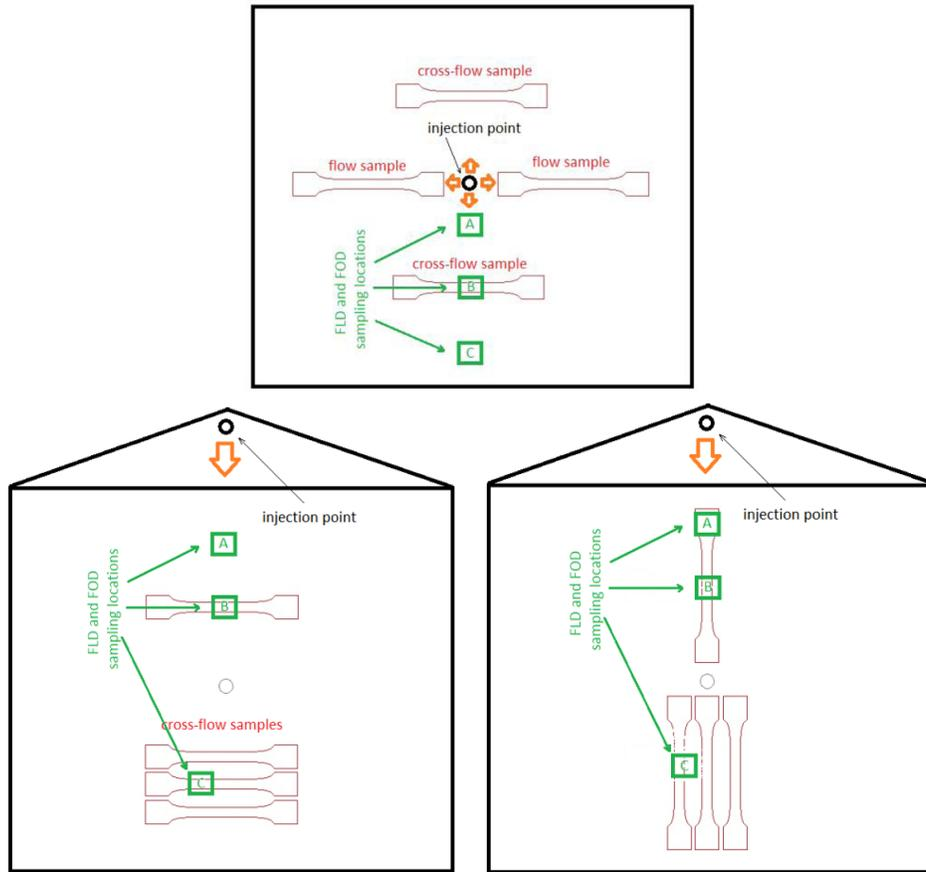
Figure 2. Sampling locations for center-gated plaques (top), and edge-gated plaques (bottom).
