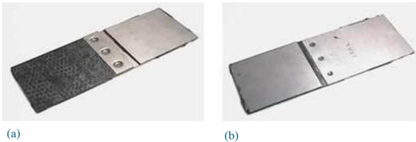
Figure 7. Composite-to-steel weld bonded joint specimen: (a) front and (b) back
