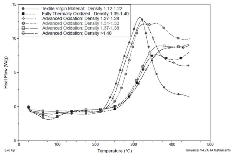
Figure 17. DSC plot comparison of conventional to advanced oxidized textile grade PAN fibers. Density in grams per cubic centimeter for each stage is noted in the legend. Note the advanced fiber with density 1.36–1.37 is considered an anomaly.
