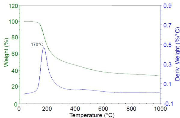
Figure 11. TGA of fully functionalized PE fiber.
