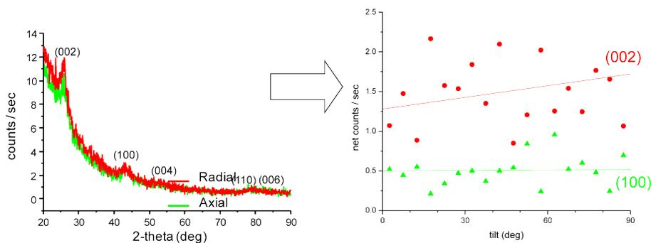
Figure 5. Axial and radial XRD patterns for lignin based CF.
