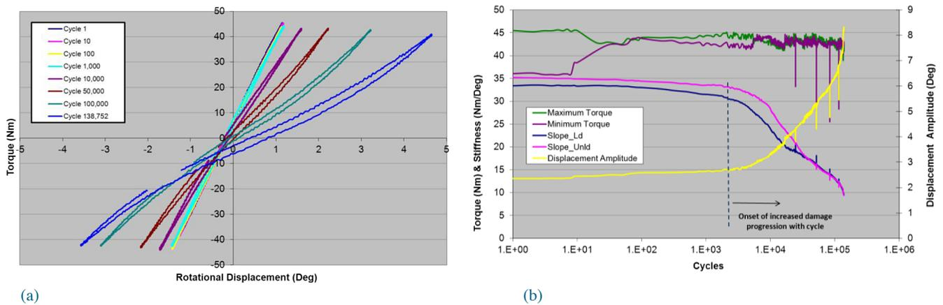
Figure 12. Cyclic torsion fatigue data collected for composite-to-steel weld bond specimen ( $\pm 42.4$  Nm, 1 Hz): (a) rotational displacement versus cycle and (b) torque, stiffness, and displacement amplitude versus cycle.
