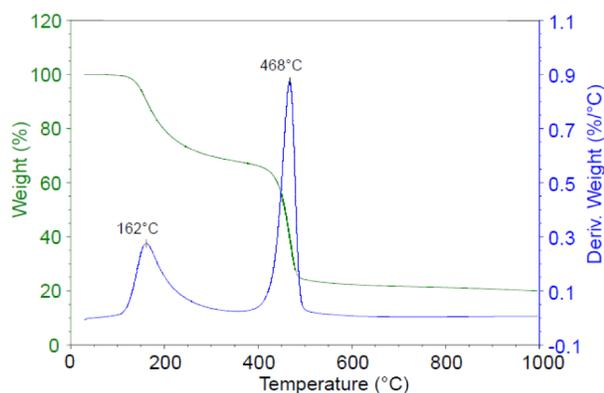
Figure 10. TGA of partially functionalized PE fiber.
