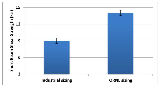
Figure 24. SBSS of CF-vinyl ester matrix composites made from industrial CF and ORNL sized CF.
