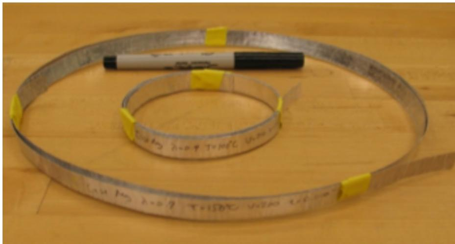
Figure 18. MgAZ31B strip produced directly from cast ingot by LSEM
