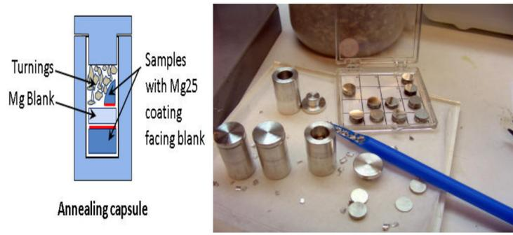
Figure 3. Diffusion annealing apparatus for Mg samples based on the Shewmon and Rhines technique (Shewmon and Rhines, 1954).
