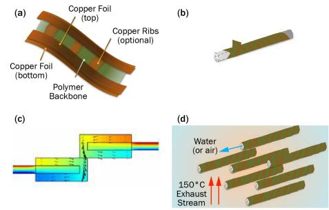
The proposed concept is a simple and modular heat exchanger formed from an array of tubes. (a) The tape that is used to construct the heat exchanger consists of a polymer backbone and copper-clad edges. (b) The heat exchanger tubes are manufactured by winding the metal-polymer tape and bonding the edges. (c) The overlapping copper edges enhance heat transfer. (d) Tubes are placed in the flue gas stack. *Photo credit University of Illinois.*
