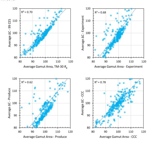
Figure 2. Average change in chroma (ΔC) versus average gamut area for the set of 344 light sources, using the four different sample/object sets. The outlier points are mostly highly structured SPDs (e.g., color mixed LEDs, HID) with low fidelity.
