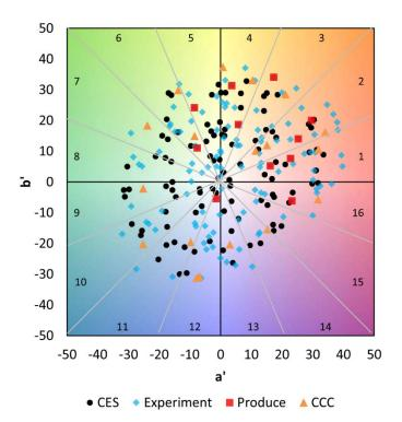
Figure 4. CAM02-UCS (a', b') coordinates of the samples in the four sets in the a'-b' plane of the CAM02-UCS. The coordinates were determined using 3500 K Planckian radiation, which was an arbitrary choice. The TM-30 hue angle bins and their corresponding numerical identifier are also shown.
