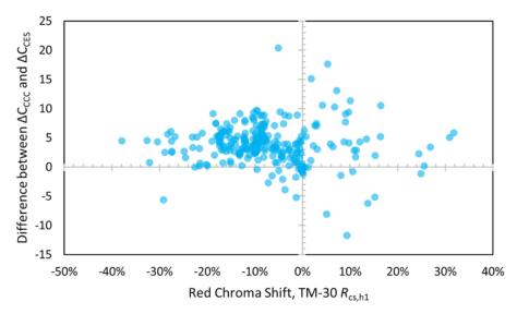
Figure 13.  $\Delta C$  versus TM-30  $R_{ch,h1}$  for the three object sets. There is a clear pattern for the experiment and produce sets, but not the CCC set.
