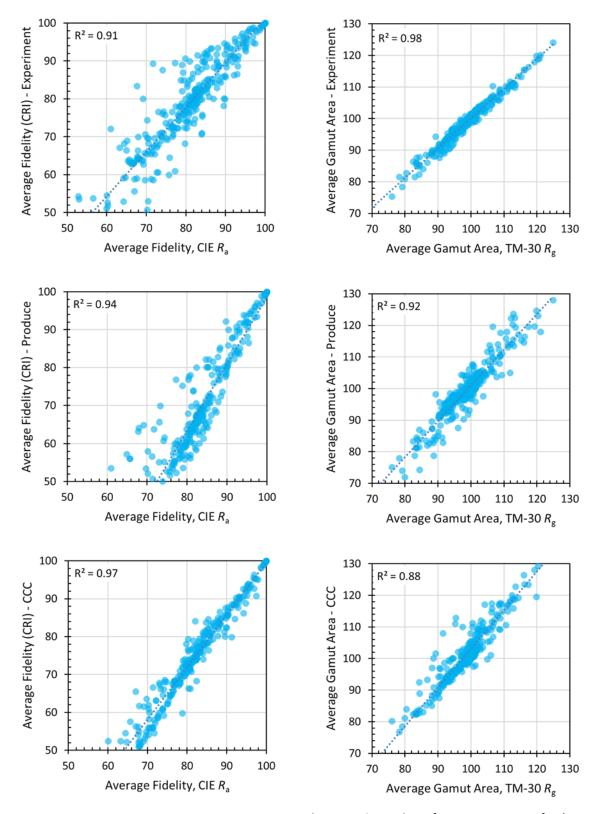
Figure 10. Comparison of average color fidelity for three object sets (using CIE  $R_a$  formulas) versus standard CIE  $R_a$  calculations. The correlation and magnitude of residuals is dependent on the spectral features and average chroma of the object sets.
