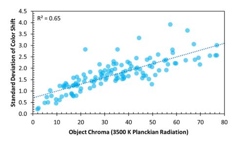
Figure 6. Average color shift (top) and standard deviation of color shift (bottom) for the experimental object set illuminated by the 26 SPDs used by Royer and colleagues [2016]. As object chroma increases, the chromaticity tents to be less stable from light source to light source.
