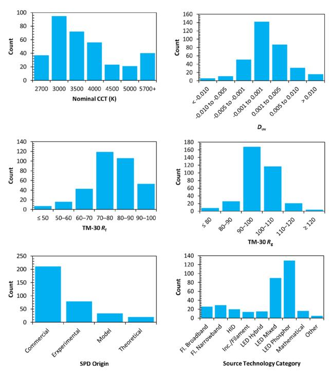
Figure 1. Characterization of the 344 sources comprising the dataset used in this evaluation.
