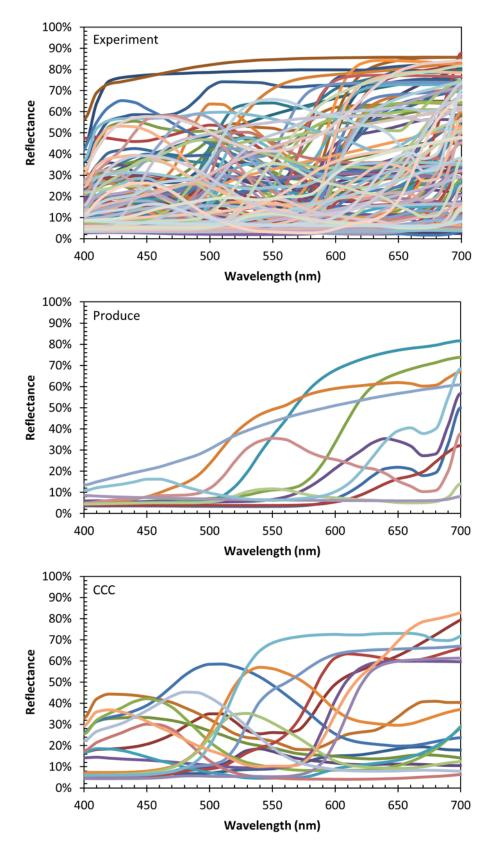
Figure 8. Spectral reflectance functions for the three non-TM-30 object sets included in this analysis.
