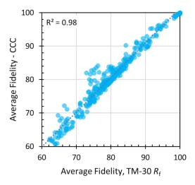
Figure 7. Comparison of average color fidelity for three object sets versus standard TM-30 average fidelity (R<sub>f</sub>) calculations. In this case, the scaling factor for each of the custom average color fidelity measures was adjusted using the same procedure that was used to calculate TM-30 R<sub>f</sub>. As such, the correlations are about 1:1 on average, but there is still variation due to features of the spectral reflectance functions.
