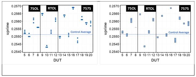
Figure A-2: The u' readings from the DUTs using TL-2 after 5,000 hrs of AST exposure. The actual readings are shown on the left, and the corresponding box plot is shown on the right. The average readings from the control samples are shown as the dotted blue line.
