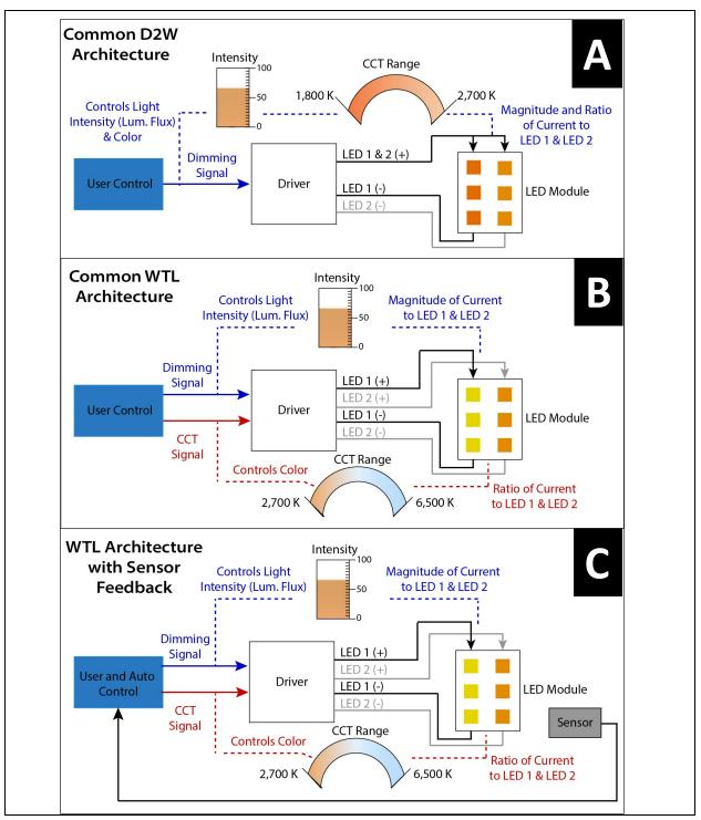
Figure 1-1: Common TLS system architectures. (A) Dim-to-warm systems, (B) standard WTL system, and (C) WTL systems with sensor feedback.
