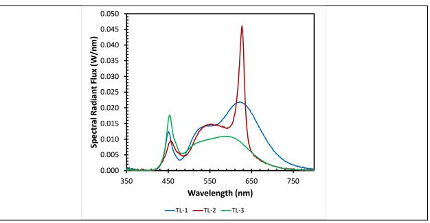
Figure 2-7: SPDs of the test lamps.
