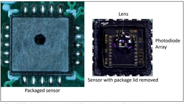
Figure 2-2: Packaged sensor on test board (left) and sensor elements after the package top was removed (right).
