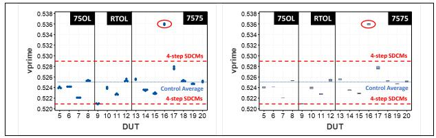
Figure 3-1: The  $\nu'$  readings from DUTs using TL-1 after 5,000 hrs of AST exposure. The actual readings are shown on the left, and the corresponding box plot is shown on the right. The average readings from the control samples are shown as the dotted blue line.
