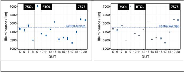
Figure A-5: Illuminance readings from the DUTs using TL-2 after 5,000 hrs of AST exposure. The actual readings are shown on the left, and the corresponding box plot is shown on the right. The average readings from the control samples are shown as the dotted blue line.
