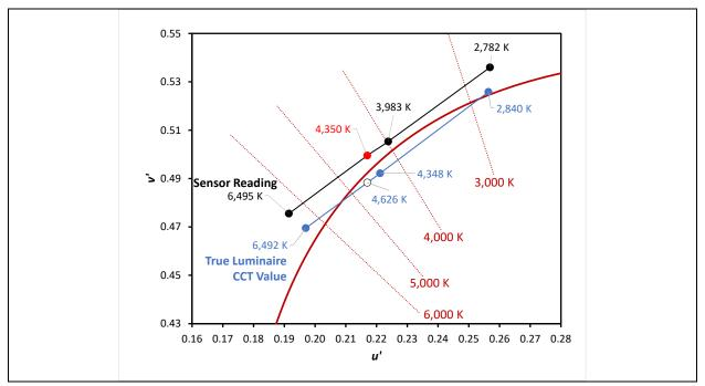
Figure 4-2: Potential impact of a faulty chromaticity sensor reading on CCT value of light from a TLS system. The blue dots and line represent the true luminaire values, and the black dots and line represent the readings from a faulty chromaticity sensor.
