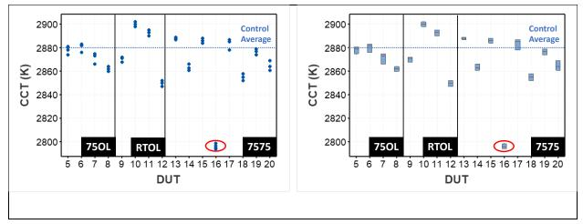
Figure 3-5: The CCT readings from the DUTs using TL-2 after 5,000 hrs of AST exposure. The actual readings are shown on the left, and the corresponding box plot is shown on the right. The average readings from the control samples are shown as the dotted blue line.
