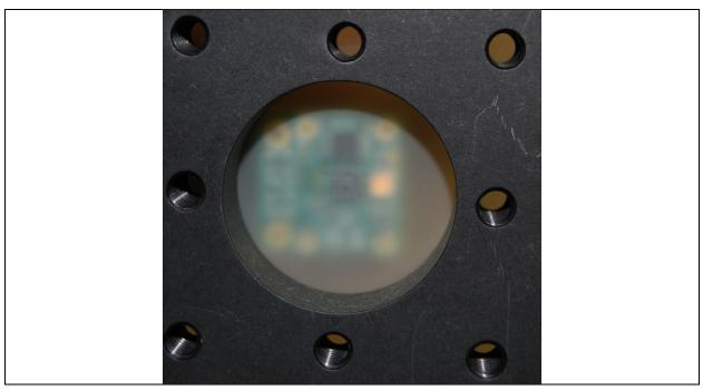
Figure 2-6: The optical diffuser film is positioned to just touch the surface of the sensor element.
