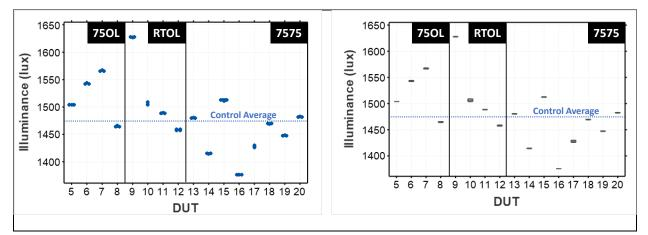
Figure A-4. Illuminance readings from the DUTs using TL-1 after 5,000 hrs of AST exposure. The actual readings are shown on the left, and the corresponding box plot is shown on the right. The average readings from the control samples are shown as the dotted blue line.
