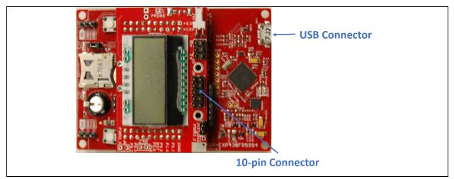
Figure 2-4: Reader board used to test the DUTs.
