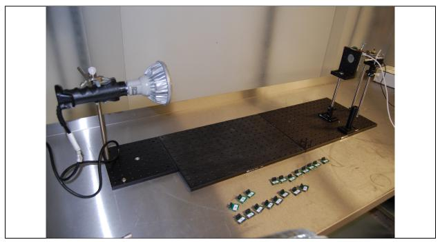
Figure 2-5: Experimental arrangement used to measure the sensor DUTs after AST exposure.
