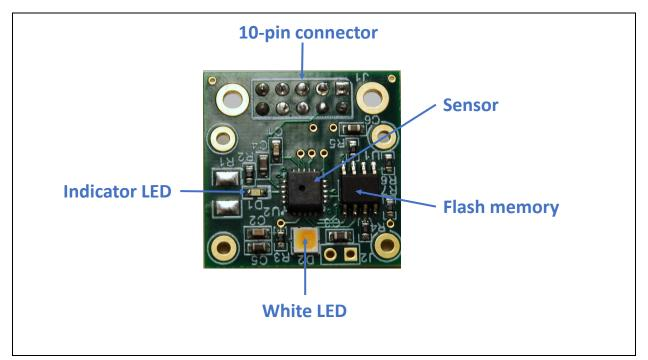
Figure 2-3: Sensor test boards used during this study.
