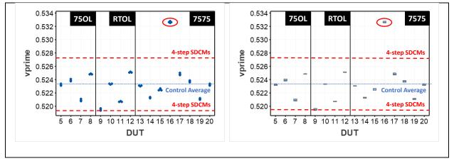
Figure 3-2: The  $\nu'$  readings from DUTs using TL-2 after 5,000 hrs of AST exposure. The actual readings are shown on the left, and the corresponding box plot is shown on the right. The average readings from the control samples are shown as the dotted blue line.
