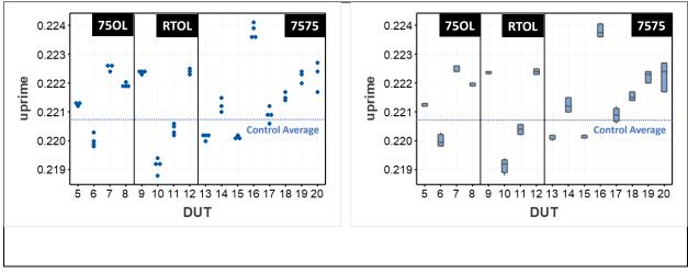
Figure A-3: The *u*'readings from the DUTs using TL-3 after 5,000 hrs of AST exposure. The actual readings are shown on the left, and the corresponding box plot is shown on the right. The average readings from the control samples are shown as the dotted blue line.
