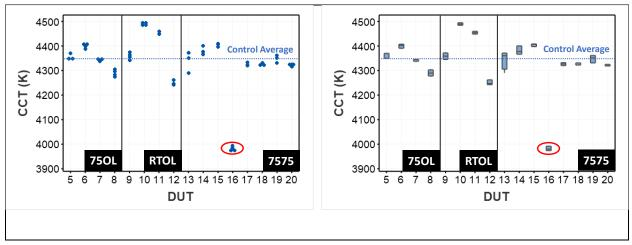
Figure 3-6: The CCT readings from the DUTs using TL-3 after 5,000 hrs of AST exposure. The actual readings are shown on the left, and the corresponding box plot is shown on the right. The average readings from the control samples are shown as the dotted blue line.
