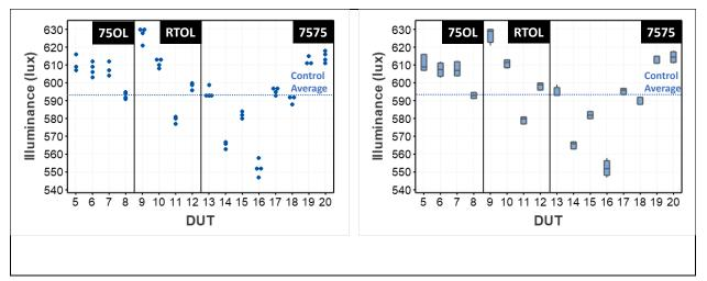
Figure A-6: Illuminance readings from the DUTs using TL-3 after 5,000 hrs of AST exposure. The actual readings are shown on the left, and the corresponding box plot is shown on the right. The average readings from the control samples are shown as the dotted blue line.
