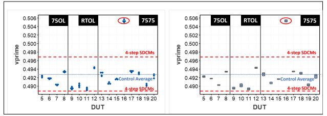
Figure 3-3: The  $\nu'$  readings from DUTs using TL-3 after 5,000 hrs of AST exposure. The actual readings are shown on the left, and the corresponding box plot is shown on the right. The average readings from the control samples are shown as the dotted blue line.
