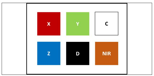
Figure 2-1: Arrangement of the photodiodes and inorganic interference filters in the DUTs.
