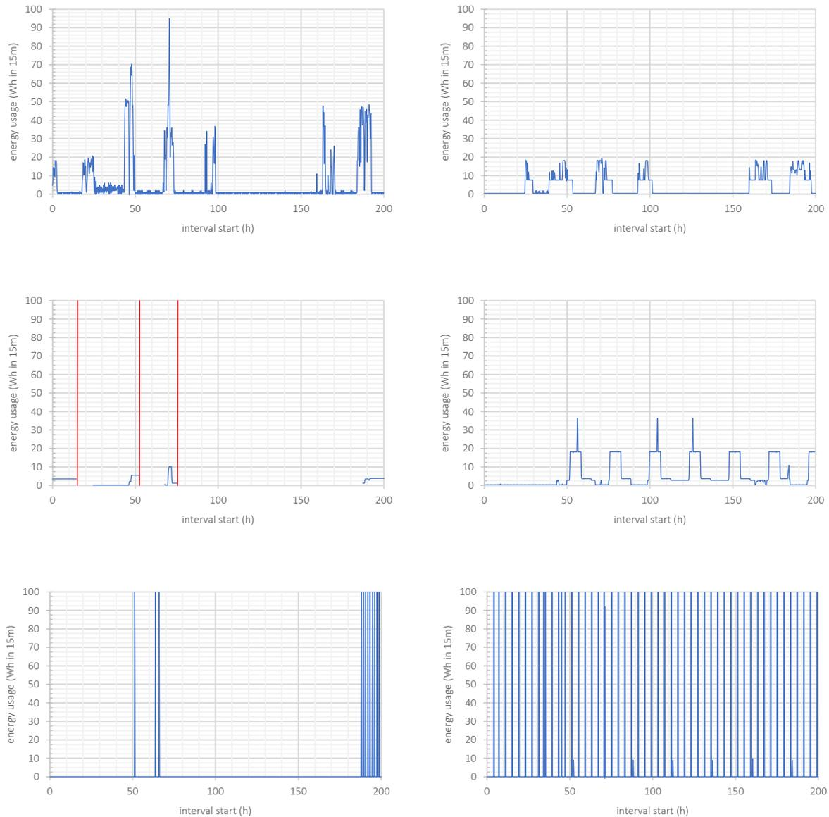
**Figure 4.1.** Energy usage per 15-minute interval for each of the six CLS over a period of 200 hours. Red vertical lines indicate a 15-minute-interval data point that was not reported due to network or other issues.
