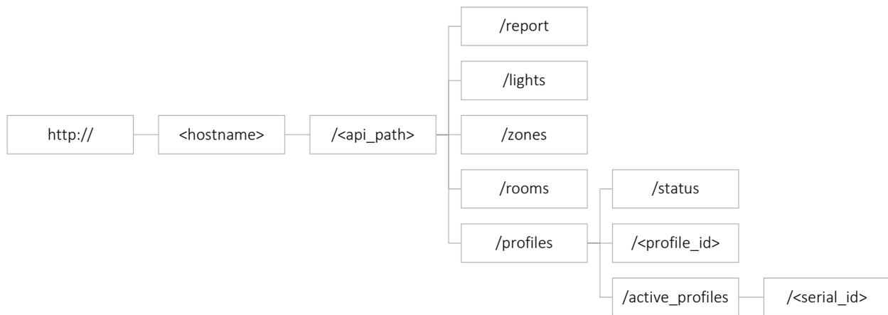
**Figure 3.1.** Connected lighting system API resource tree, example 1
