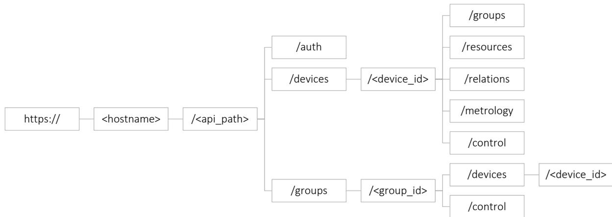
**Figure 3.2.** Connected lighting system API resource tree, example 2
