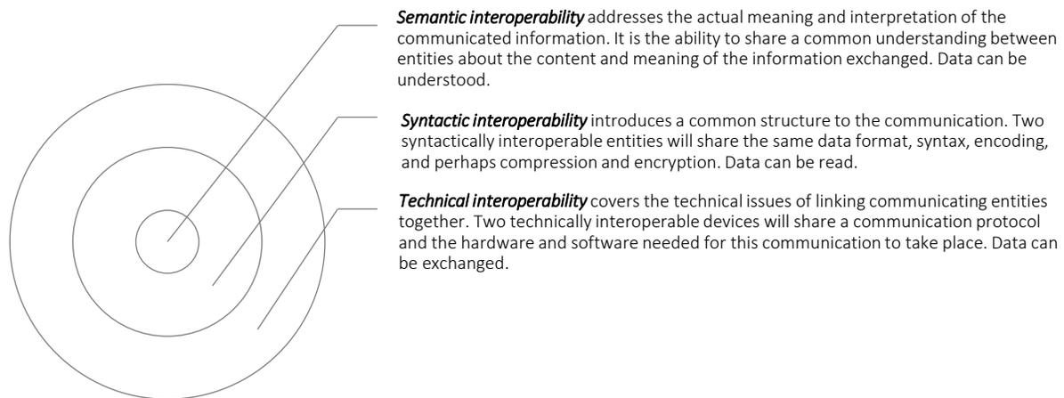
**Figure 2.1.** Three conceptual layers of communication-system interoperability
