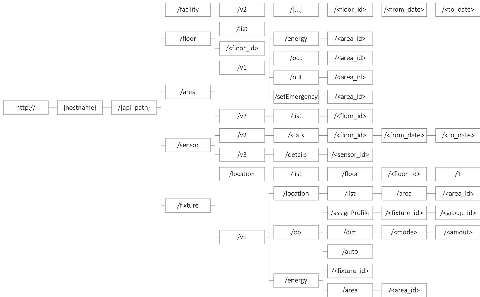
**Figure 3.3.** Connected lighting system API resource tree, example 3
