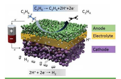
Depiction of the proposed electrochemical cell in the low-temperature production of ethylene and hydrogen from ethane. *Graphic image courtesy of Idaho National Laboratory*
