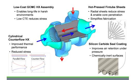
Overview of the key components and their potential benefits for the glass ceramic-matrix composite (GCMC) heat exchanger (HX) concept. *Graphic image courtesy of United Technologies Research Center (UTRC)*
