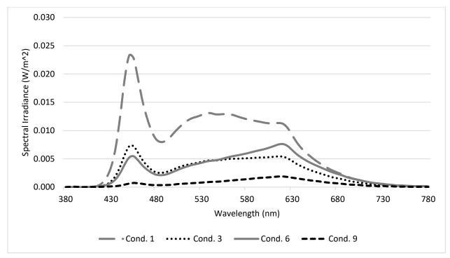
Figure 5. Plot of the spectral power distribution measured at the patient eye position when laying slightly upright in bed for lighting conditions 1, 3, 6, and 9.
